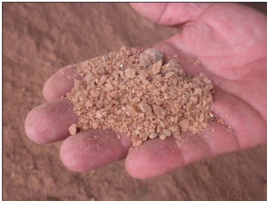
FIG 14. MeltDown® 20 is a granular de-icing chemical distributed to TxDOT by Envirotx
