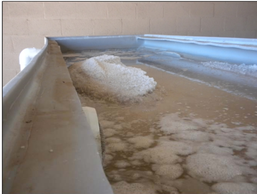
FIG 17. The TxDOT Childress District invested in a salt brine manufacturing tank system to make their own salt brine
