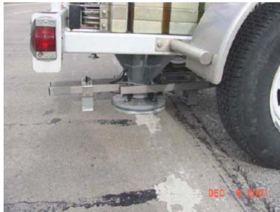
**Figure 2. 34 Deflection Testing at Pavement Edge With Asphalt Shoulder**
