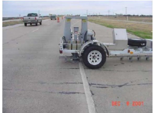
**Figure 2. 33 Deflection Testing at Pavement Edge With Tied Concrete Shoulder**
