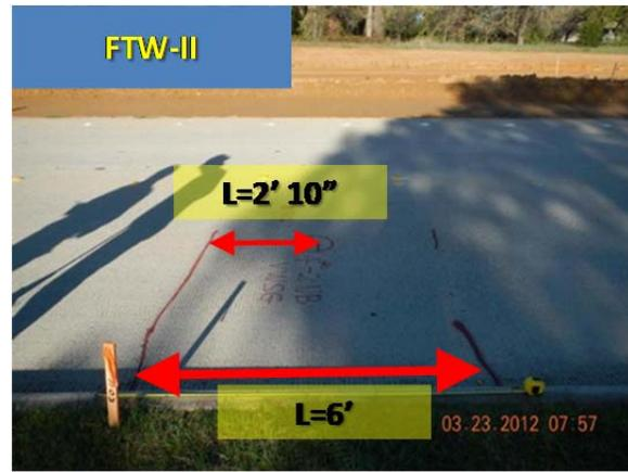
Figure 4. 63 Crack Location at FTW-II Test Section
