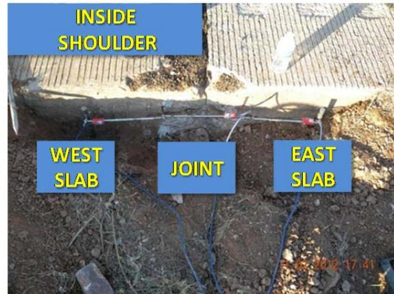
Figure 4. 25 Crackmeter Installation at Inside Shoulder – Childress Test Section
