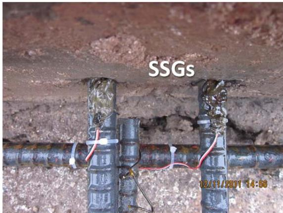
**Figure 3. 9 Steel Strain Gage Installation at LBB-I Test Section**
