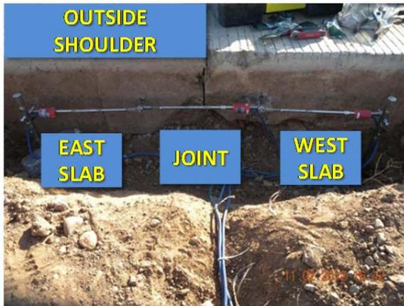
Figure 4. 24 Crackmeter Installation at Outside Shoulder – Childress Test Section
