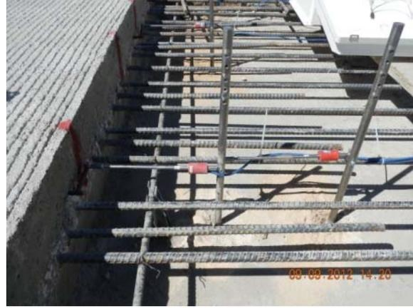
**Figure 3. 50 Reference Crackmeter Attached to Measure Invar Movement at BWD-II Test Section**
