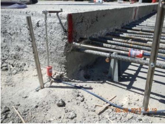
**Figure 3. 49 Vertical Crackmeter Installed at the Free Slab Edge at BWD-II Test Section**
