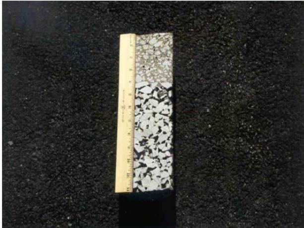
**Figure 2. 43 Cross-Section of Cement Stabilized Drainable Base (Photo Courtesy of M. Mueller)**
