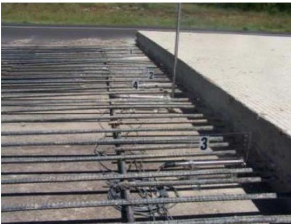
**Figure 2. 10 Slab Movement Experimentation (Nam, 2005)**
