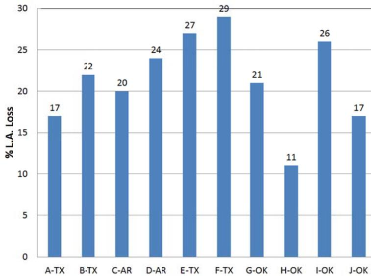
**Figure 3.1 L.A. Abrasion Loss for Aggregates**
