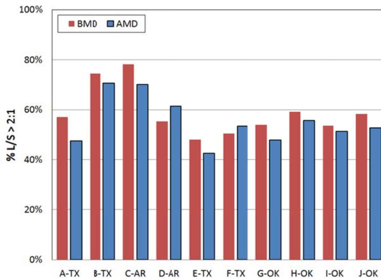
**Figure 3.12 Particle Shape Before and After Micro-Deval**
