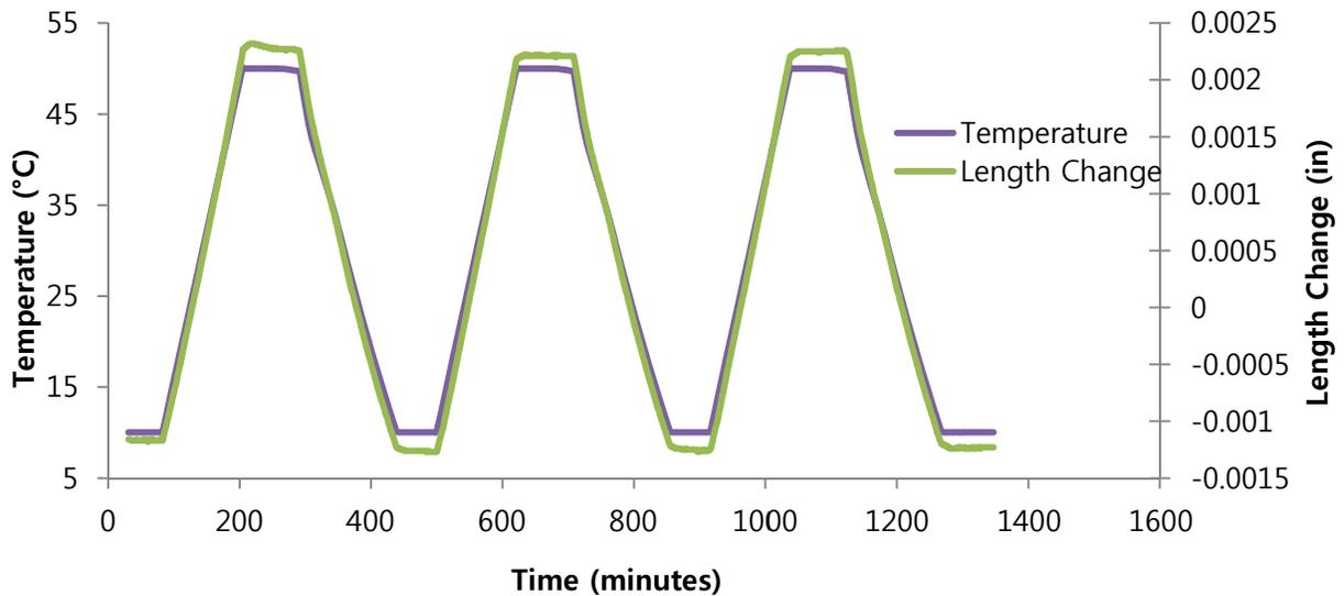
**Figure 3.21 Three Cycles of Heating and Cooling and Change in Length for 4-in. x 7-in. Concrete Cylinder of B-TX**
