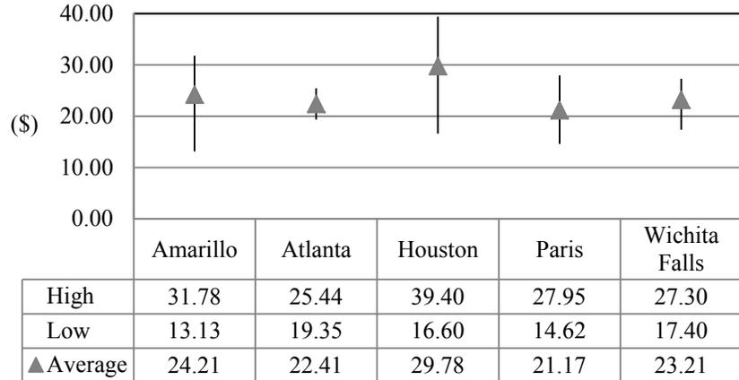
**Figure 4.2 Total Cost of Coarse Aggregate Including Delivery Per Ton**
