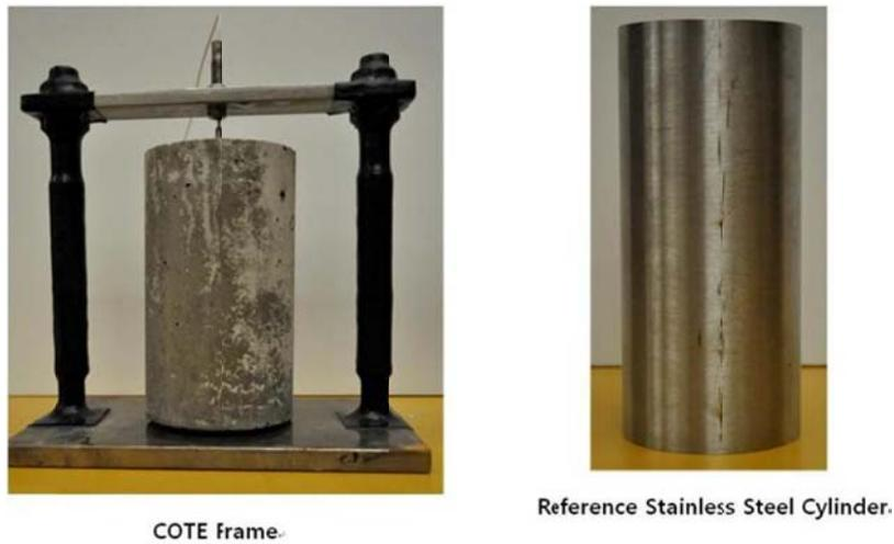
**Figure 3.20 CoTE Frame and Reference Stainless Steel Cylinder**
