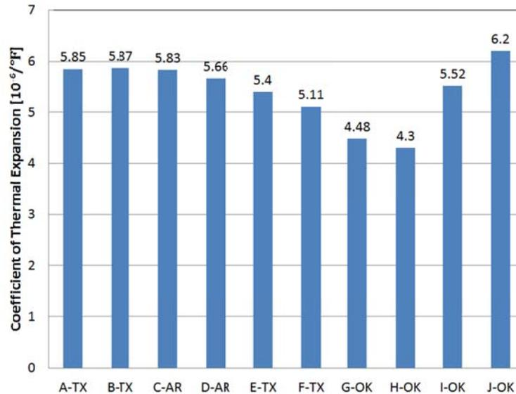
**Figure 3.22 CoTE for Concrete Specimens Older than 28 Days**
