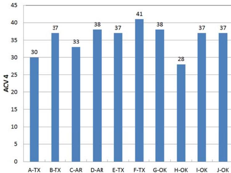
**Figure 3.14 Aggregate Crushing Value**
