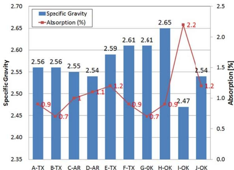
**Figure 3.3 Specific Gravity and Absorption of Aggregates**
