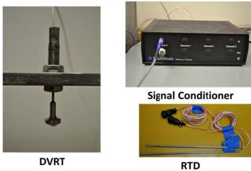
**Figure 3.18 Various Components of CoTE Setup**
