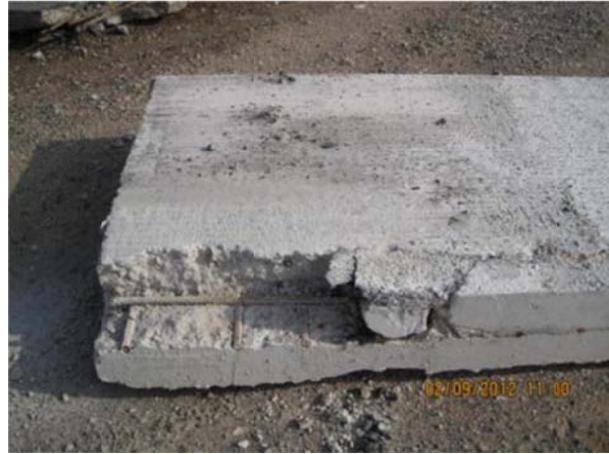
**(b) Transverse Steel above Longitudinal Steel**
