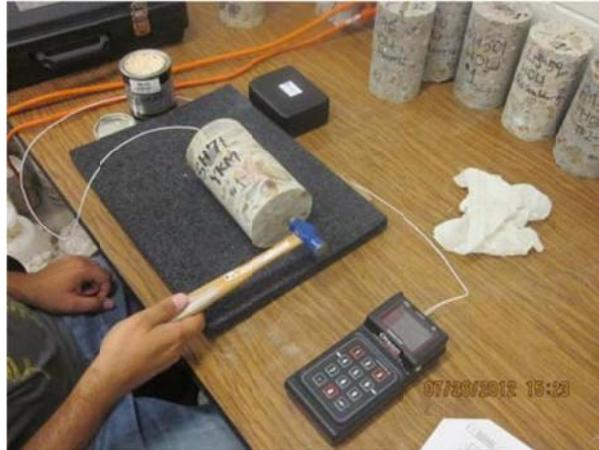
**Figure 2.21 Resonant Frequency Test**
