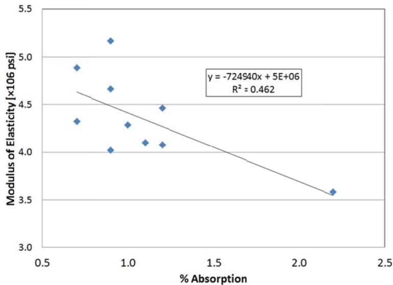
**Figure 3.17 Comparison of 28-day Modulus of Elasticity of Concrete and % Absorption of Aggregate**
