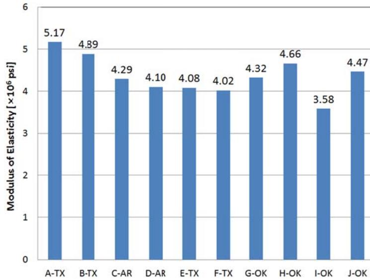
**Figure 3.16 Modulus of Elasticity for Concrete Specimens at 28 Days of Age**
