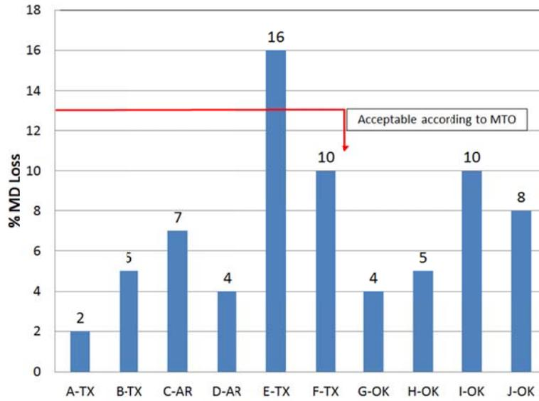
**Figure 3.4 Micro-Deval Loss for Aggregates**
