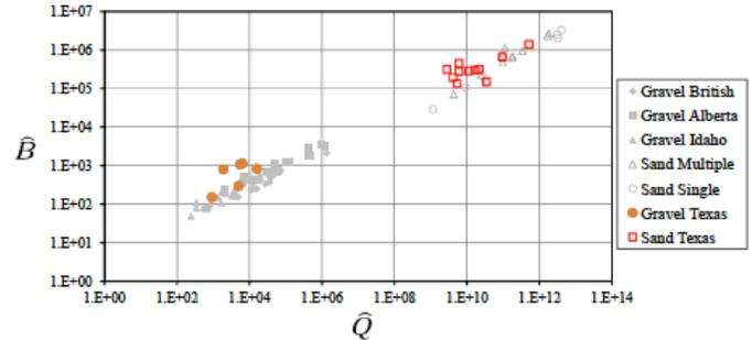
Figure 2. Dimensionless Discharge and Topwidth for Texas Streams.
