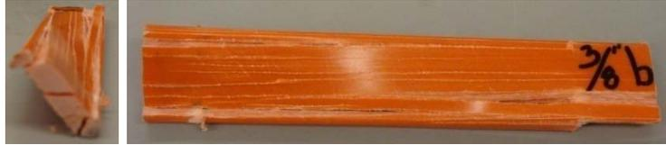
Figure 3.17 Failure of Specimens Subjected to Torsion
