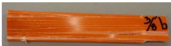
(c) Laboratory specimen failed due to torsion
