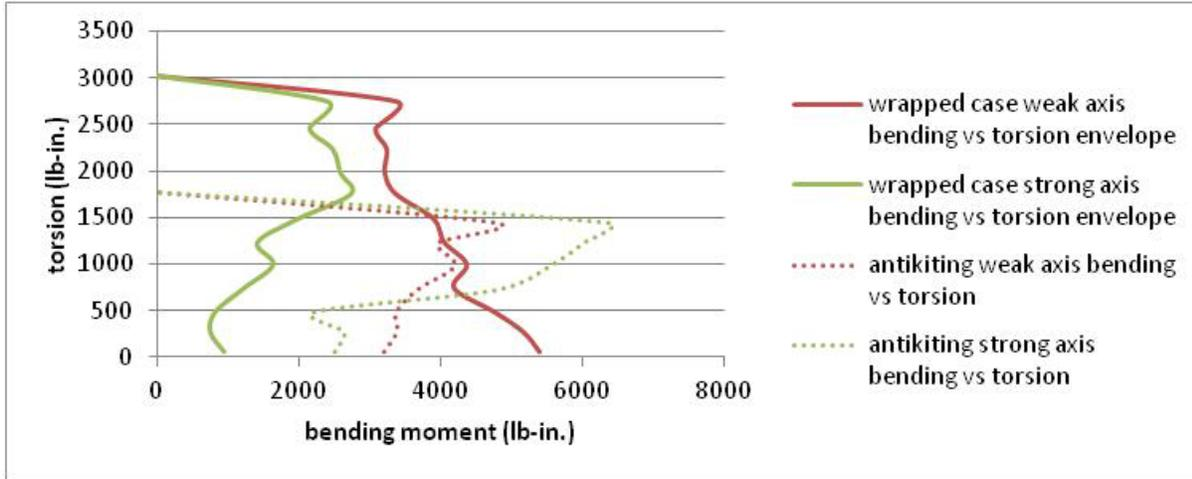
Figure 4.10 Torsion-Bending Moment Interaction of Steel Frame Signs
