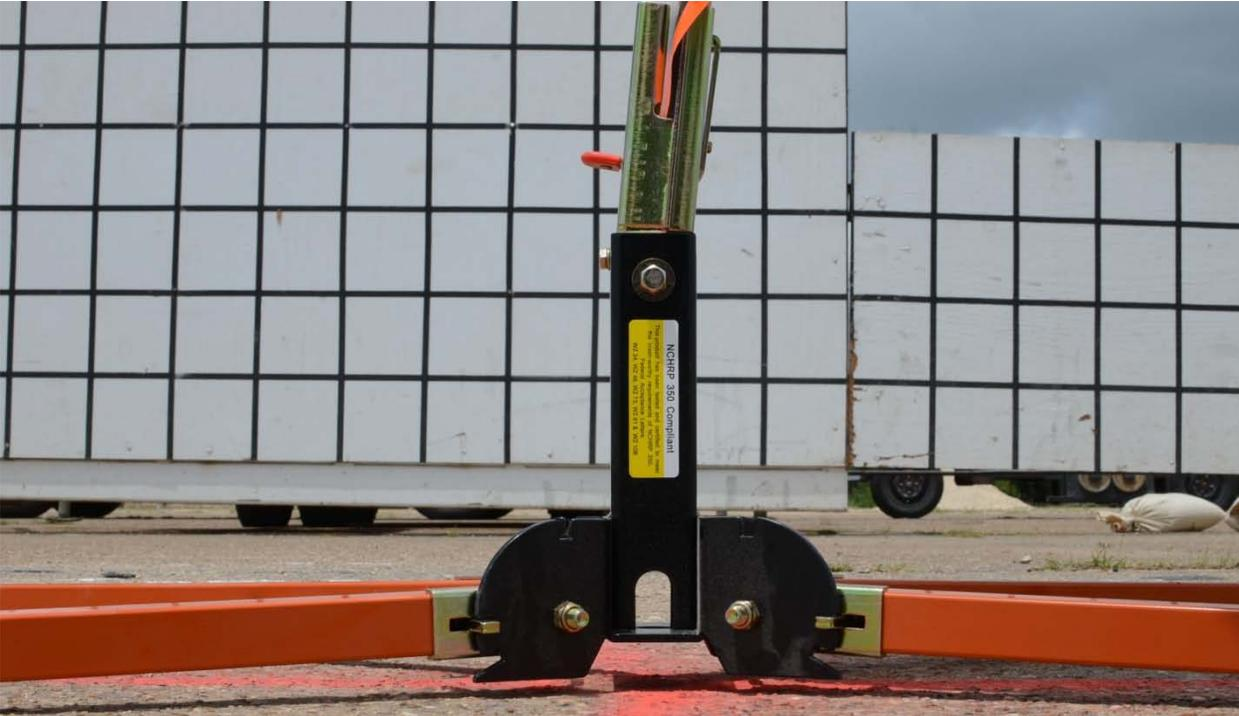
Figure 6.13 Type 1 Test Sign with a Spring Loaded Universal, Snap-in Bracket
