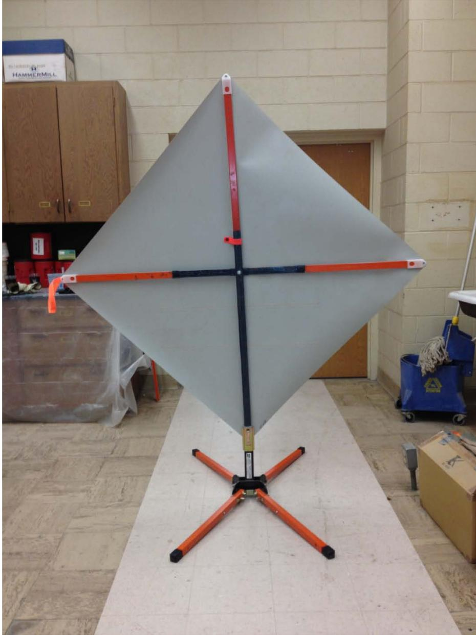
Figure 5.3 Photos of a Sign Fabricated with the Proposed Vertical and Horizontal Frames
