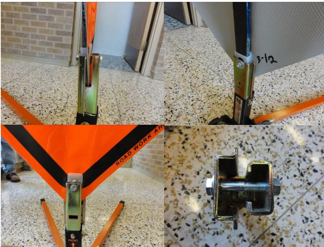
Figure 3. Photos of the fabricated prototype through-bolt connection used for a crashworthiness test specimen
