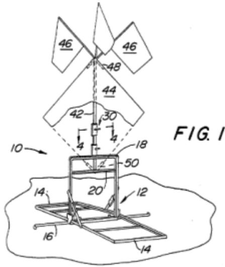
Figure 2.1 Early Brace Design of the Roll-up Sign (Left: U.S. Patent 4280853, Right: U.S. Patent 4309836)
