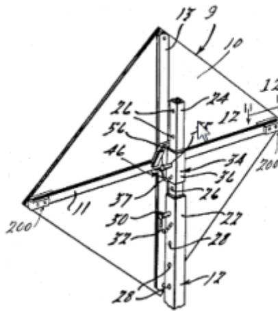
Figure 2.2 Brace Design of the Roll-up Sign (Left: U.S. Patent 4490934, Right: U.S. Patent 4548379)
