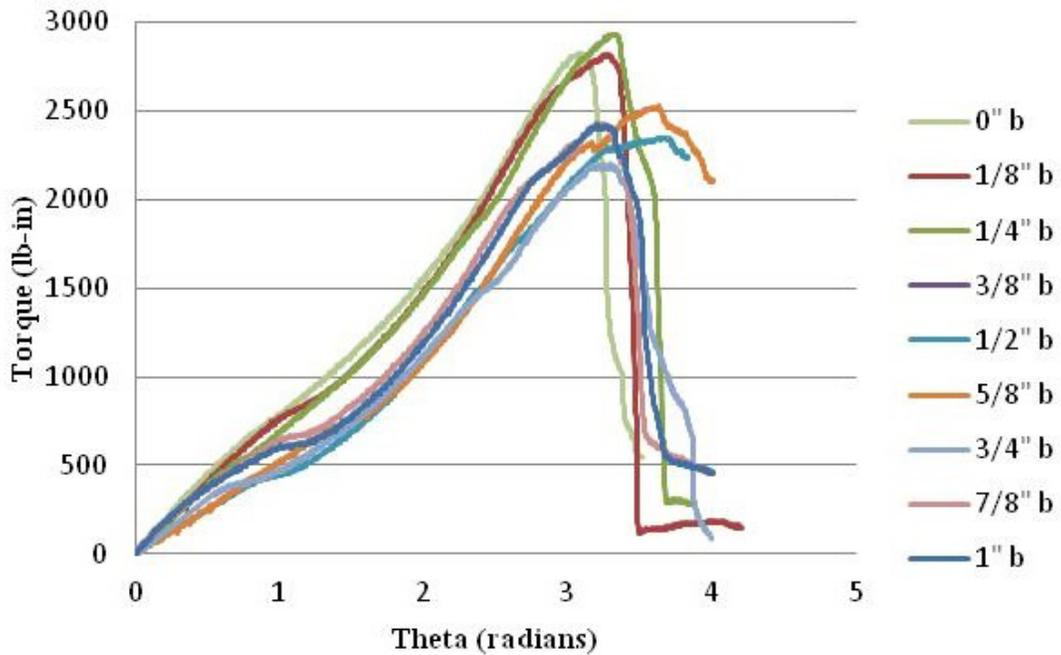
Figure 6.2 Torsion Test Results - Fiberglass Frames Reinforced with Carbon Fiber Sheets
