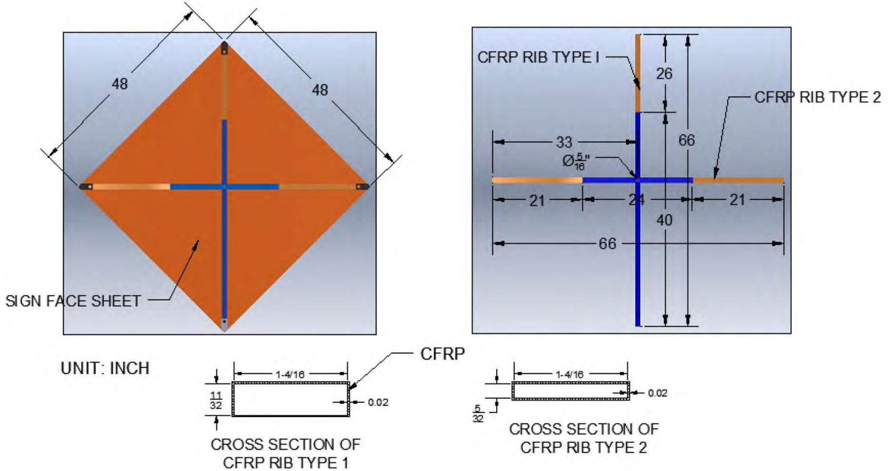
Figure 2.2. Dimensional Details of the Portable Roll-Up Sign Panel and Supports.
