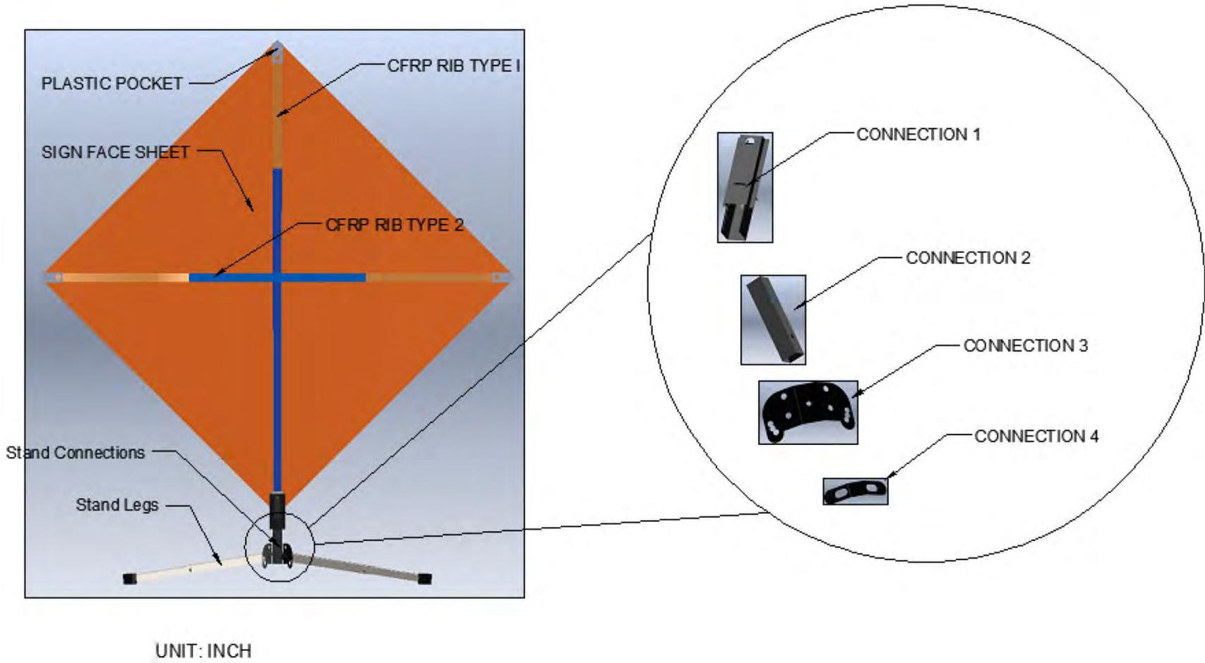
Figure 2.1. Components of the Portable Roll-Up Sign.
