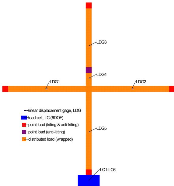
Figure 3.19 Instrumentation
