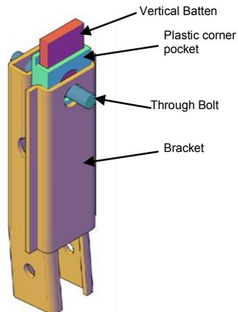
Figure 2. Schematic design representation of the prototype through-bolt connection used for fabricating the proposed roll-up sign design
