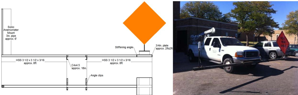
Figure 3.27 Truck Instrumented with a Sign Assembly and Sonic Anemometer
