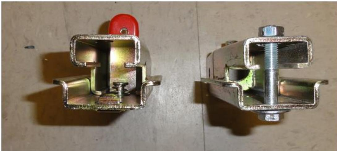
Figure 1. Spring-loaded universal, snap-in, pocket-type roll-up sign receiver bracket (Left) and the prototype through-bolt bracket
