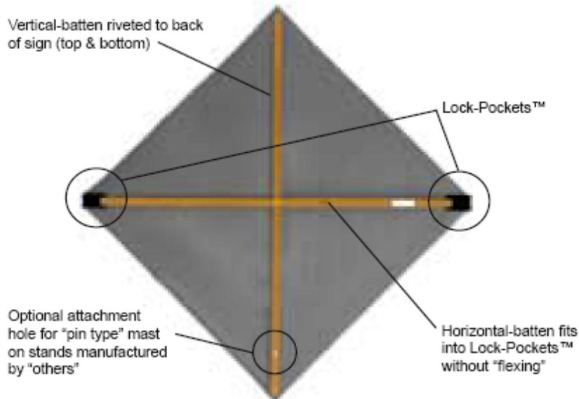
Figure 2.4 Braces of Roll-Up Sign (USA-Sign, 2007)
