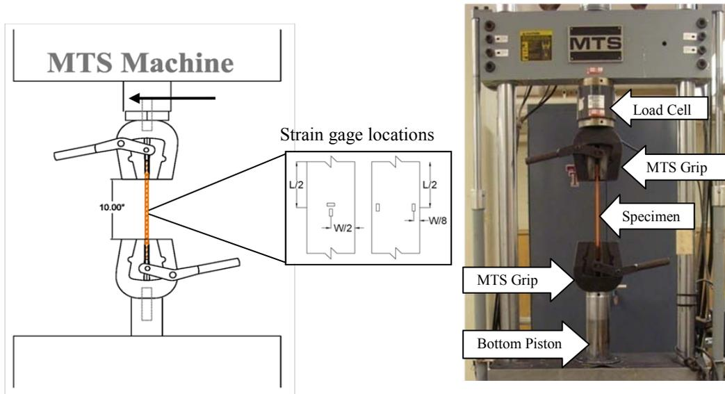
Figure 3.2 Tension Test Set-Up
