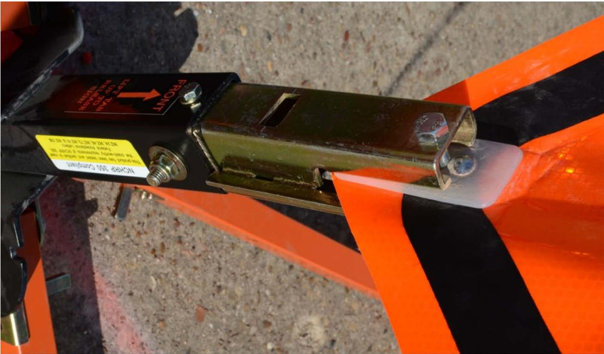
Figure 6.14 Type 2 Test Sign with a Through-Bolt Bracket
