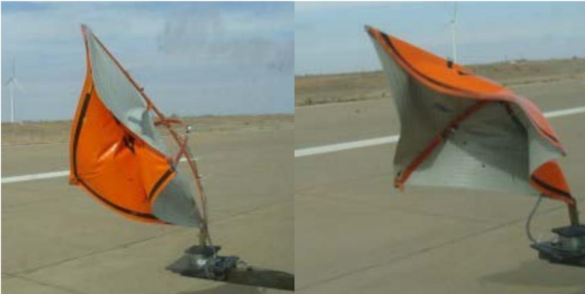
Figure 3.21 Examples of Anti-Kiting and Wrapped Cases
