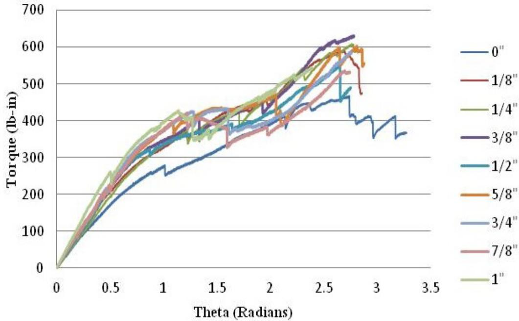
Figure 6.1 Torsion Test Results - Fiberglass Frames
