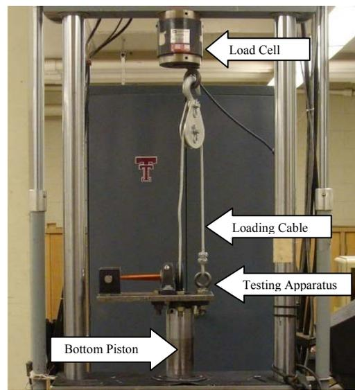
Figure 3.6 Close up of Torsion Test Supporting Plate Design and Actual Torsion Test Set-Up
