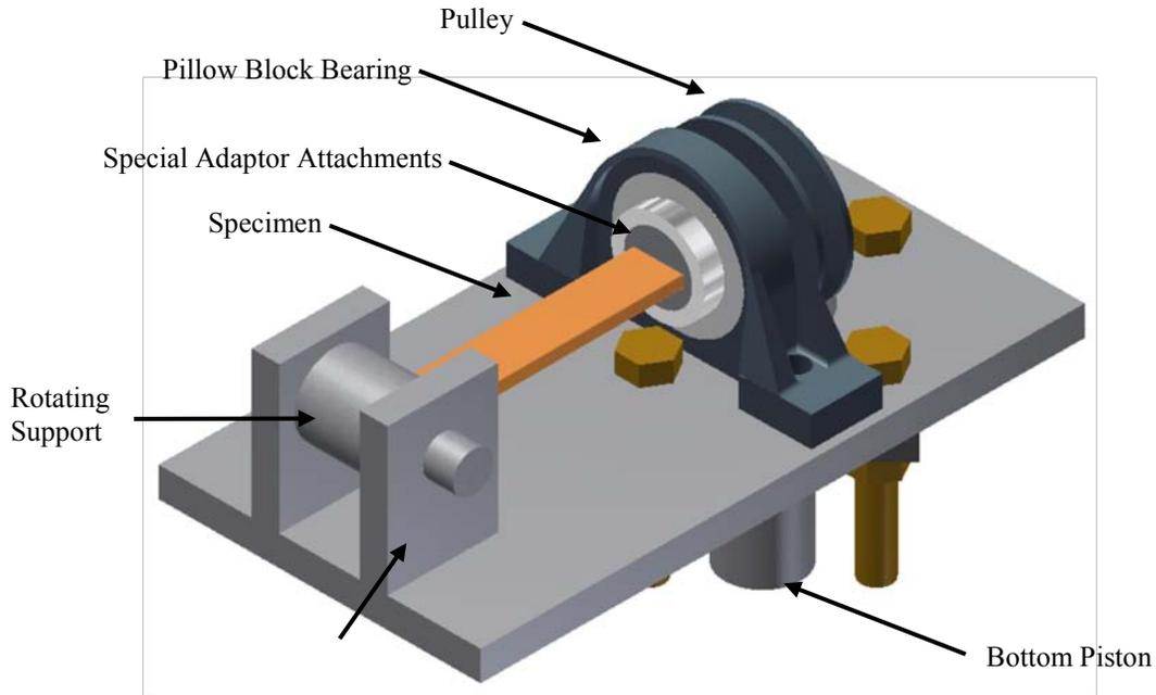
Figure 3.5 Prototype of Torsion Testing Apparatus
