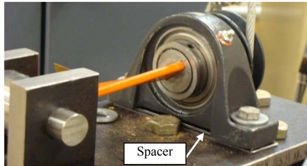
Figure 3.7 Combined Torsion and Bending Test Showing the Spacers Added.
