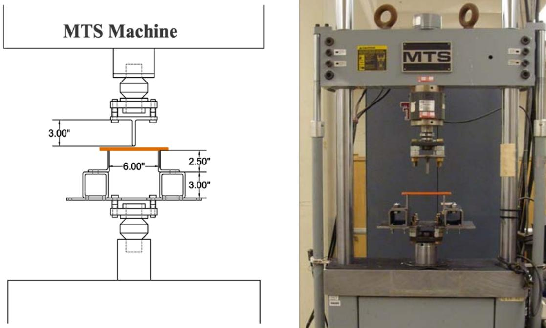
Figure 3.4 Bending Test Set-Up
