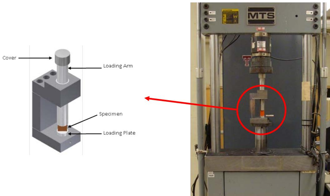
Figure 3.3 Compression Test Set-Up
