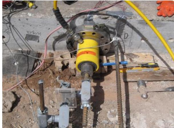
Figure 3.2- (l) Install LVDT
