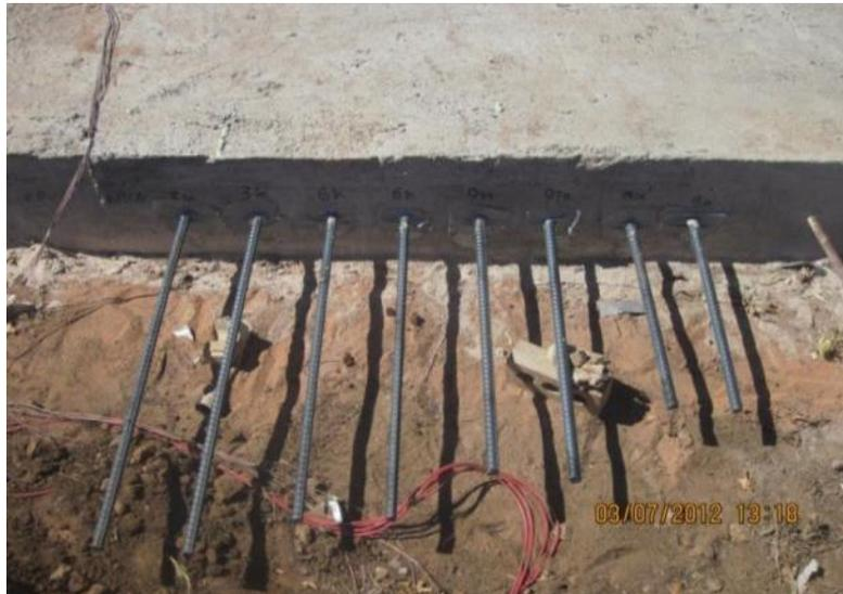
Figure 3.4- (a) Tie bars of different embedment length
