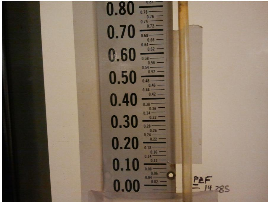
Figure 28: Sight Glass Used to Measure Head in the Head Tank
