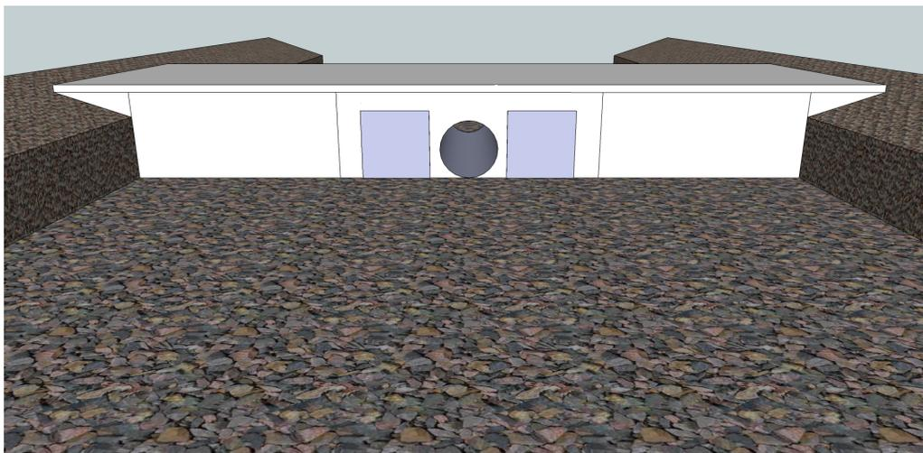
Figure 22: Diagram of Experimental Model S-6-C (The barrel is 6 inch diameter)
