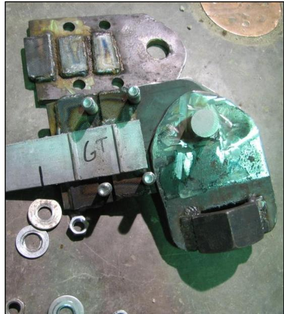
**Figure 5.19** Friction Gripper Used for Testing Strip Reinforcement in Type A Backfill
