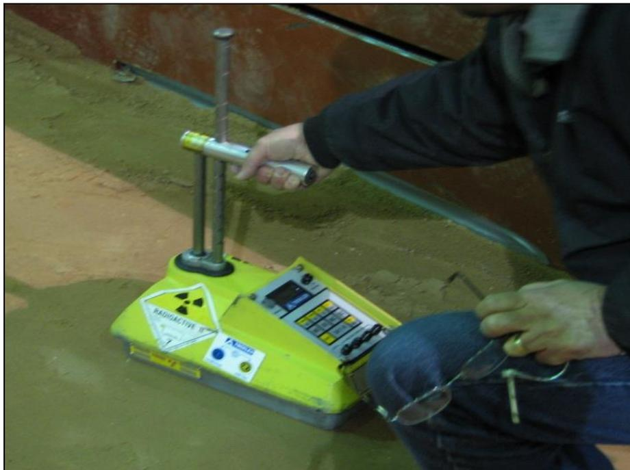
**Figure 5.12** Measurement of Compacted Density Using the Nuclear Density Gage
