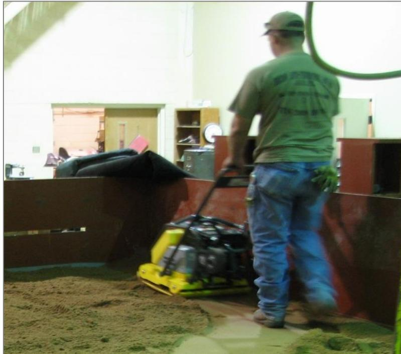
**Figure 5.11** Compaction of the Backfill in Test Box
