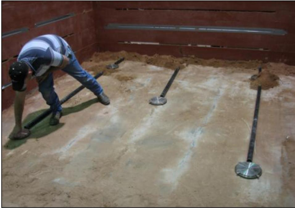
**Figure 5.10** Mounting Earth Pressure Cells on the Bottom Slab of Test Box
