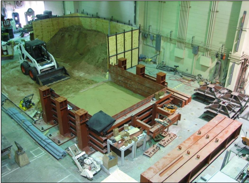
**Figure 5.6** Skid Steer Loader in Operation during Filling of the Test Box
