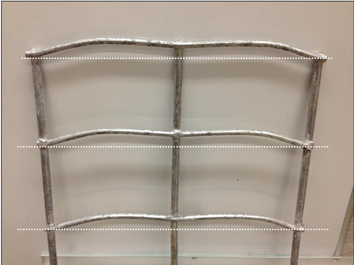
**Figure 6.41** Transverse Bar Deformation of an Exhumed Grid Reinforcement
