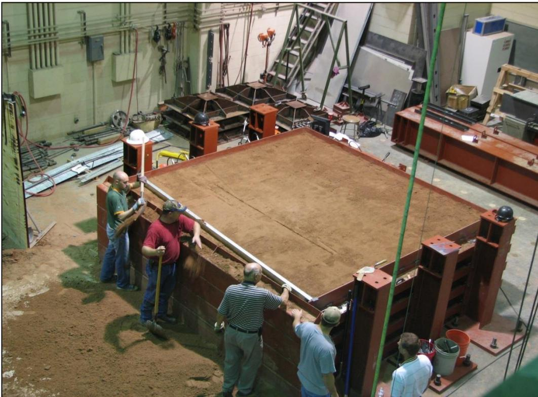
**Figure 5.16** Grading the Final Loose Lift of Backfill within the Test Box
