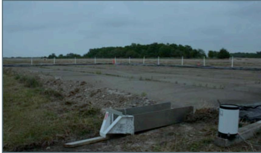
Figure 6: Photograph looking upstream from the outlet for the concrete surface watershed. Diagonal dimension from H-flume to orange cone in far corner is  $\approx 111$  feet. Dimensionless slope along the diagonal is 0.0025
