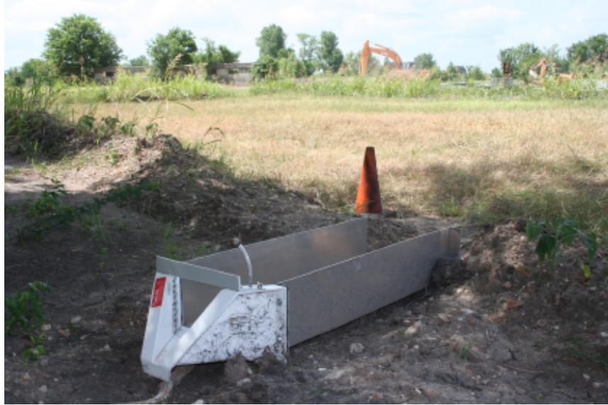
Figure 7: Photograph looking upstream from the outlet for the concrete surface watershed. Diagonal dimension from H-flume to the far corner (left of the orange machinery in the image background) is  $\approx 111$  feet. Dimensionless slope along the diagonal is 0.0025
