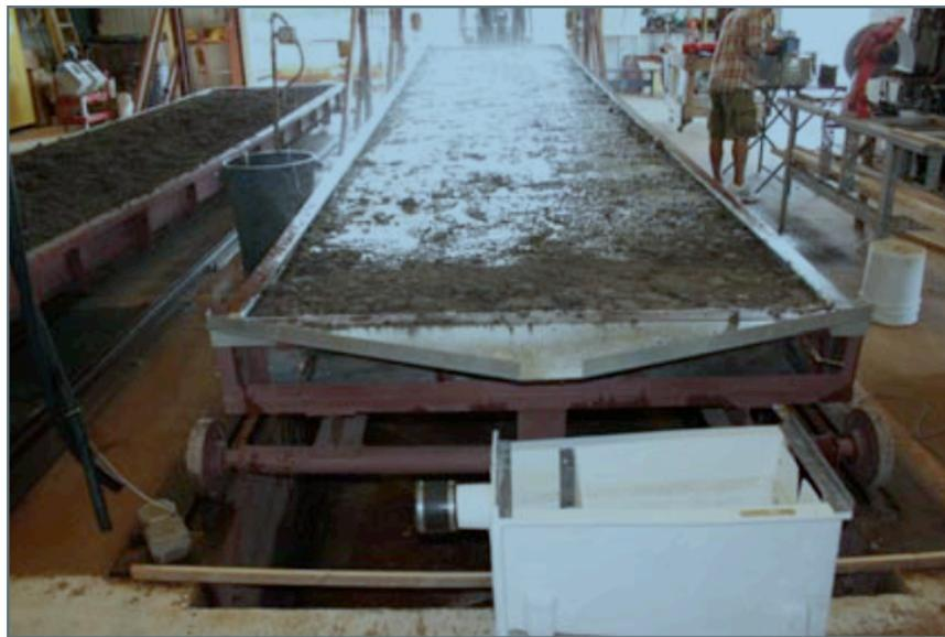
Figure 9: Photograph looking upstream from the outlet for the rainfall-simulator watershed. Longitudinal dimension from the outlet (foreground) to the end of the watershed is 30 ft.
