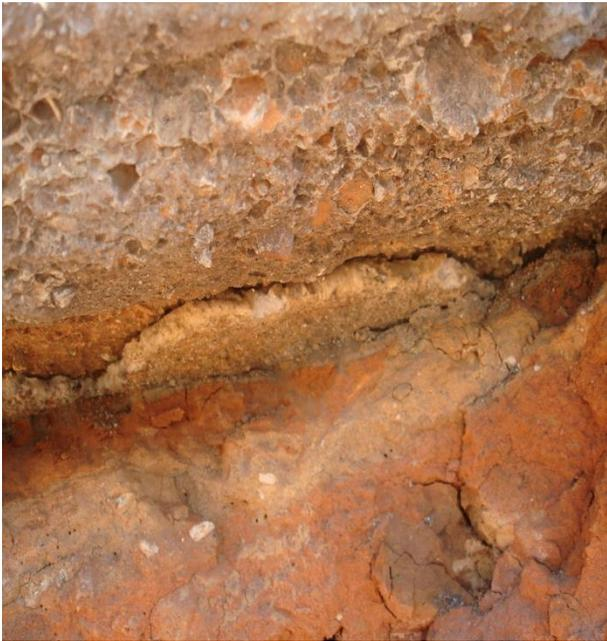
Figure 2.21 Undersealing material
