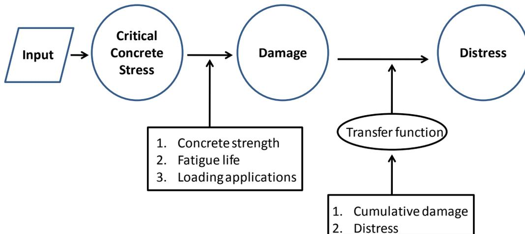
**Figure 7.1 Overall algorithm of mechanistic-empirical CRCP design procedure**
