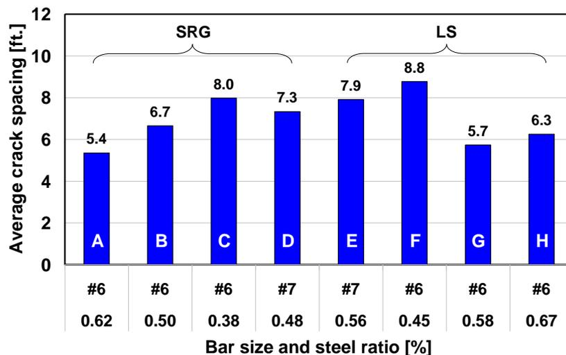
**Figure 4.4 Average Crack Spacing of All Sections in BW 8 Frontage Road**
