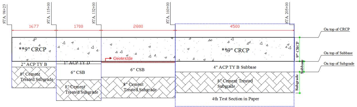
Figure 3.17 Test Section layout
