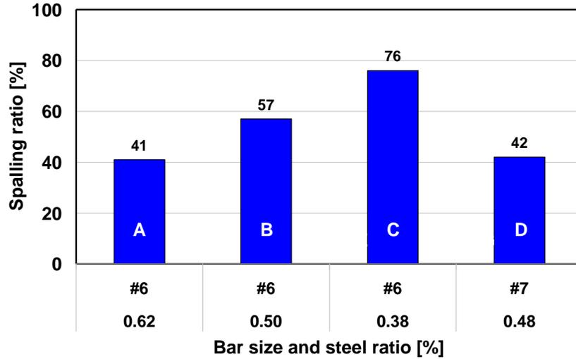
**Figure 4.9 Spalling Ratio for SRG Sections**
