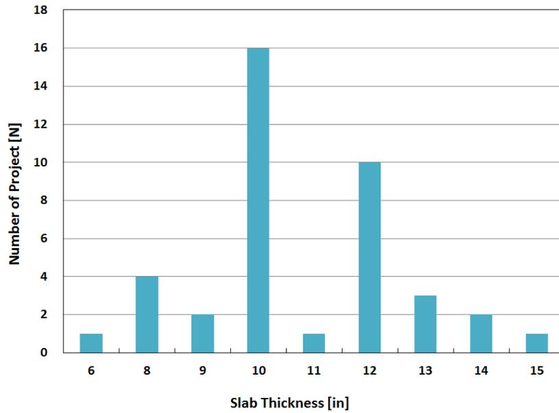
**Figure 7.5 Number Project Distribution vs. Slab Thickness**
