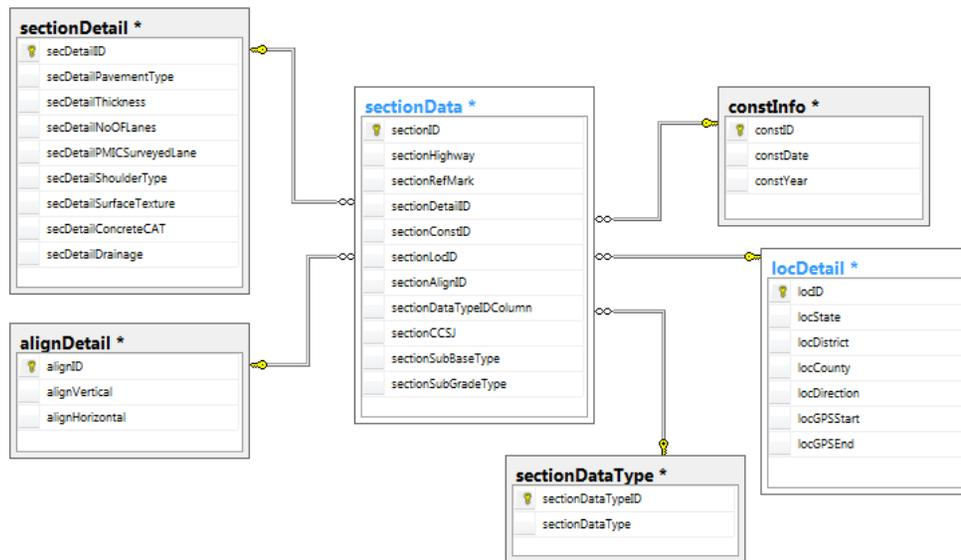
Figure 6.1 TxRPDB Database Architecture
