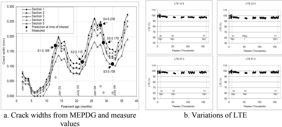
**Figure 3.12 Crack Widths from MEPDG and Measure Values and Variations of LTE (Kohler 2005)**
