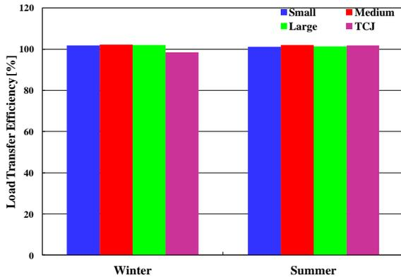
**Figure 3.8 LTE at various crack spacing and TCJ at two different seasons**
