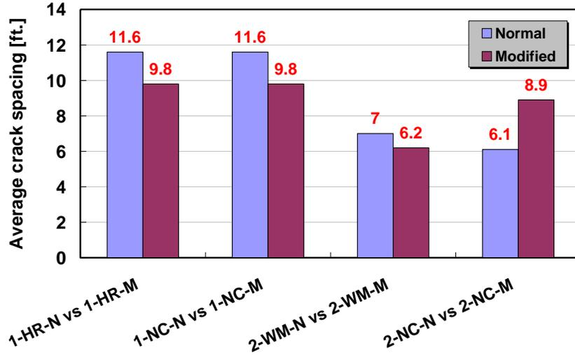
**Figure 4.41 Effect of Batching Method on Average Crack Spacing**
