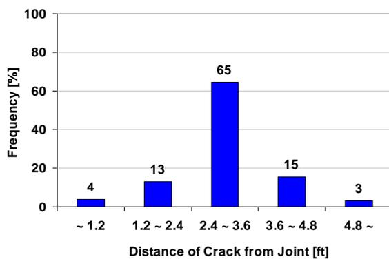
(c) Distance of Crack from Joint in Jointed Section
