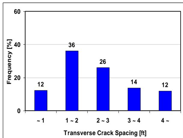
(b) Crack Spacing Distributions
