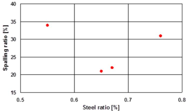
**Figure 4.17 Relationship between Steel Percentage and Spalling Ratio for SRG Sections**
