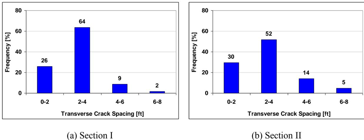
**Figure 4.49 Crack Spacing Distribution of US 290-2E Section**
