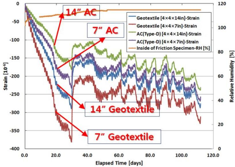
Figure 3.20 Concrete Prisms Strain
