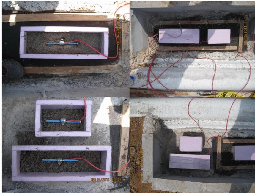
**Figure 3.19 Concrete Prisms**
