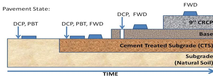
Figure 3.22 Field Testing
