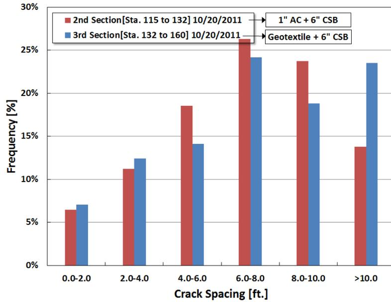
Figure 3.21 Transverse Cracking Pattern
