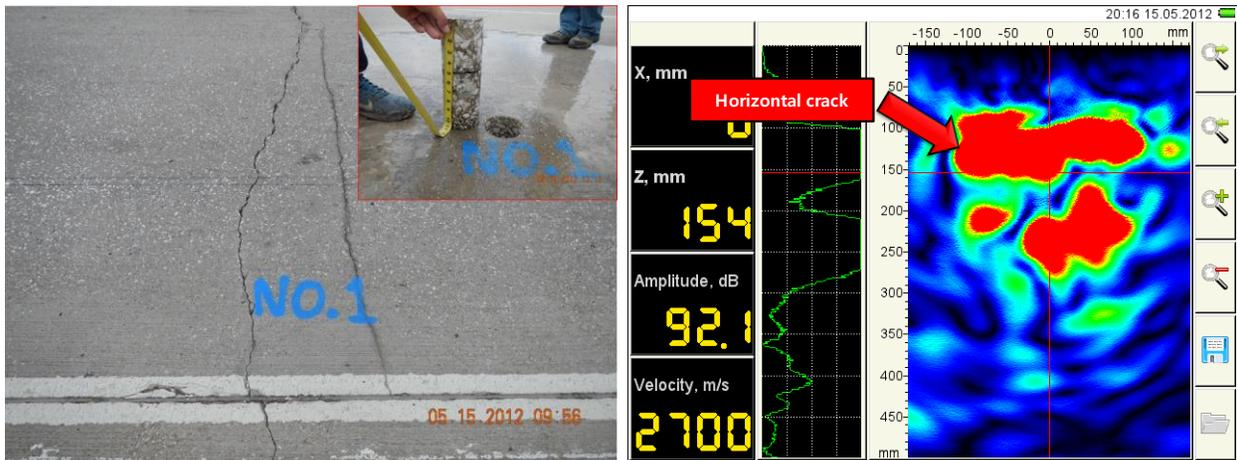
a. Horizontal crack in narrow transverse crack
