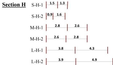
Figure C.5 Selected Cracks for FWD Testing in IH 45 Spring Creek Section (continued)
