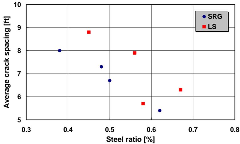
**Figure 4.5 Correlation between Steel Percentage and Crack Spacing in BW 8 Section**
