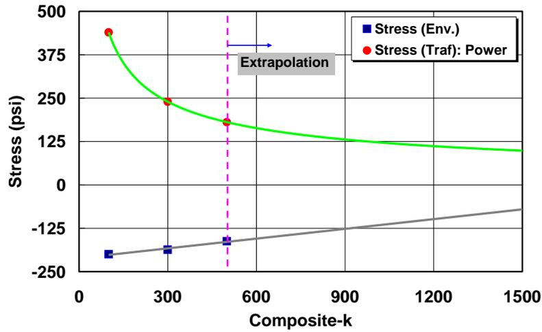
Figure 7.11 Extension of  $k$ -value Upper Limit Using Extrapolation Method
