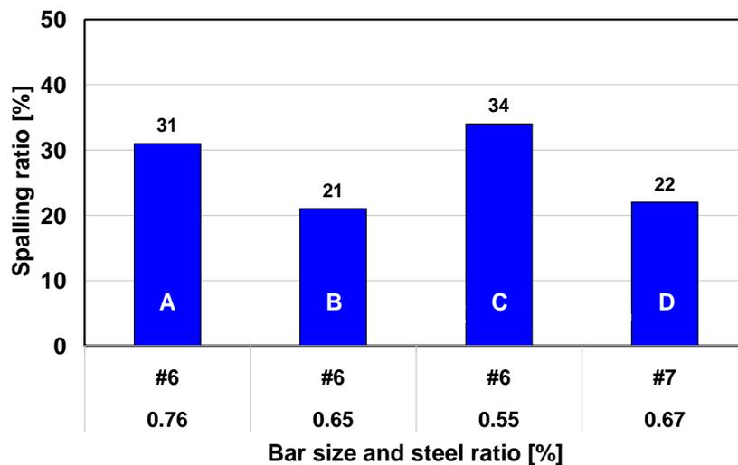
**Figure 4.16 Spalling Ratio for SRG Sections**
