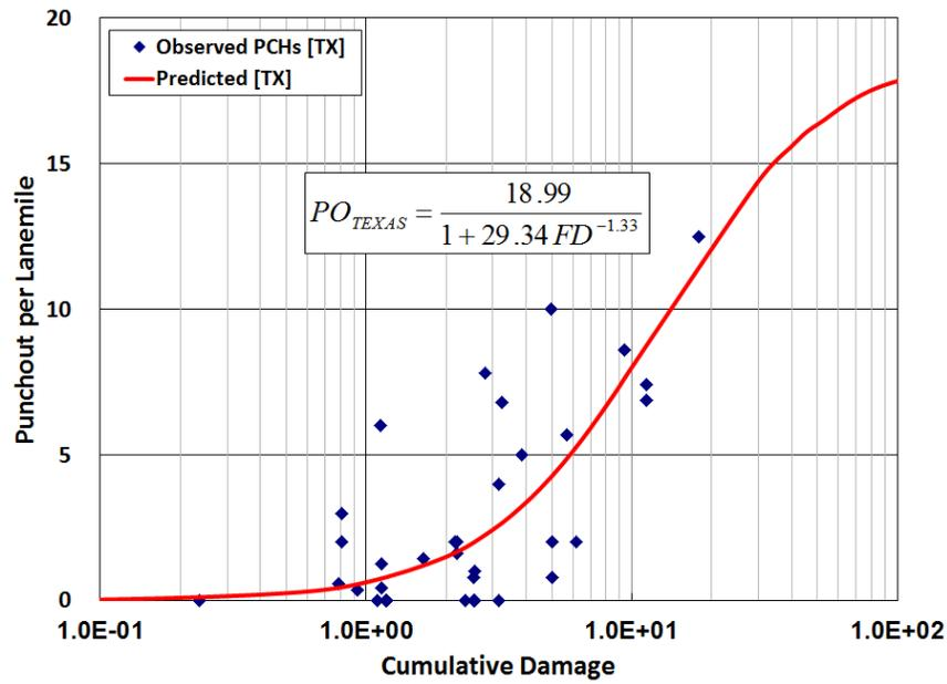
Figure 7.8 Transfer Function for TxCRCP-ME
