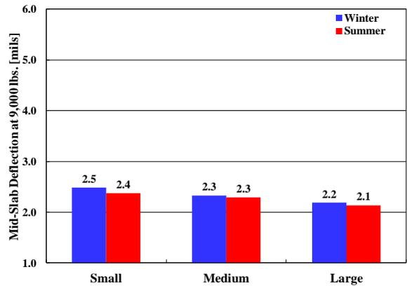
**Figure 3.7 Deflections at Cracks - Mid Slab at Level-I Test Sections**
