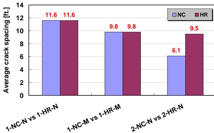
**Figure 4.43 Effect of Curing Method on Average Crack Spacing**
