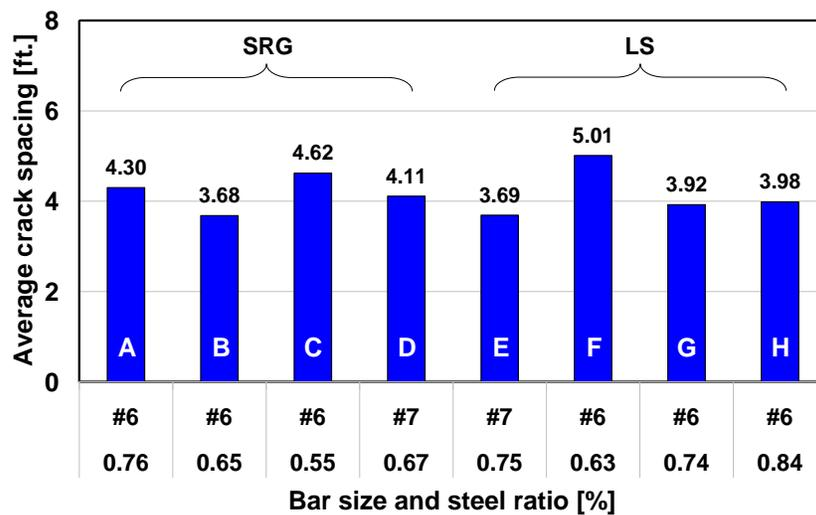
Figure 4.12 Average Crack Spacing in Various Sections
