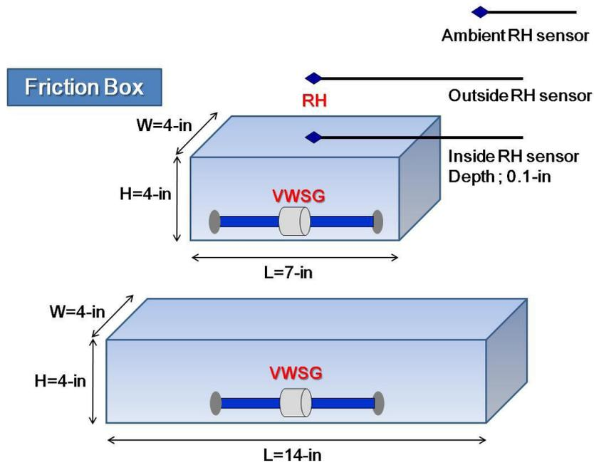
Figure 3.18 Concrete Prisms for Friction Evaluation
