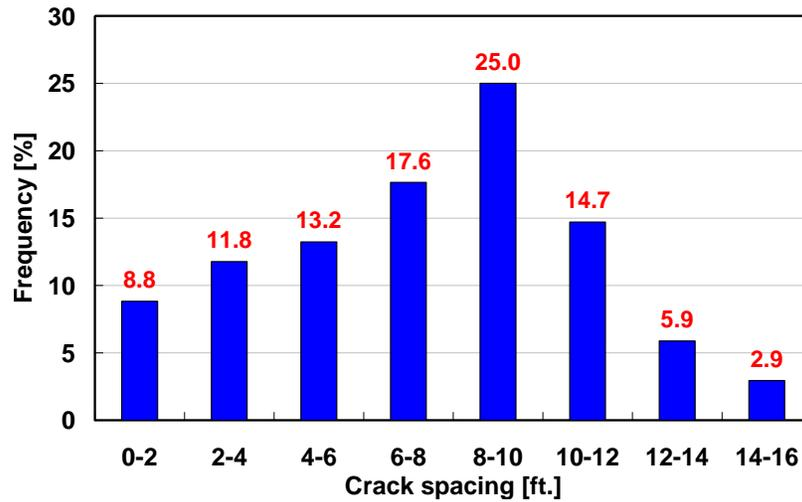
**Figure 4.32 Crack Spacing Distributions in in Van Horn IH 10 Section**
