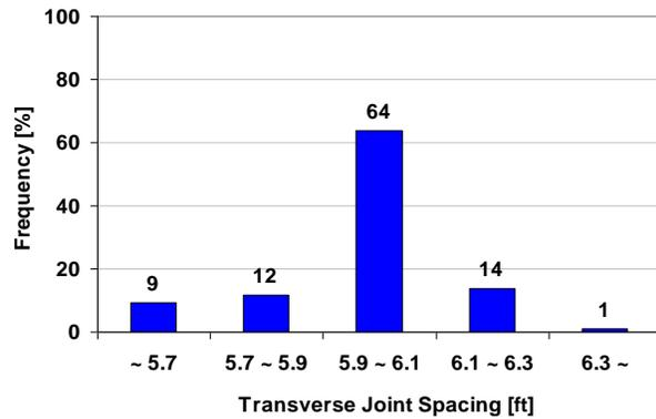
(a) Joint Spacing Distributions in Jointed Section
