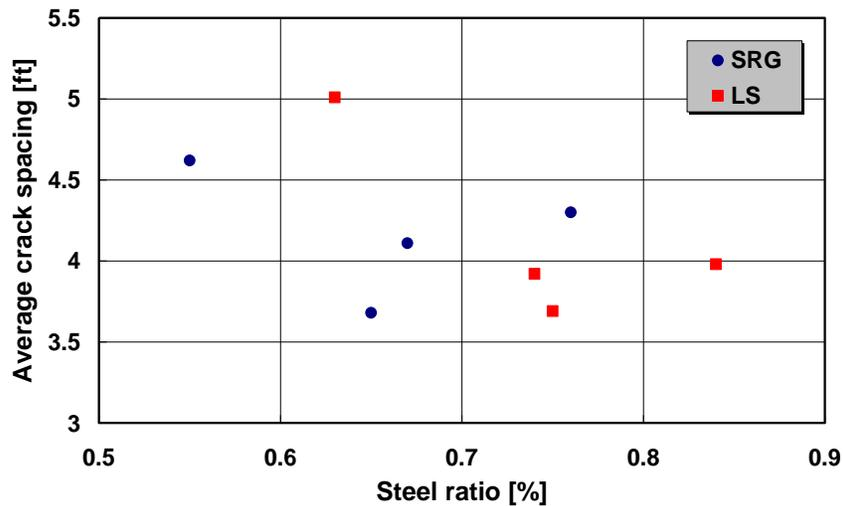
**Figure 4.13 Relationship between Steel Percentage and Crack Spacing in SH 45 Section**
