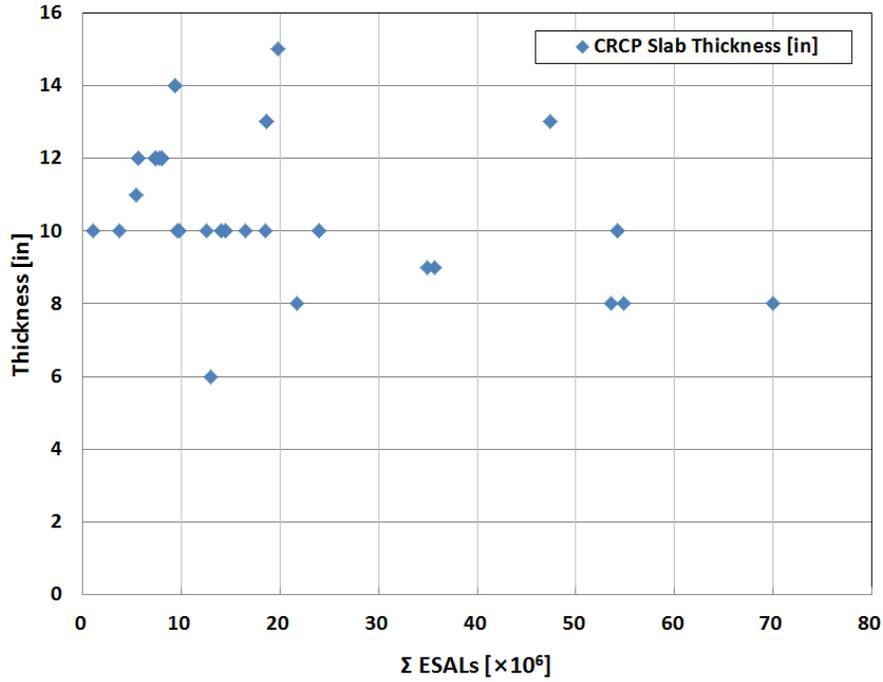
Figure B.7 Slab Thickness Distribution vs. ESALs
