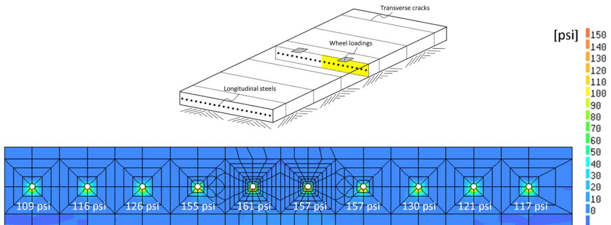
**Figure 7.14 Principal Concrete Stresses under Wheel Loading**
