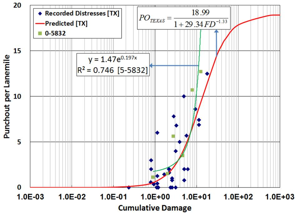
Figure B.8 Comparison of Transfer Function (0-5832 vs. 0-6274)
