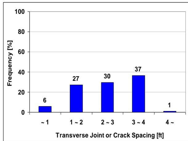
(b) Joint or Crack Spacing Distributions
