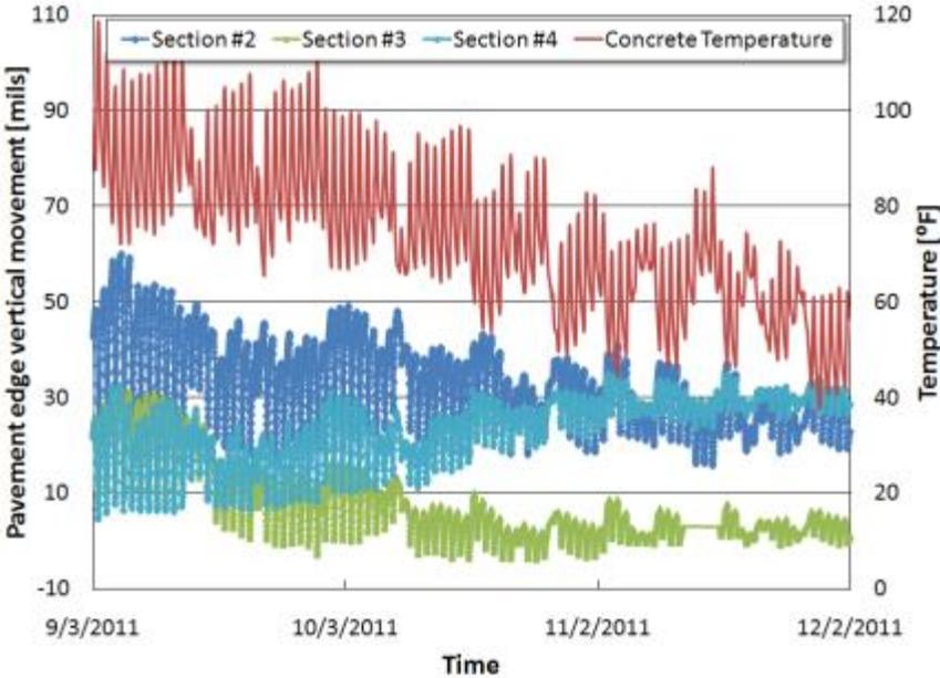
**Figure 3.2 Pavement edge vertical movements**
