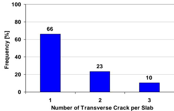
(b) Number of Transverse Cracks per Slab in Jointed Section
