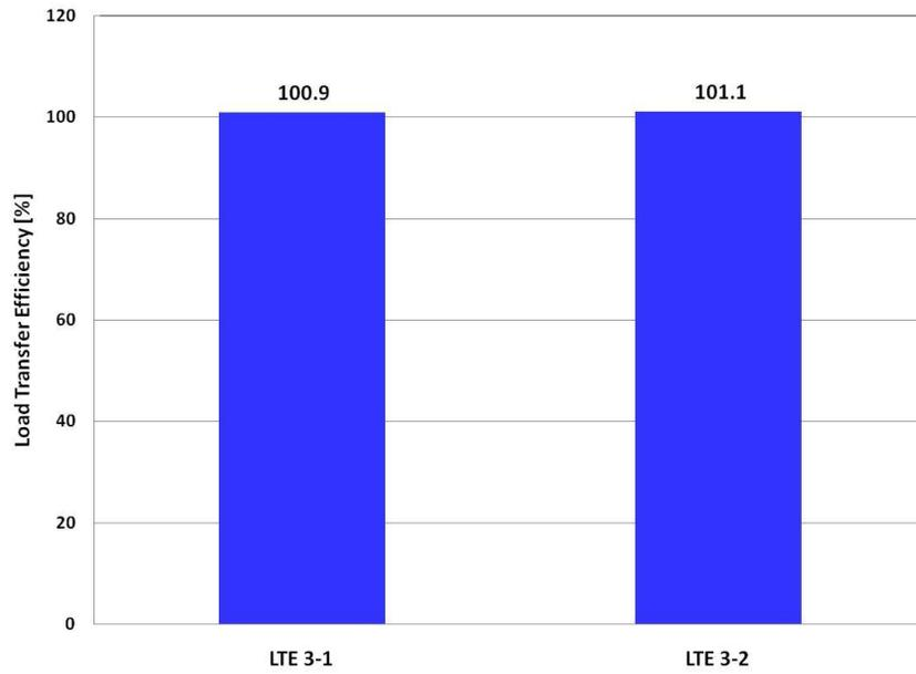
**Figure 2.17 LTE in Upstream and Downstream of Punchout Slab**
