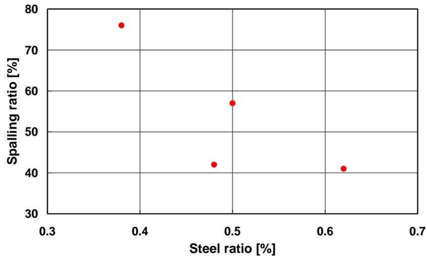
**Figure 4.10 Relationship between Steel Percentage and Spalling Ratio for SRG Sections**
