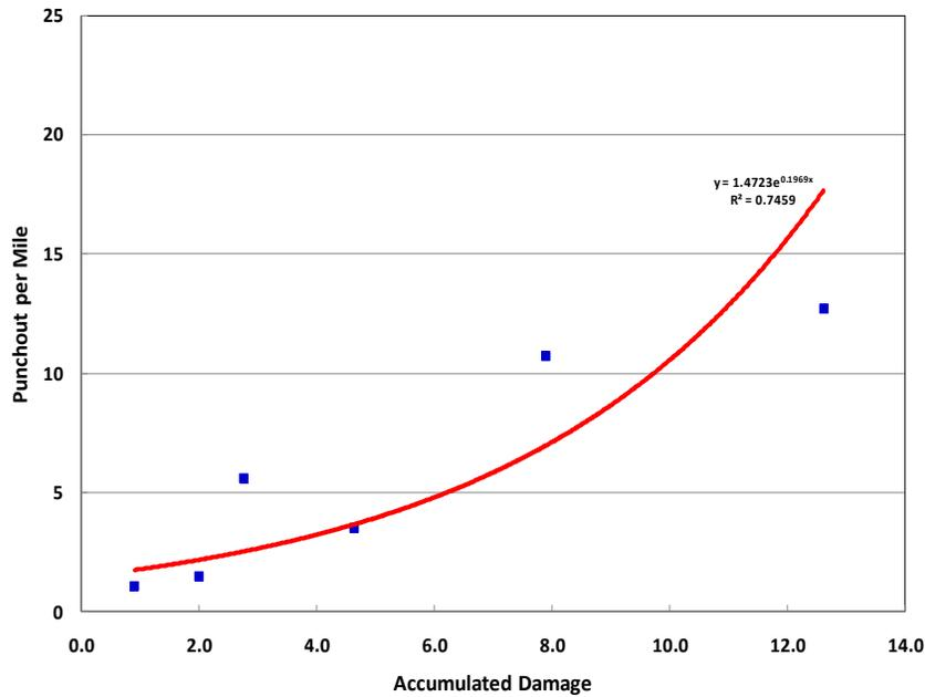
**Figure 7.2 Transfer Function in TxDOT Research Project 0-5832**
