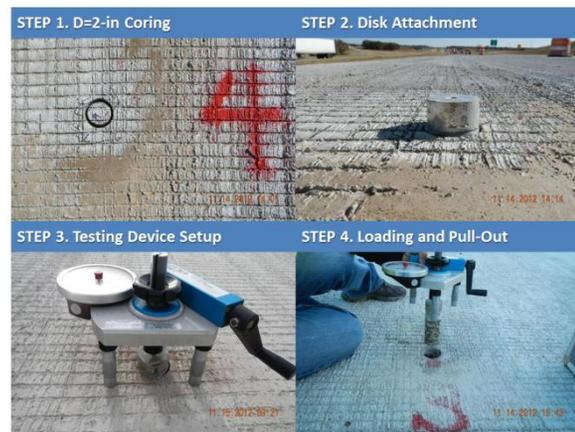
b. Bond strength testing procedure
