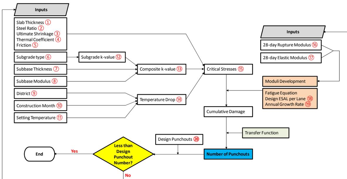
Figure 7.12 Architecture of TxCRCP-ME Software
