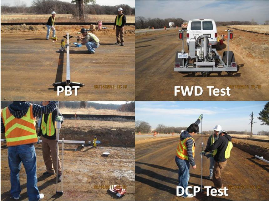
Figure 3.23 Various Field Testings
