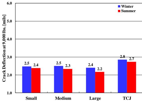
**Figure 3.6 Crack Deflections at Level-I Test Sections**
