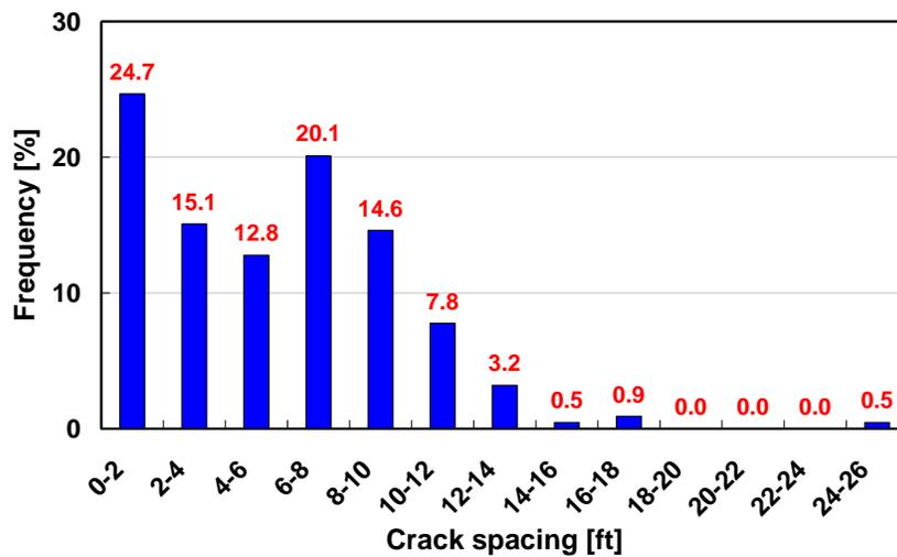
Figure 4.59 Crack Spacing Distributions for Kendleton US 59S Section
