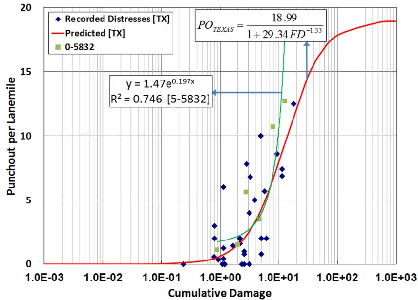
Figure 7.9 Comparison of Transfer Function between LTPP and Texas
