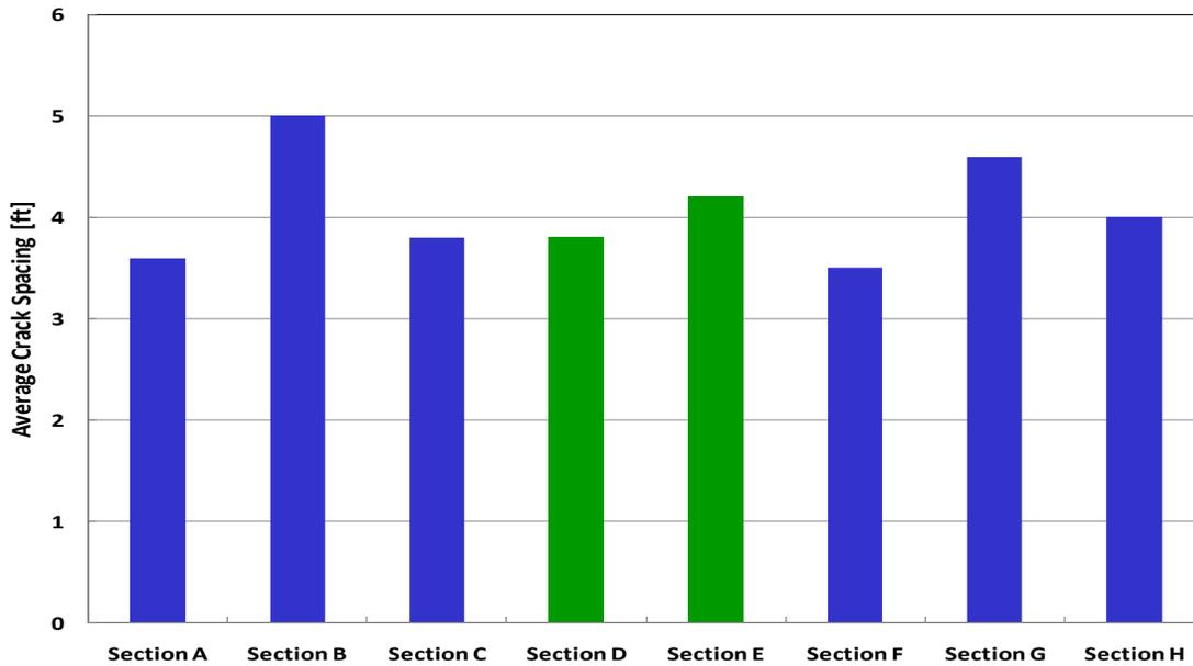
Figure 2.11 Average Crack Spacing in Various Sections
