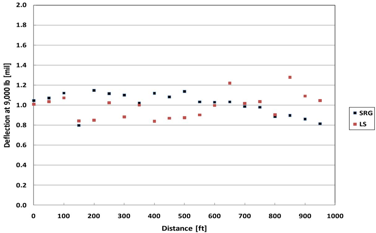
Figure 2.12 Deflection at SRG and LS Sections
