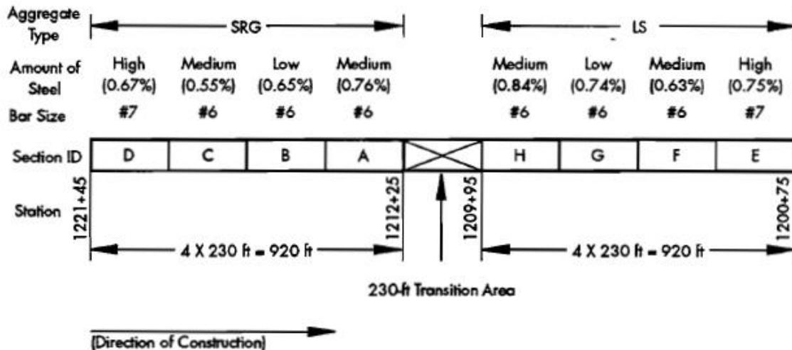
Figure 2.10 Layout of Test Sections in IH 45 in Spring Creek
