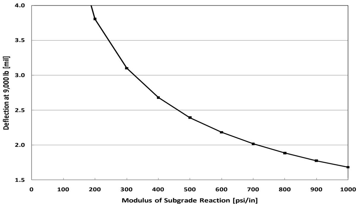
Figure 4.6 Deflections at Interior Condition for Various Modulus of Subgrade Reaction
