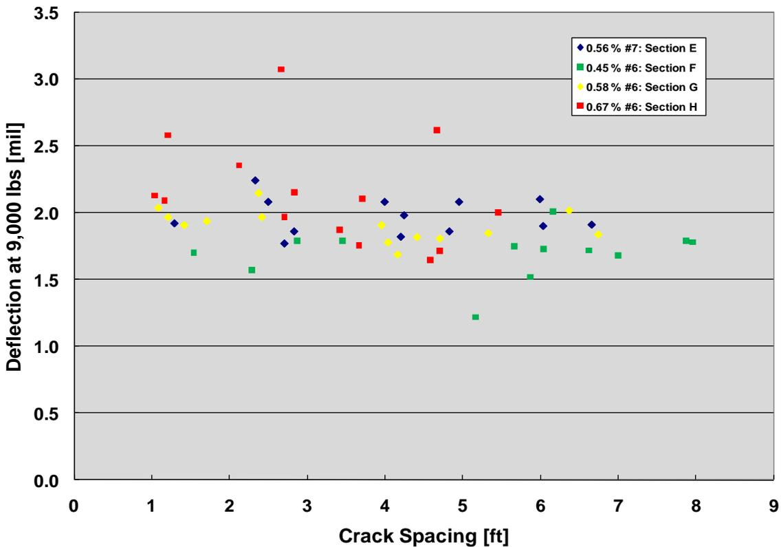
Figure 2.5 Crack Spacing and Deflections for Various Steel Percentages
