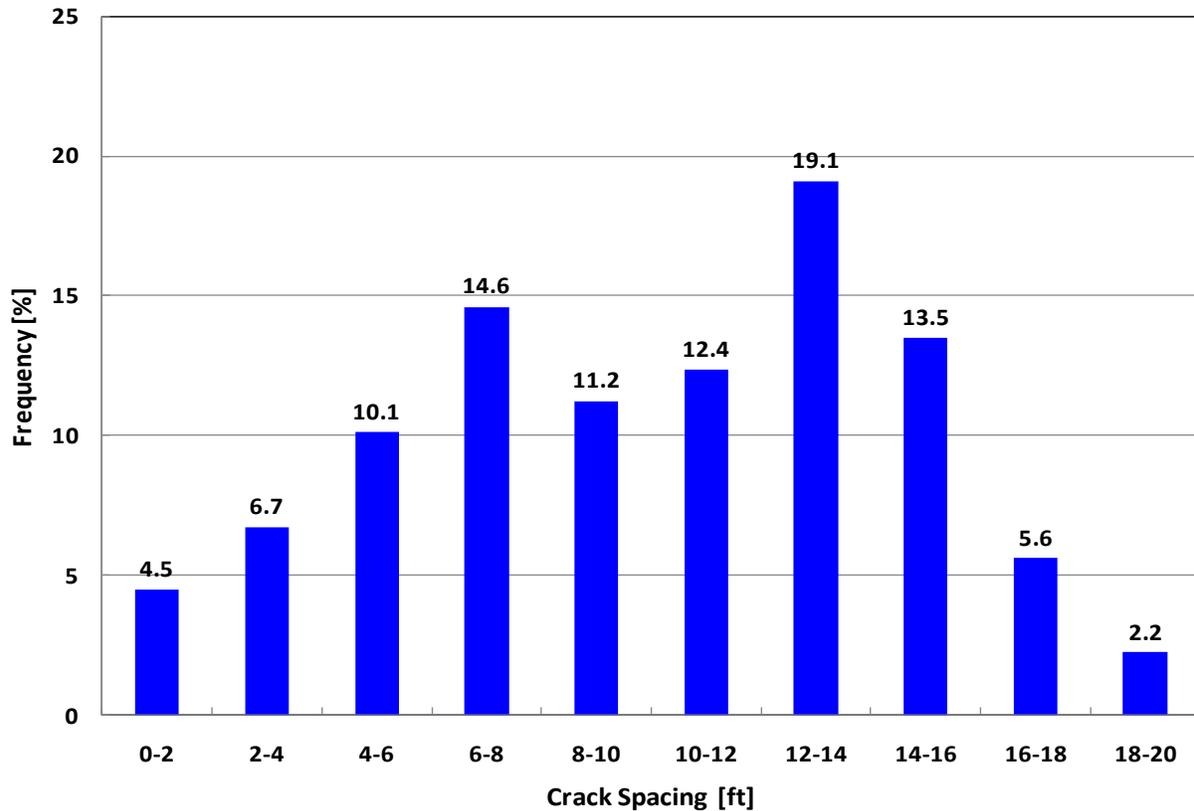
Figure 2.17 Crack Spacing Distribution in Baytown Section in 2010
