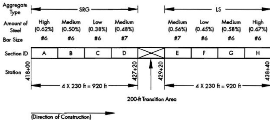
Figure 2.2 Layout of Test Sections in BW 8 Frontage Road
