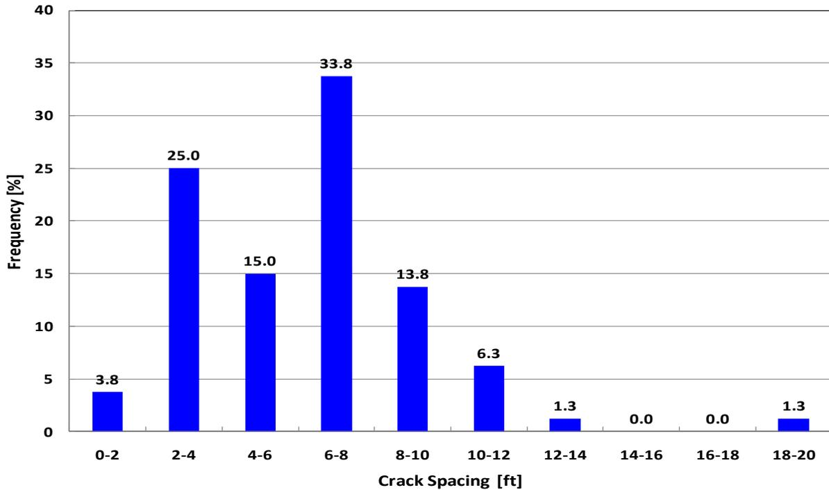
Figure 2.16 Crack Spacing Distribution in Cleveland section in 2010
