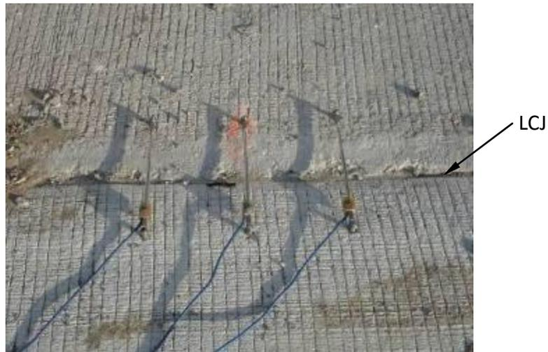
(a) Crackmeters installed at the surface across the LCJ in the tied section
