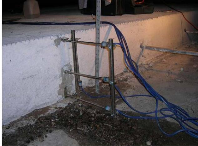
(a) Crackmeter for transverse movement measurements
