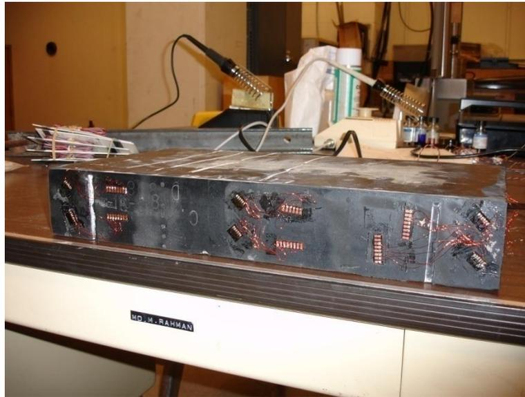
Figure 4.19 – Strain Gage Installed, 32-in. by 9-in. Bearing
