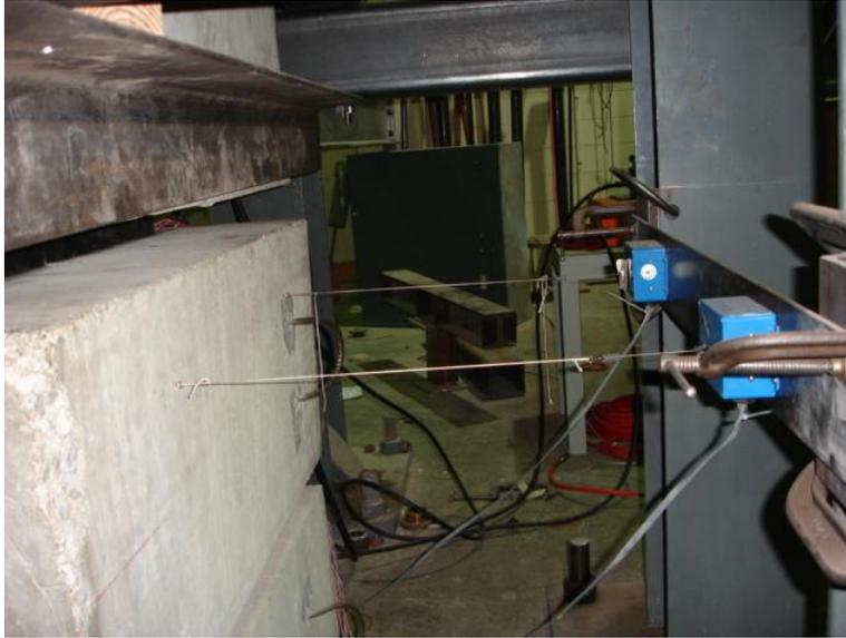
Figure 4.21 – Cable Extension Displacement Sensors – Longitudinal Direction
