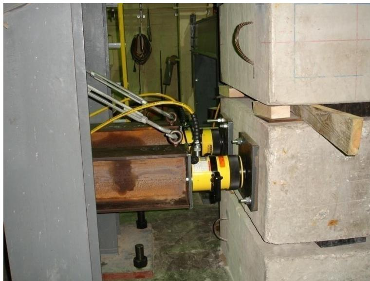
Figure 4.13 – Elevation View of Longitudinal Rams
