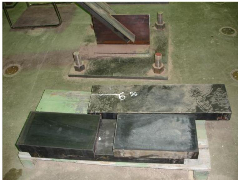
Figure 4.15 – Standard Single and Double Bearings
