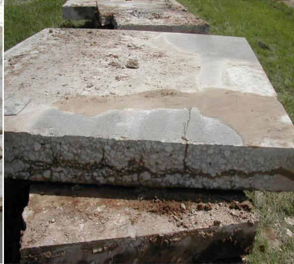
Figure 2.6-(b) Horizontal and longitudinal cracks on US281 in Wichita Falls
