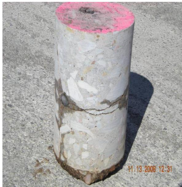
Figure 2.14-(b) Core showing horizontal cracking and longitudinal crack on steel
