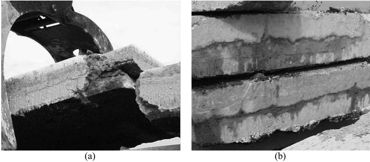
Figure 2.6: Horizontal cracks in slabs removed from IH30 in Paris District
