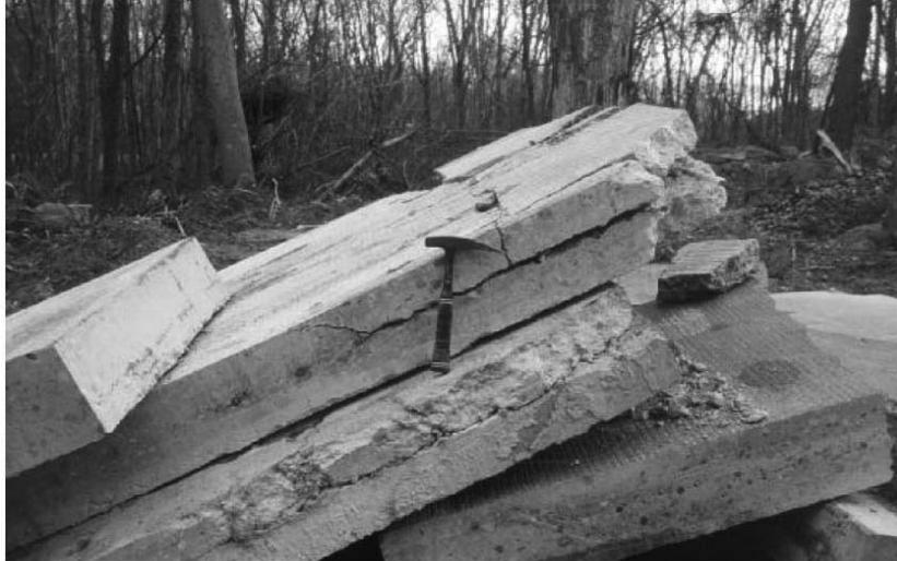
*Figure 2.11: Slabs with horizontal cracks*
