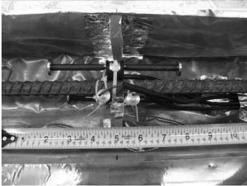
(a) Plan view of installed VWSGs
