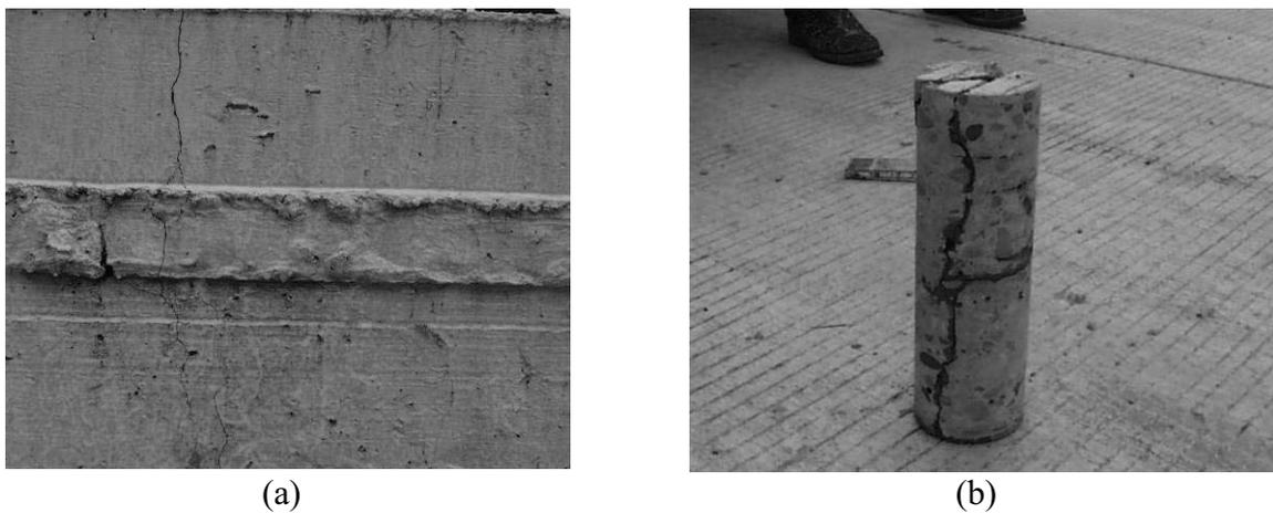
*Figure 2.3: Horizontal cracking in new CRCP*
