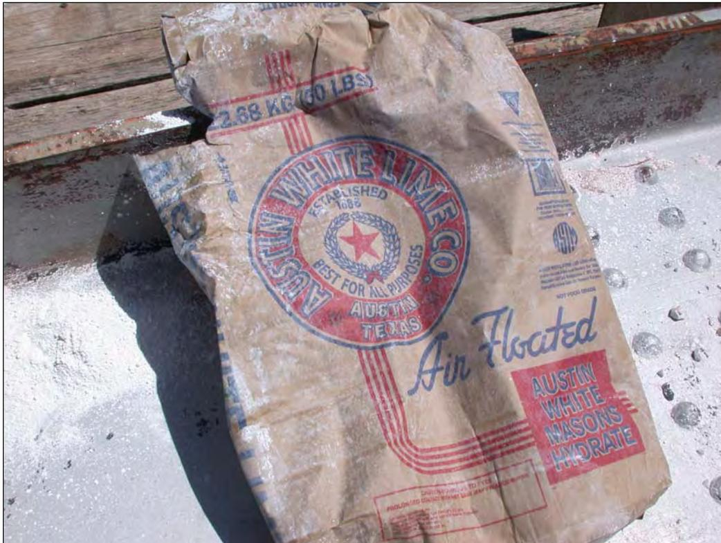
**Figure 6.11** 50-lb Bag, Type A Hydrated Lime
