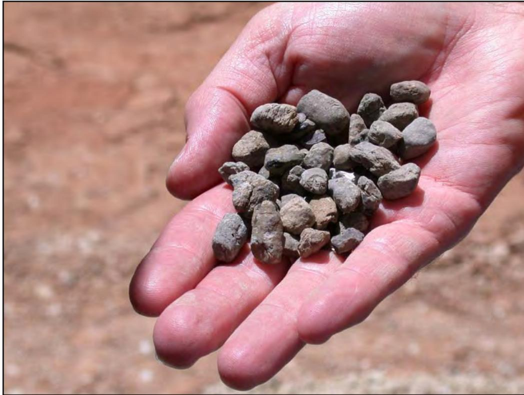
**Figure 4.2** Dirty Seal Coat Aggregate
