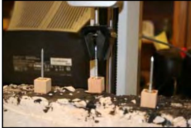
**Figure 3.6** Pullout Strength Testing Arrangement
