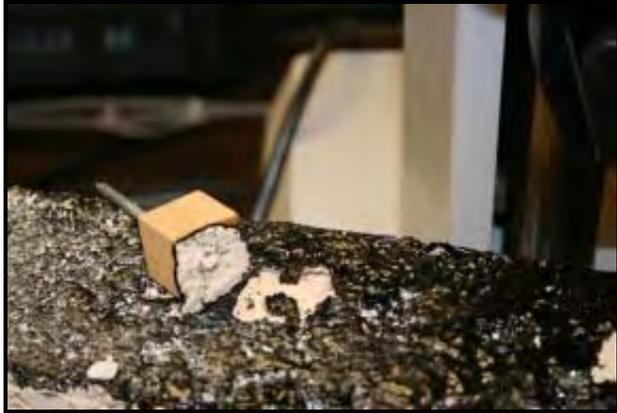
**Figure 3.16** Unusual Failure in Pullout Test (See note in Table 3.6)
