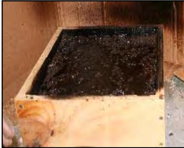
**Figure 3.3** Prime Coated Specimen after Curing
