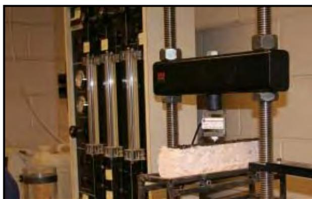
**Figure 3.5** Flexural Strength Testing Arrangement
