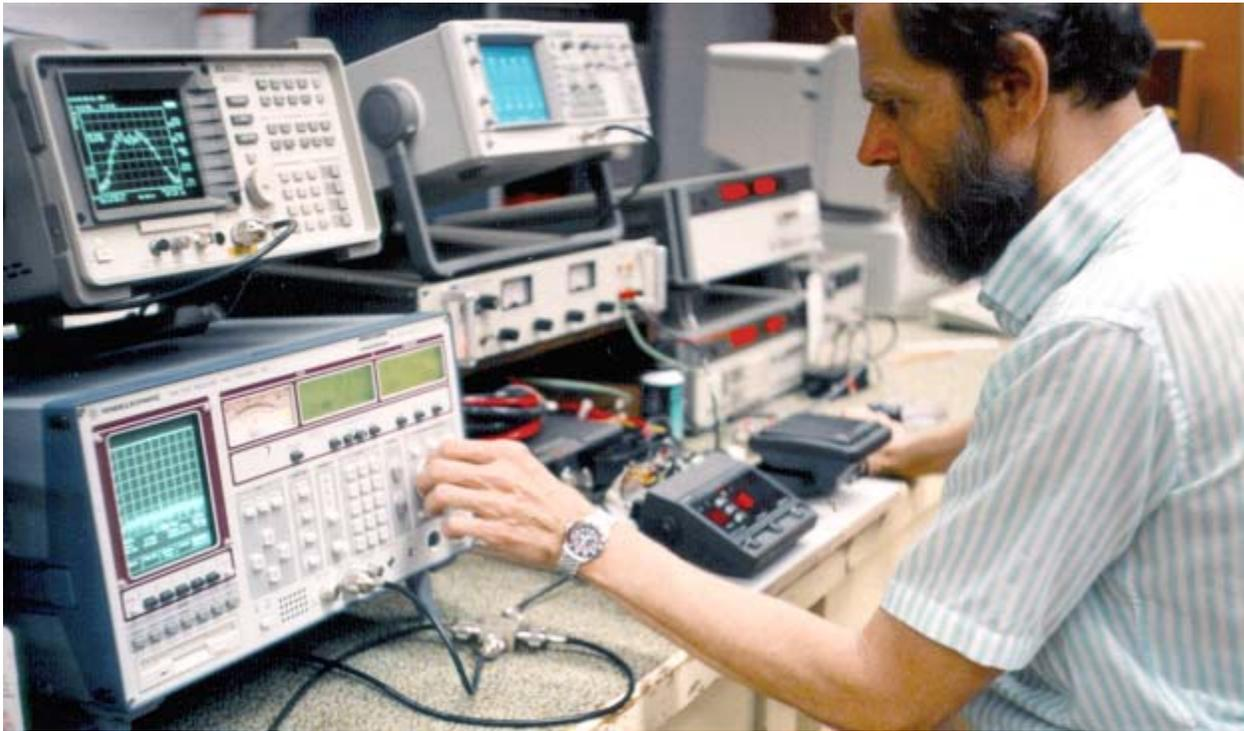
**Figure 2: Bench-Top Testing with a TxDOT Radio in a Laboratory at Texas Tech University**
