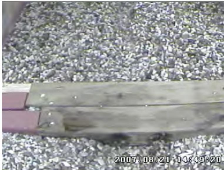
Figure 2.9: Image of Physical Model Experimental Configuration — 2-Barrel Circular Culvert. This image is from an actual experiment — water is running through the culvert in the image (downstream is into the image.)
