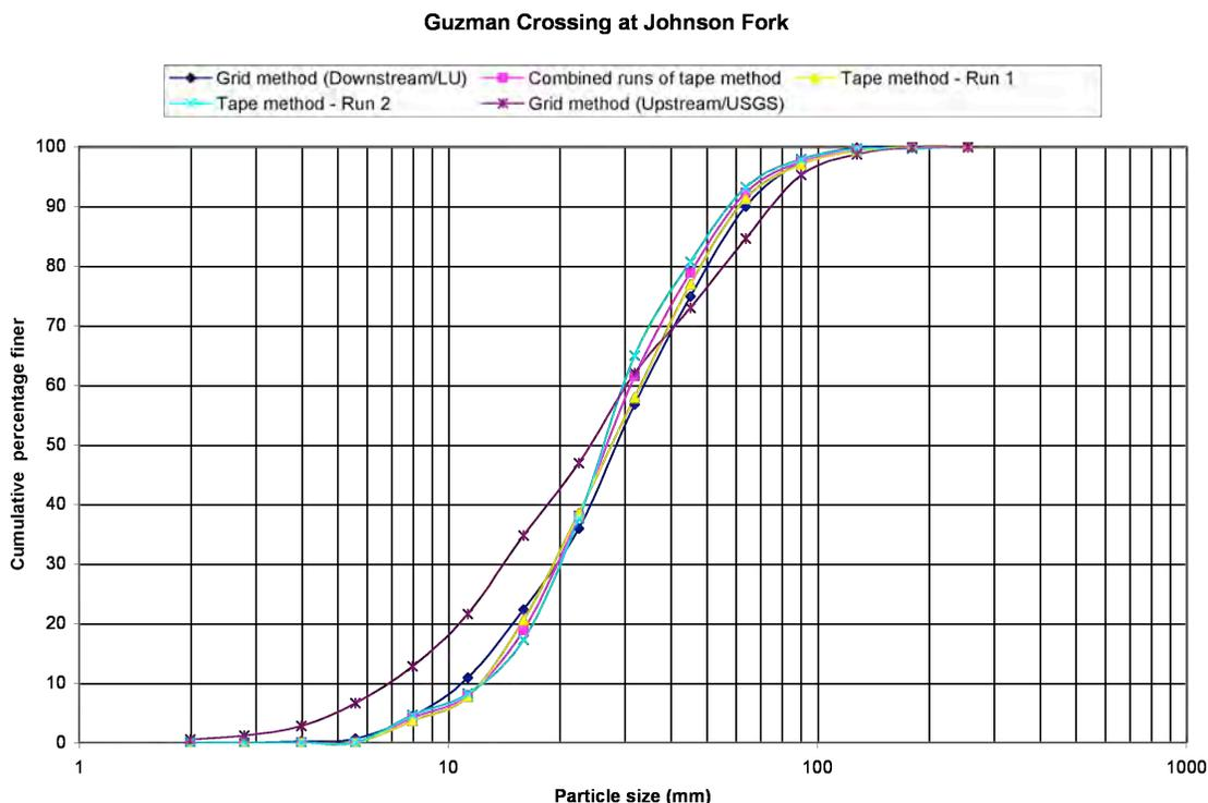
Figure 3.2: Particle-size distributions for bed sediments at the Guzman crossing of Johnson Fork Creek near Junction, Texas.
