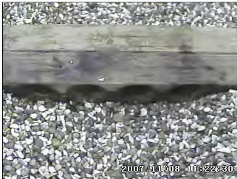
Figure 2.11: Image of Model Experimental Configuration — 4-Barrel Circular Culvert. Flow downstream is into the image.
