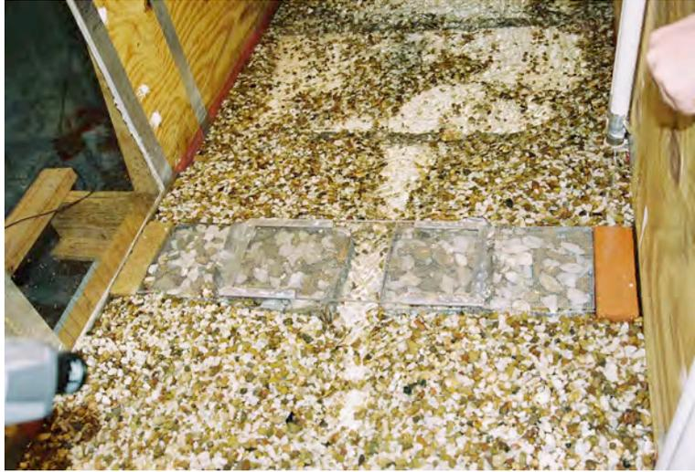
Figure 2.13: Image of Physical Model Experimental Configuration — Porous Culvert. Plastic cover representing roadbed in-place in this image.
