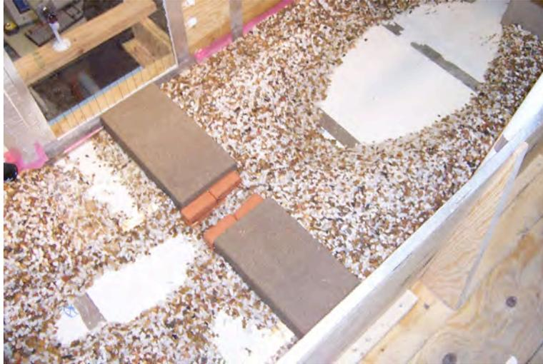
Figure 2.7: Image of Physical Model Experimental Configuration — Rectangular Culvert (cover removed). Note the eroded materials upstream and downstream (an upstream moving headcut) and the material removed just downstream of the rectangular section as well as the model roadbed. Flow was from the right to the left.
