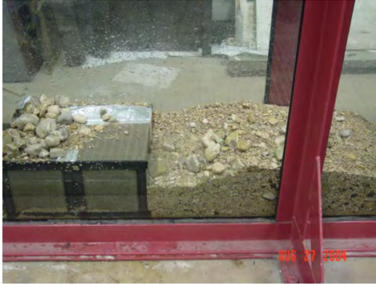
Figure 3.8: Deposition downstream from “road bed” after flood waters receded during the qualitative physical model run of late August 2004.
