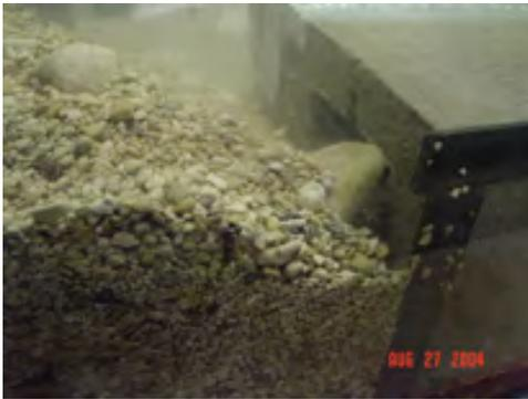
(c) Gravel bed filling culvert.
