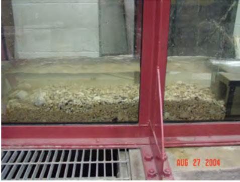
(a) Upstream portion of model looking towards culvert. Entire “road bed” is submerged.
