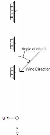
Figure E. 1. Anemometer Orientation and Angle of Attack Sign Convention
