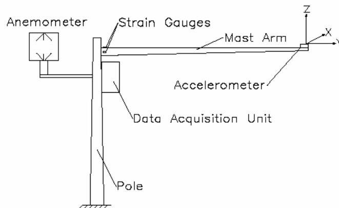
Figure 2.16 Equipment Layout for Galloping Experiment (Florea 2005)
