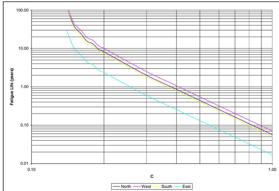
Figure 5.14. Effect of Factor  $C$  on the Prediction of the Fatigue Life of Mast Arms with Backplates
