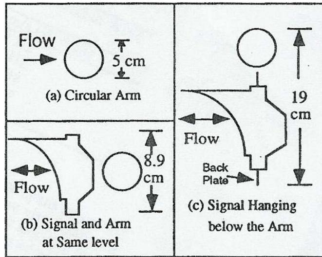
Figure 2.5 Models Used for Water-Table Experiments
