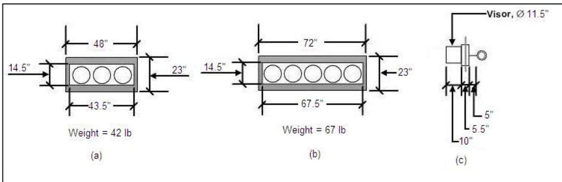
Figure 3.4 Dimensions of Signal Heads Used in Full-Scale Experiments (shown with backplates)
