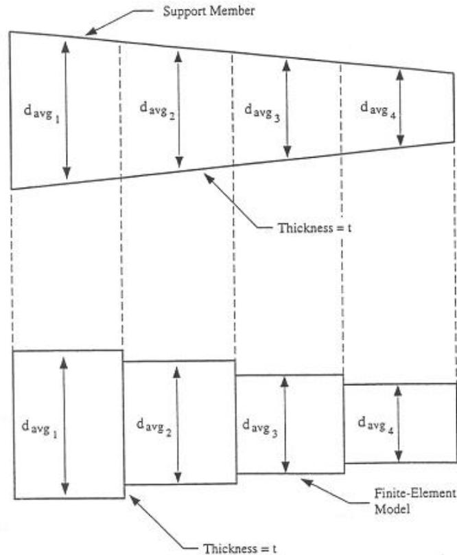
Figure 5.7 Finite-Element Modeling of Tapered Element
