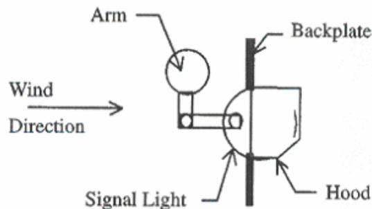
Figure 2.7 Signal Light Configuration Considered Susceptible To Galloping (Pulipaka, Sarkar, and McDonald 1998)
