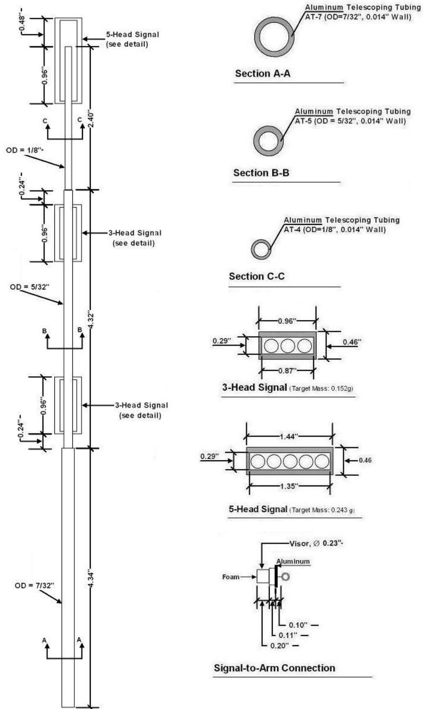
Figure 4.1 Design Drawing for Wind Tunnel Model
