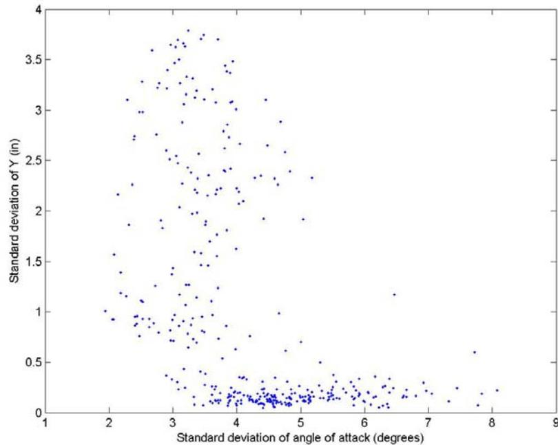
Figure 3.23 Effect of Variations in Angle of Attack on Vertical Vibrations
