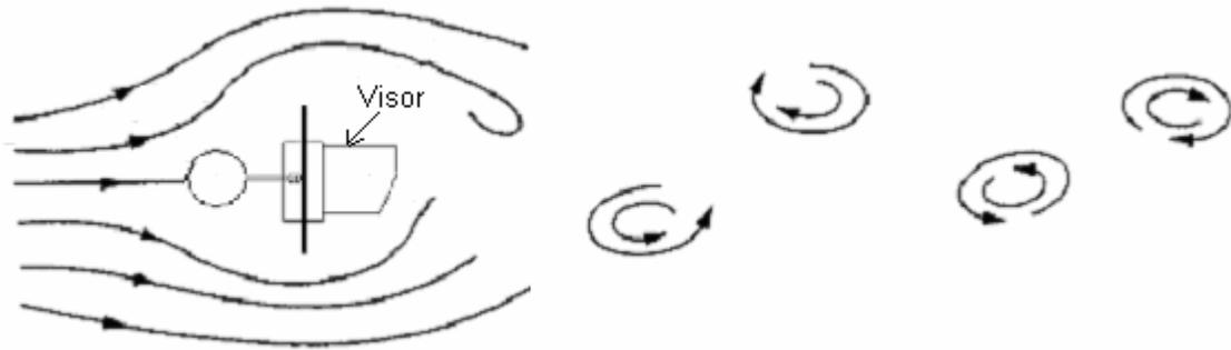
Figure 2.2 Vortex Shedding Acting on Cross-Section of Mast Arm with Traffic Signal
