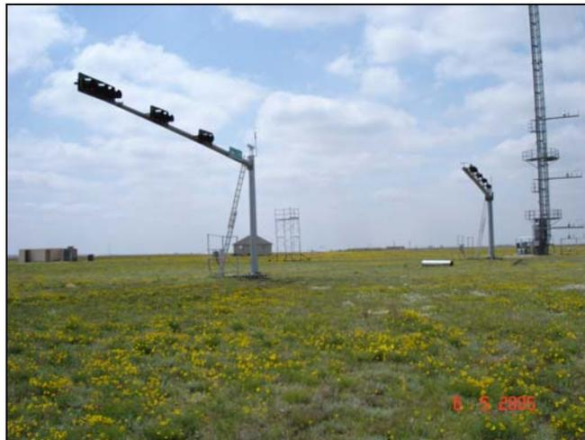
Figure 3.1 The Two Cantilever Traffic Signal Structures Tested at Reese Technology Center
