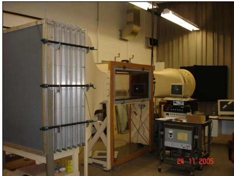
Figure 4.2 Open Circuit Small Wind Tunnel (OCSWT)
