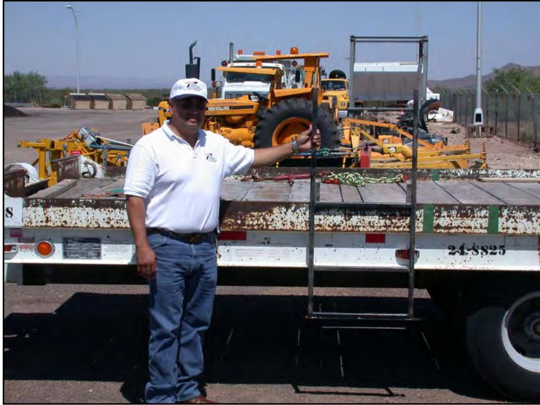
**Figure 5.8** Storable Ladders on Trailers Help Provide for Worker Safety
