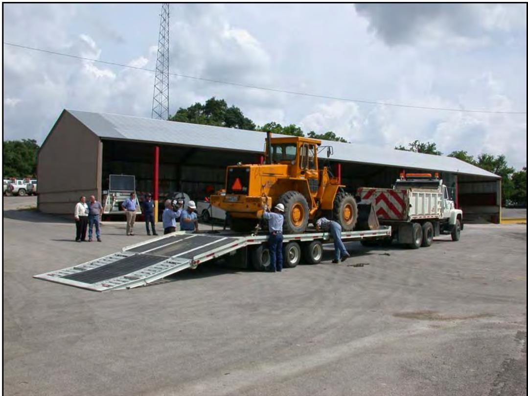
**Figure 1.1** Common TxDOT Equipment Transport Practice: a Heavy Construction/Maintenance Equipment Load (Front End Loader) Is Tied on a Tag-A-Long Trailer (Dovetail Style, Pintle Hitch) and Pulled by a 10 CY Dump Truck
