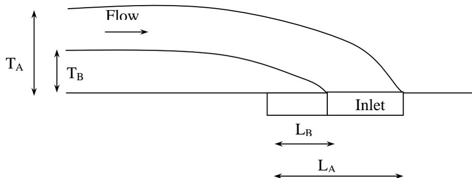
Figure 2.8 Characteristic spread  $T_A$  and  $T_B$  corresponding to inlet sizes  $L_A$  and  $L_B$  (after Fiuzat *et al.*, 2000)
