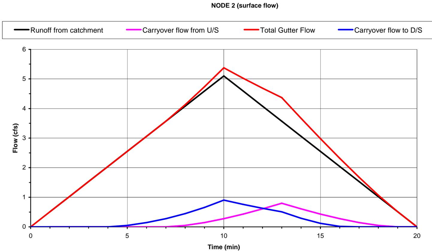
Figure C.3. Simulated **surface flow** components at the inlet I-2 (node 2) by using modified SPLIT program.
