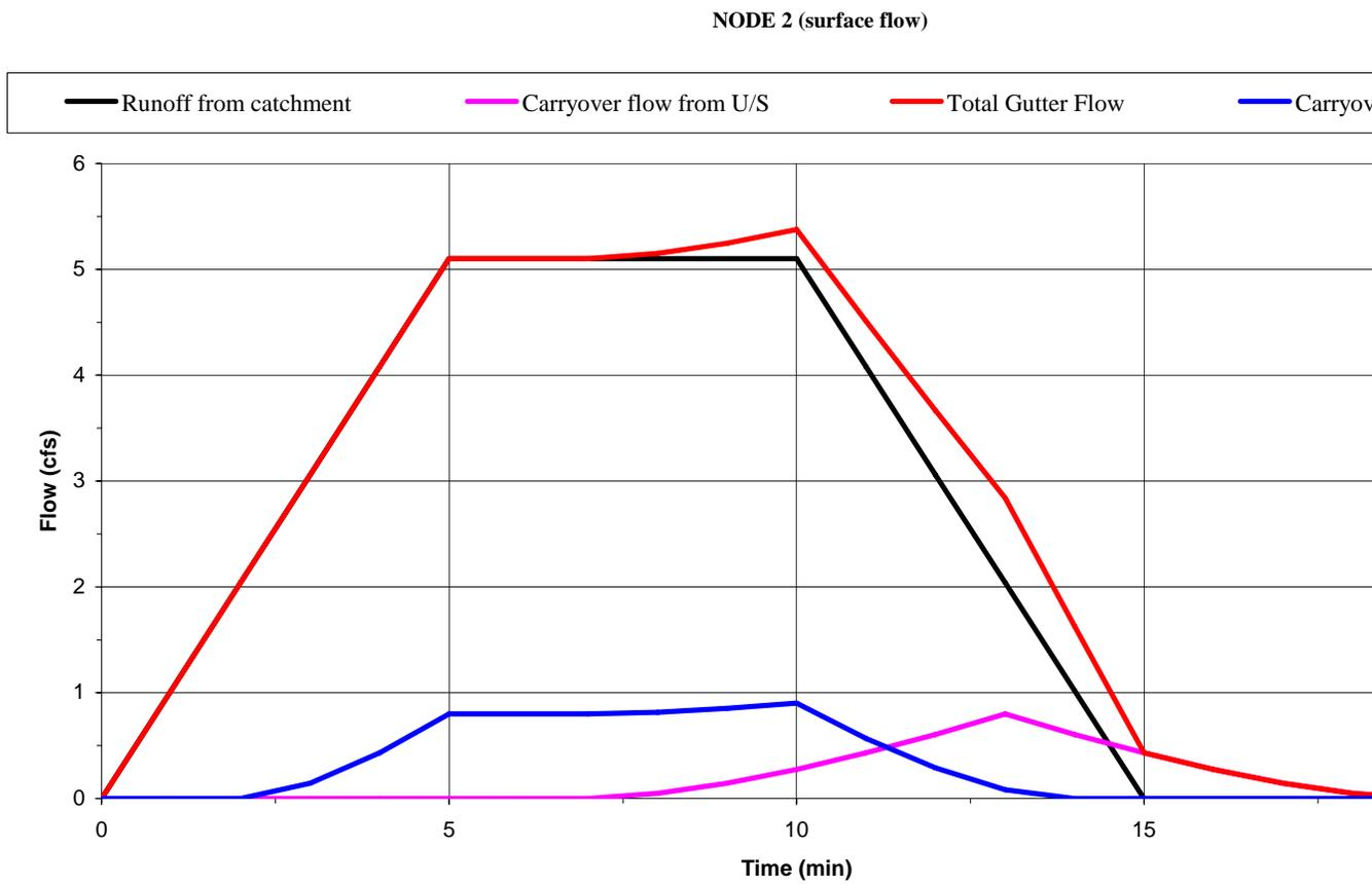
Figure C.6. Simulated **surface flow** components at the inlet I-2 (node 2) by using modified SPLIT program ( $T_c=5$  min.).
