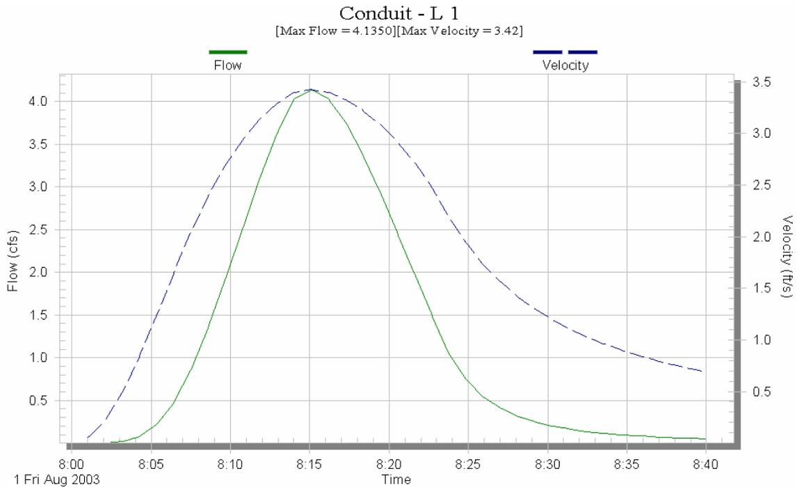
Figure 5.3. Time series plot of flows and velocity by SWMM for conduit L1.
