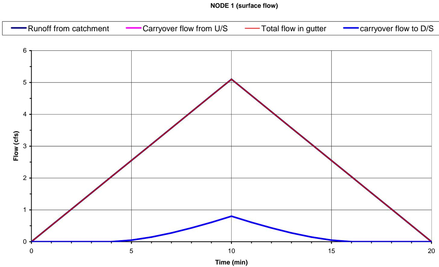
Figure C.1. Simulated **surface flow** components at the inlet I-1 (node 1) by using modified SPLIT program.
