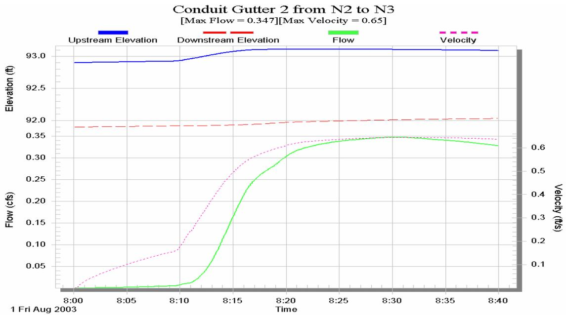
Figure D.26 Variation in flow and elevation with respect to time in the surface conduit Gutter 2.
