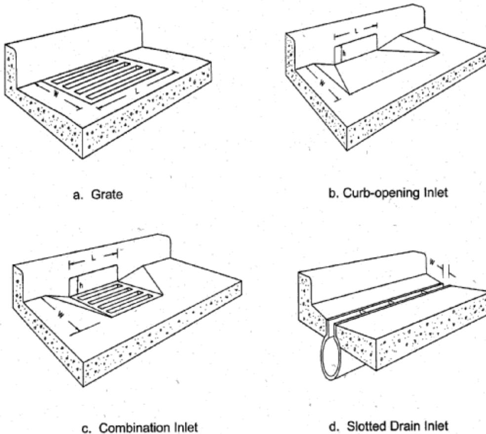
Figure 2.4. Types of storm drain inlets (Brown *et al.*, 2001).
