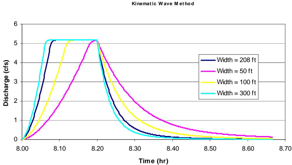
Figure D.6c. Sub-catchment hydrographs developed by Kinematic Wave Method with different basin widths.
