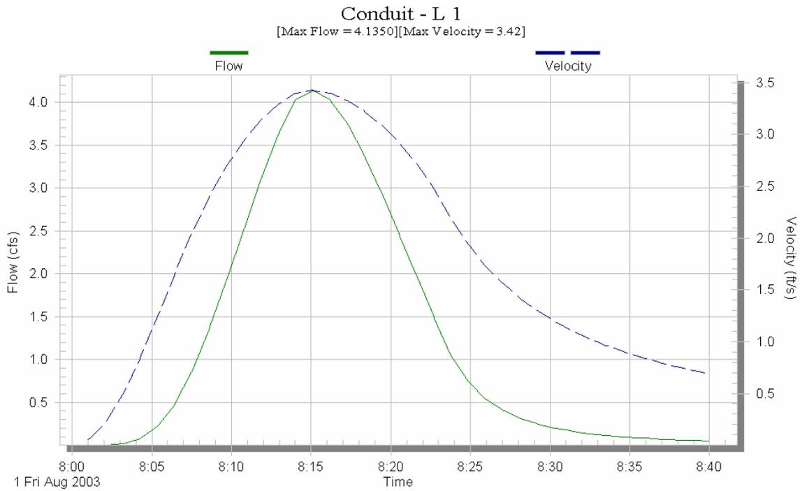
Figure D.13. Time series plot of flows and velocity by SWMM for conduit L1.
