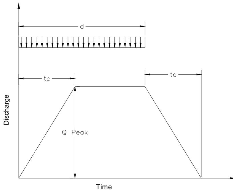
Figure 2.2(a) Hydrograph when duration of rainfall is greater than  $t_c$ .
