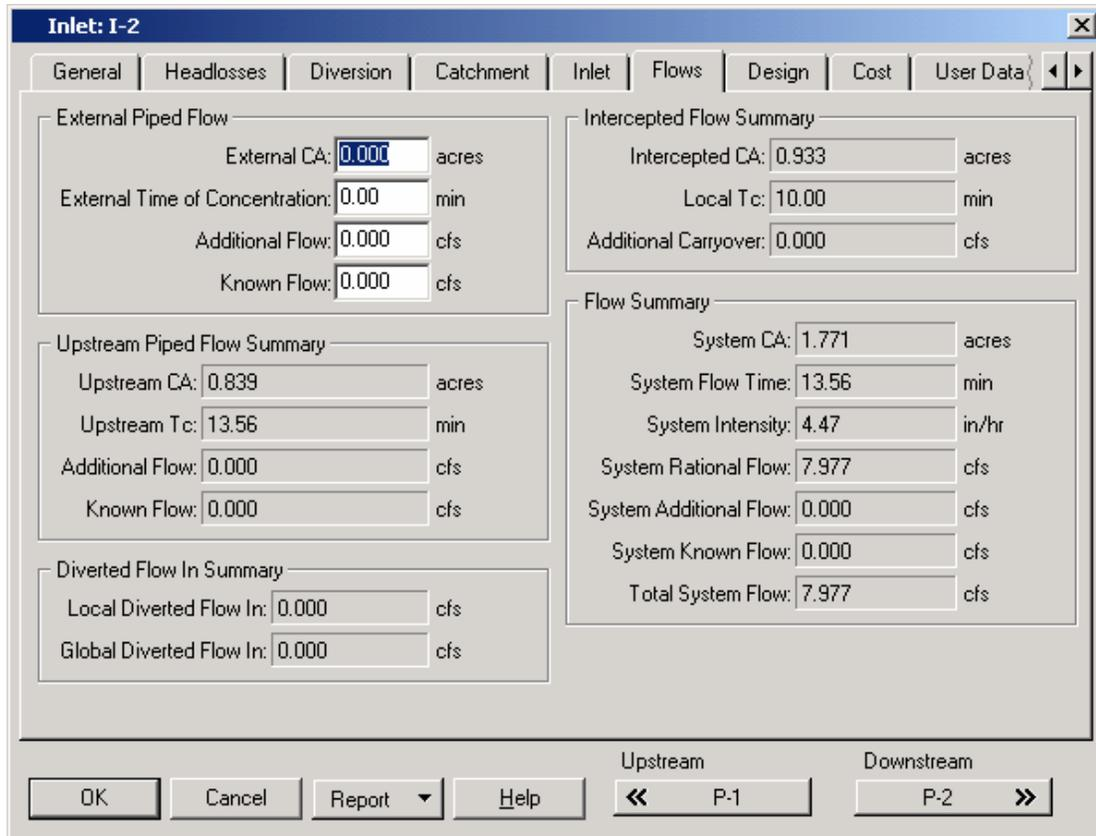
Figure A.8 Flow simulation results for Inlet I-2.
