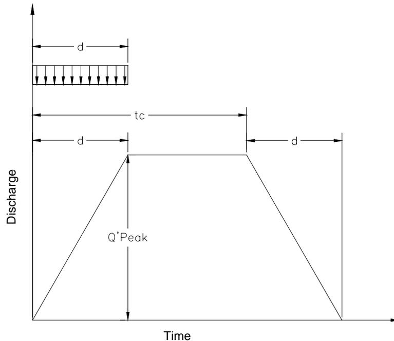
Figure 2.2(c) Hydrograph when duration of rainfall is less than  $t_c$ .
