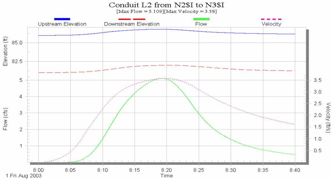
Figure D.24 Time series output of flow, velocity and elevation for conduit L2 resulted from Extran layer of SWMM for a maximum interception capacity of 3.0 cfs for inlet.
