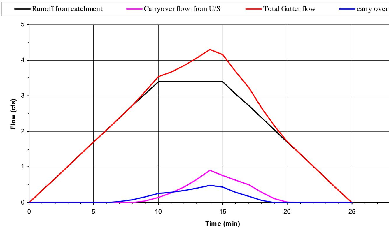
Figure C.5. Simulated **surface flow** components at the inlet I-3 (node 3) by using modified SPLIT program.
