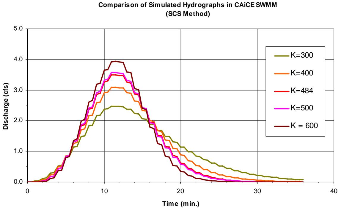
Figure D.31a. Simulated hydrographs using SCS Method in CAiCE SWMM.
