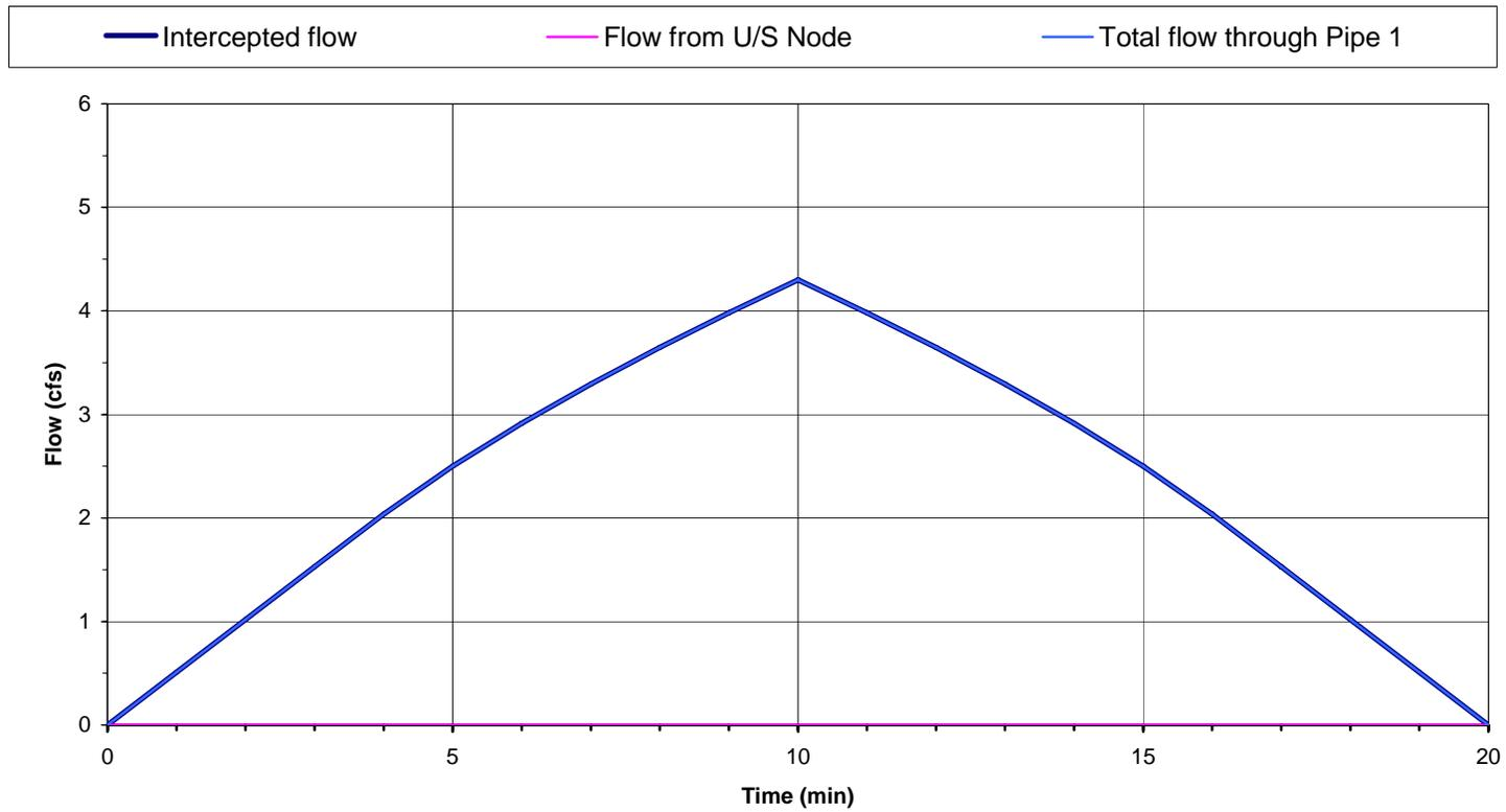
Figure C.2. Simulated **subsurface flow** components at the inlet I-1 (node 1) by using modified SPLIT program.
