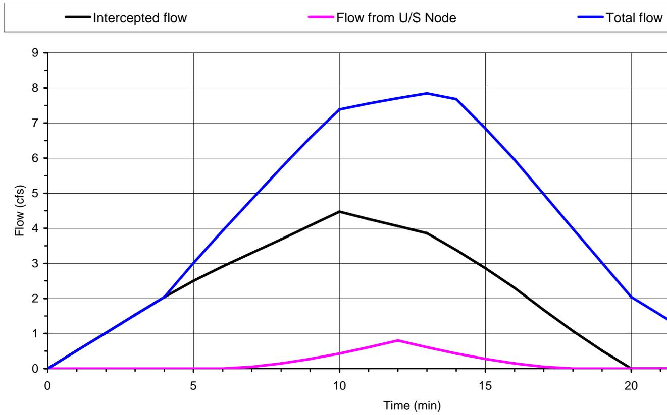
Figure C.4 Simulated **subsurface flow** components at the inlet I-2 (node 2) by using modified SPLIT program.
