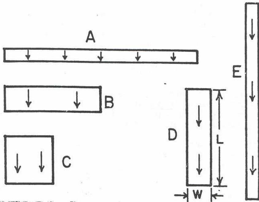
Figure D.6a. Different sub-catchment shapes to illustrate effect of sub-catchment width (Huber, 1988.)
