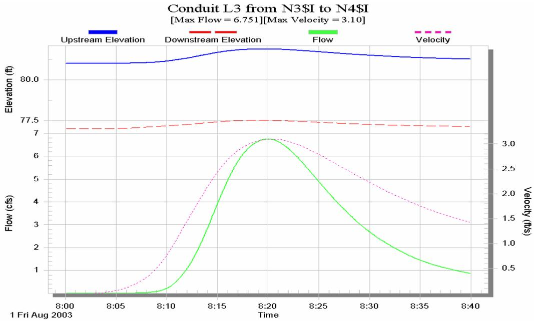
Figure D.36. Time series output from SWMM for conduit L-3.
