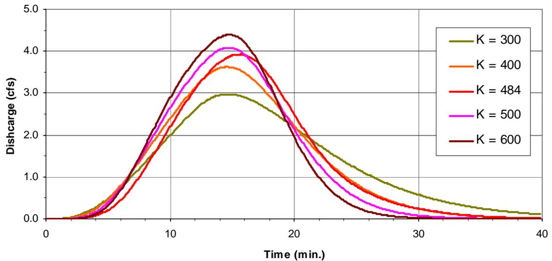
FigureD.31b. Simulated hydrograph using SCS Method in XP SWMM.
