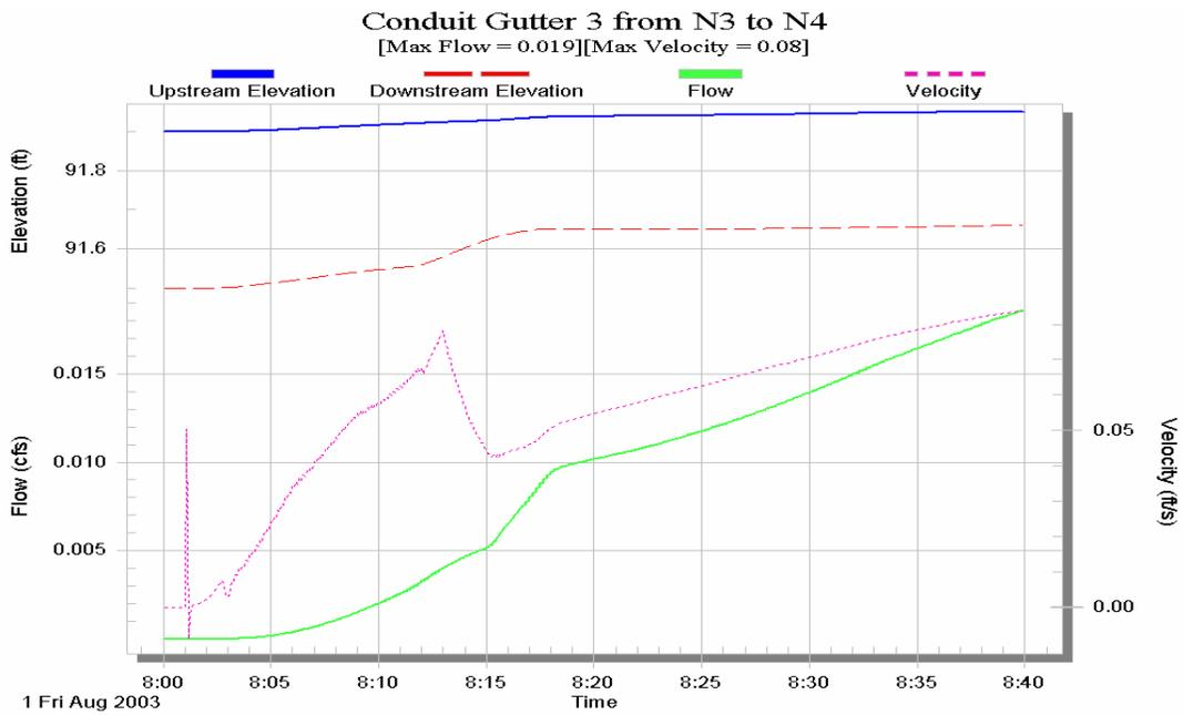
Figure D.37. Time series output from SWMM for conduit Gutter 3.
