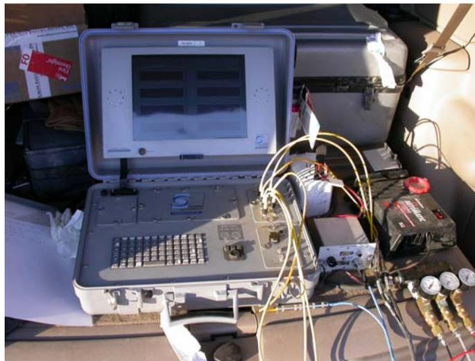
**Figure 1** Freedom Data PC Used Sonic Echo Testing
