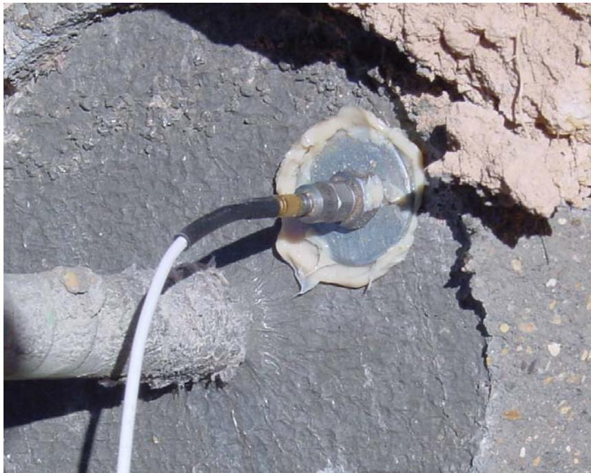
**Figure 3** Accelerometer Attached to Washer on the Grout
