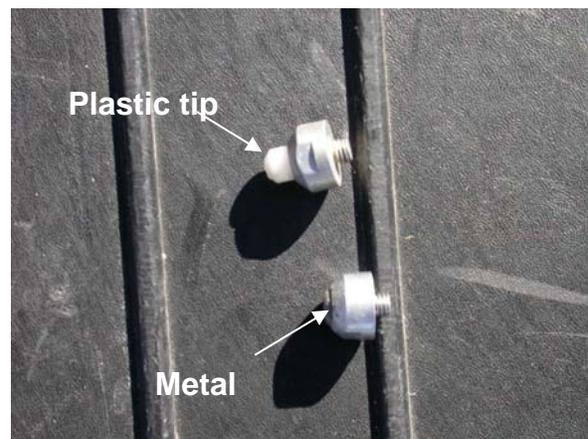
**Figure 2** Instrumented Hammer with Interchangeable Metal/Plastic Tips
