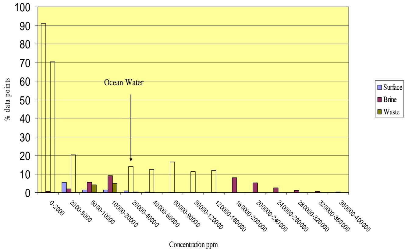
**Figure 2.2 Chart for TDS Concentration Distribution in Alternate Water Sources.**
