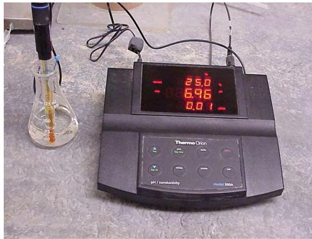
**Figure 4.2 Soil pH Measurement by Tex-128-E Test Procedure**
