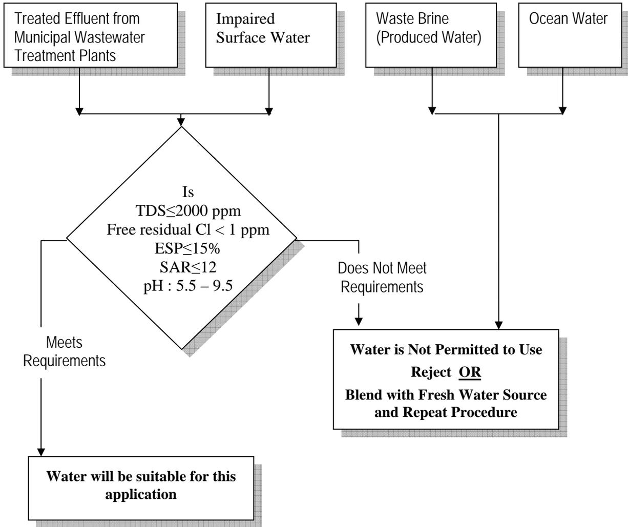
**Figure 6.8** - Stage II Decision Matrix for Water Used for Irrigation
