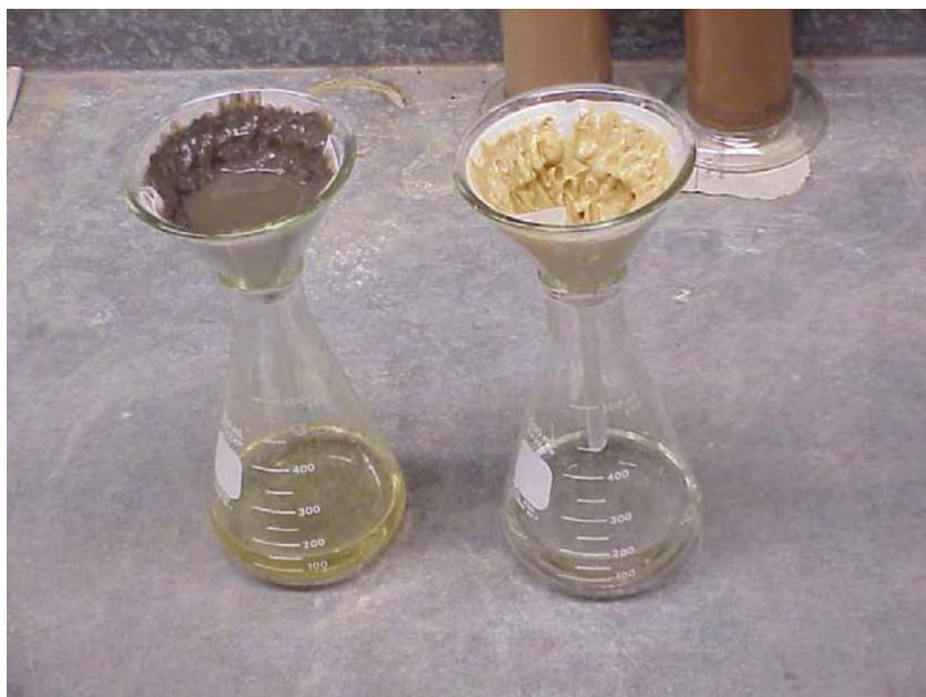
**Figure 4.4 Filtering Process in Soil Sulfate Content Testing**
