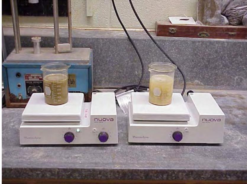
**Figure 4.3 Heating Process in Soil Sulfate Content Testing**
