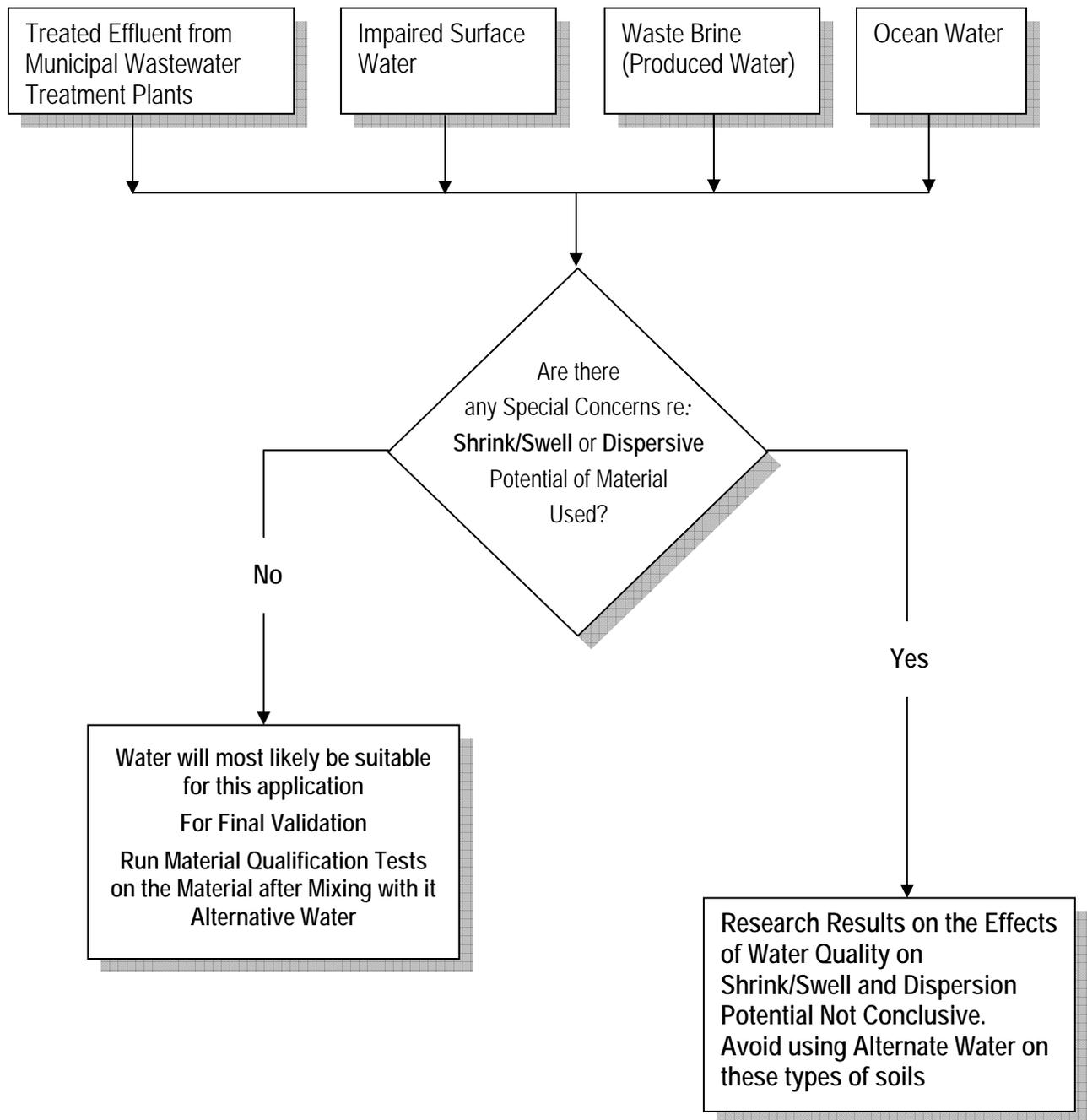
**Figure 6.7** - Stage II Decision Matrix for Water Used in the Compaction of Road Subgrades, Flexible Base Courses and Embankment Fill
