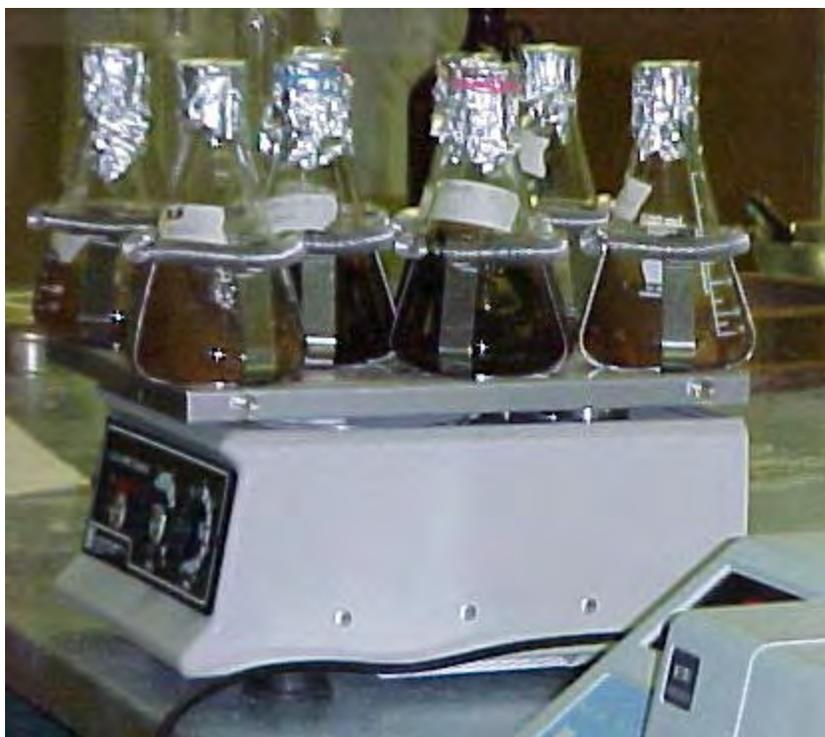
Figure 1. Mechanical Shaker
