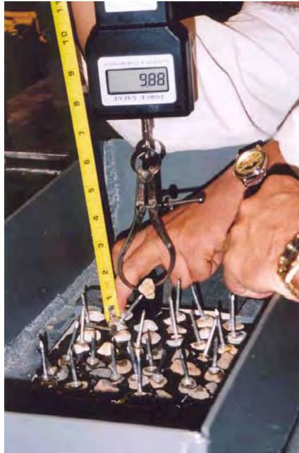
**Figure 6-5** Aggregate Pull-Out using Force Gage
