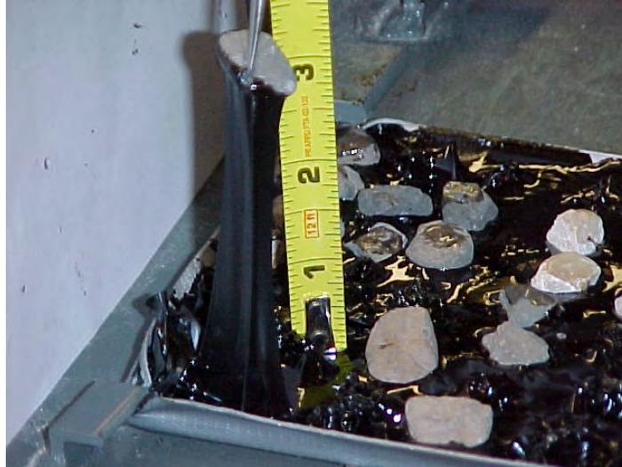
**Figure 6-7** Elongation due to Aggregate Pull-Out
