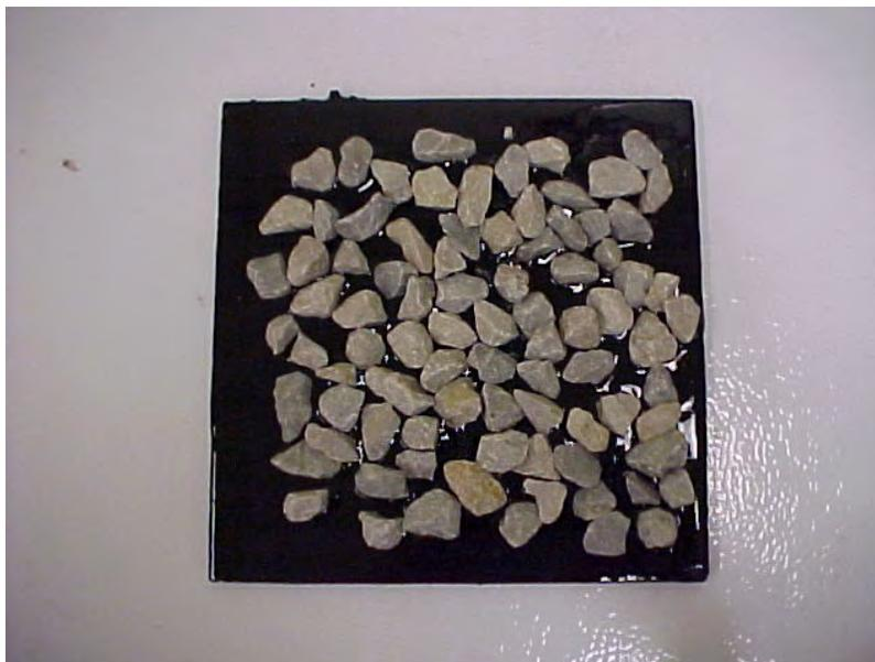
**Figure 3-4** Typical Seal Coat Specimen Collected from the Field
