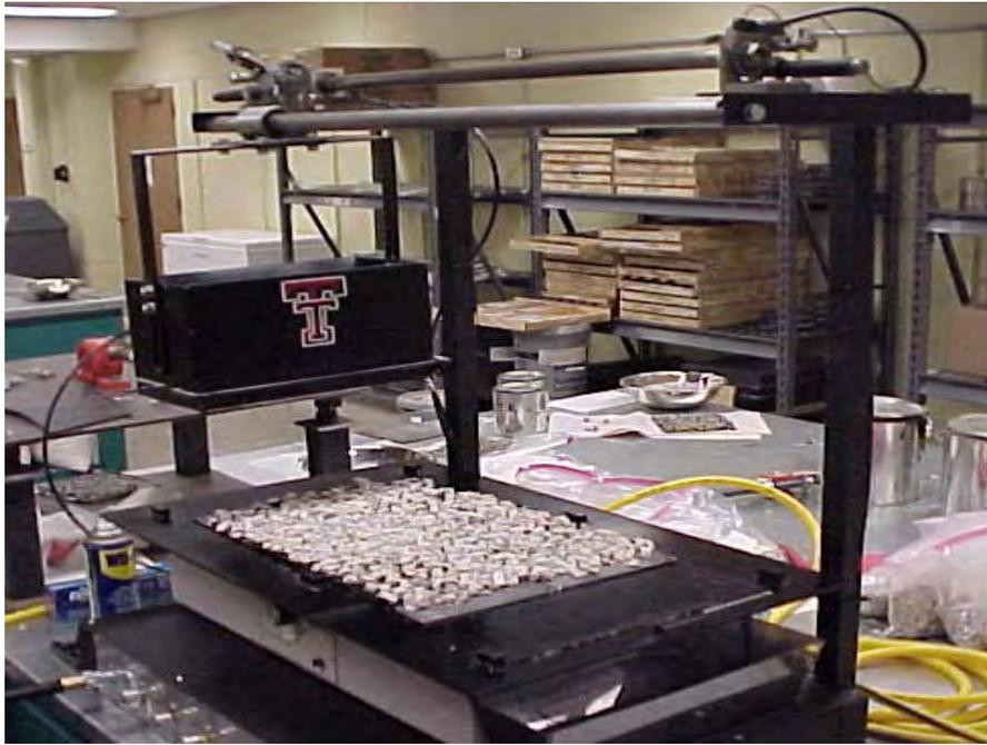
**Figure 1. Automated Chip Spreader used in Research Project 0-4362**
