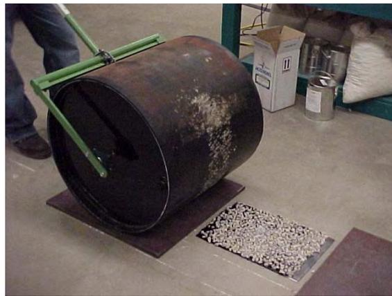
**Figure 5-1** Specimen Compaction Using the Laboratory Roller
