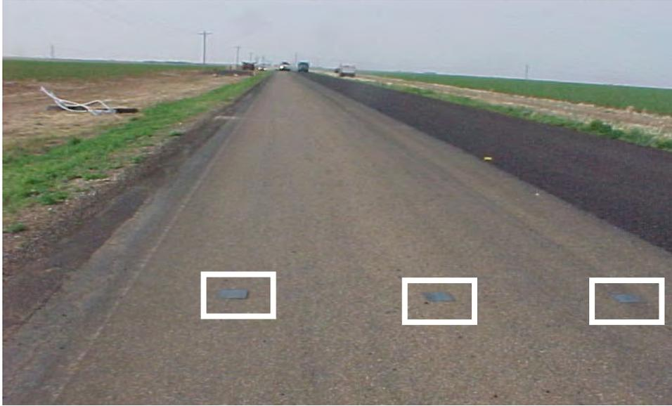
**Figure 3-3** Collection of Field Specimens at Test Projects (Insert Shows Specimen Plates Placed on Existing Pavement)
