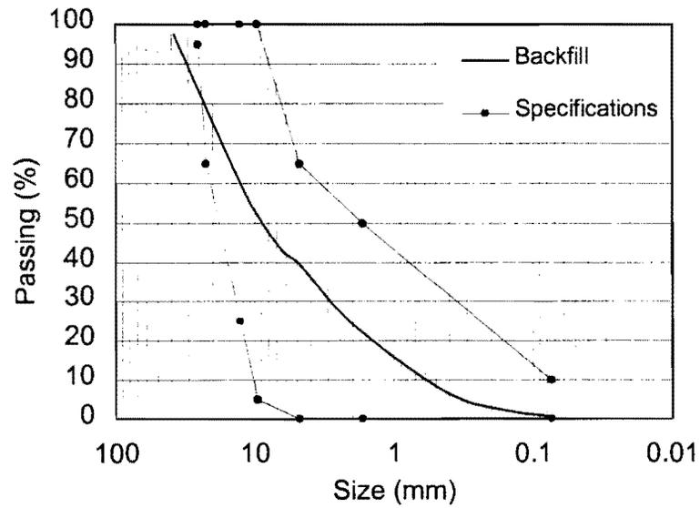
**Figure 5.43** Particle Size Distribution of Yoakum Backfill.
