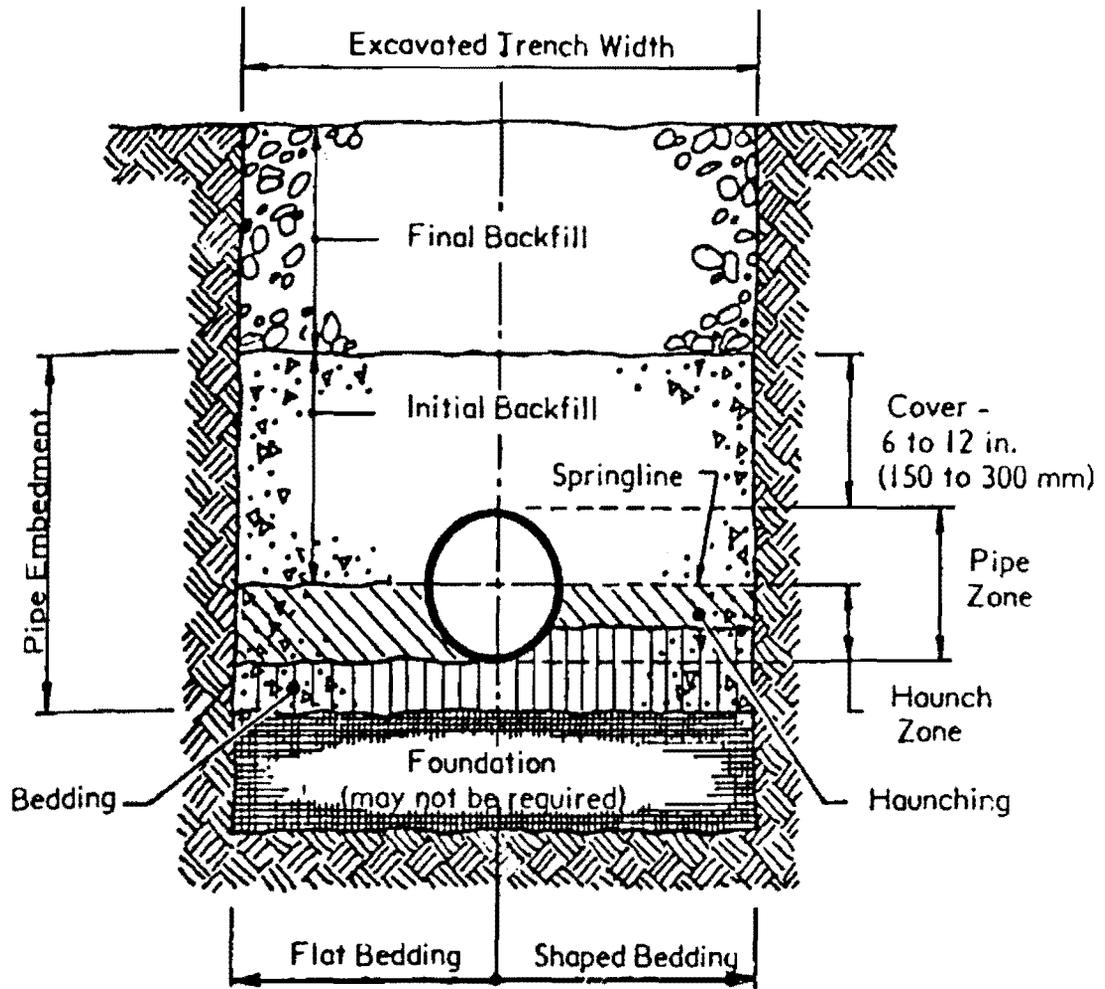
Figure 2.1. Typical Cross Section of Trench Installation (5).
