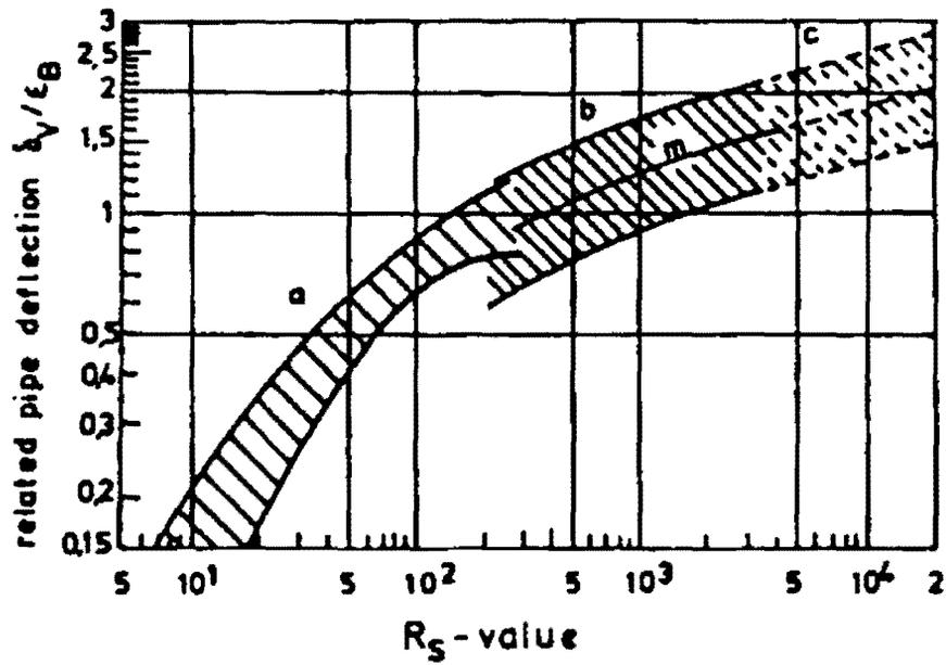
Note: a- range of flexible steel pipes, b-range of PVC and PE pipes, c-extrapolated range, m- mean curve
