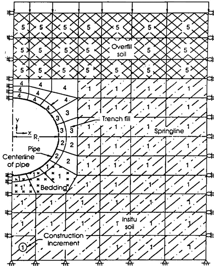
Figure 8.3. A Finite Element Mesh Used in the Analysis (49).
