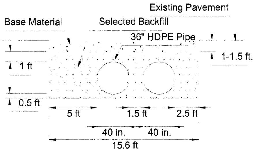
**Figure 5.29** Cross-Section of Installation A2 in Atlanta District.
