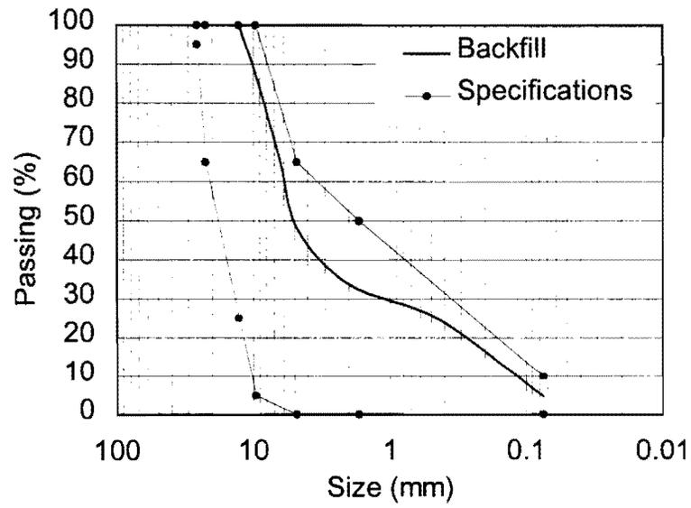
**Figure 5.19** Particle Size Distribution of Backfill in Laredo.
