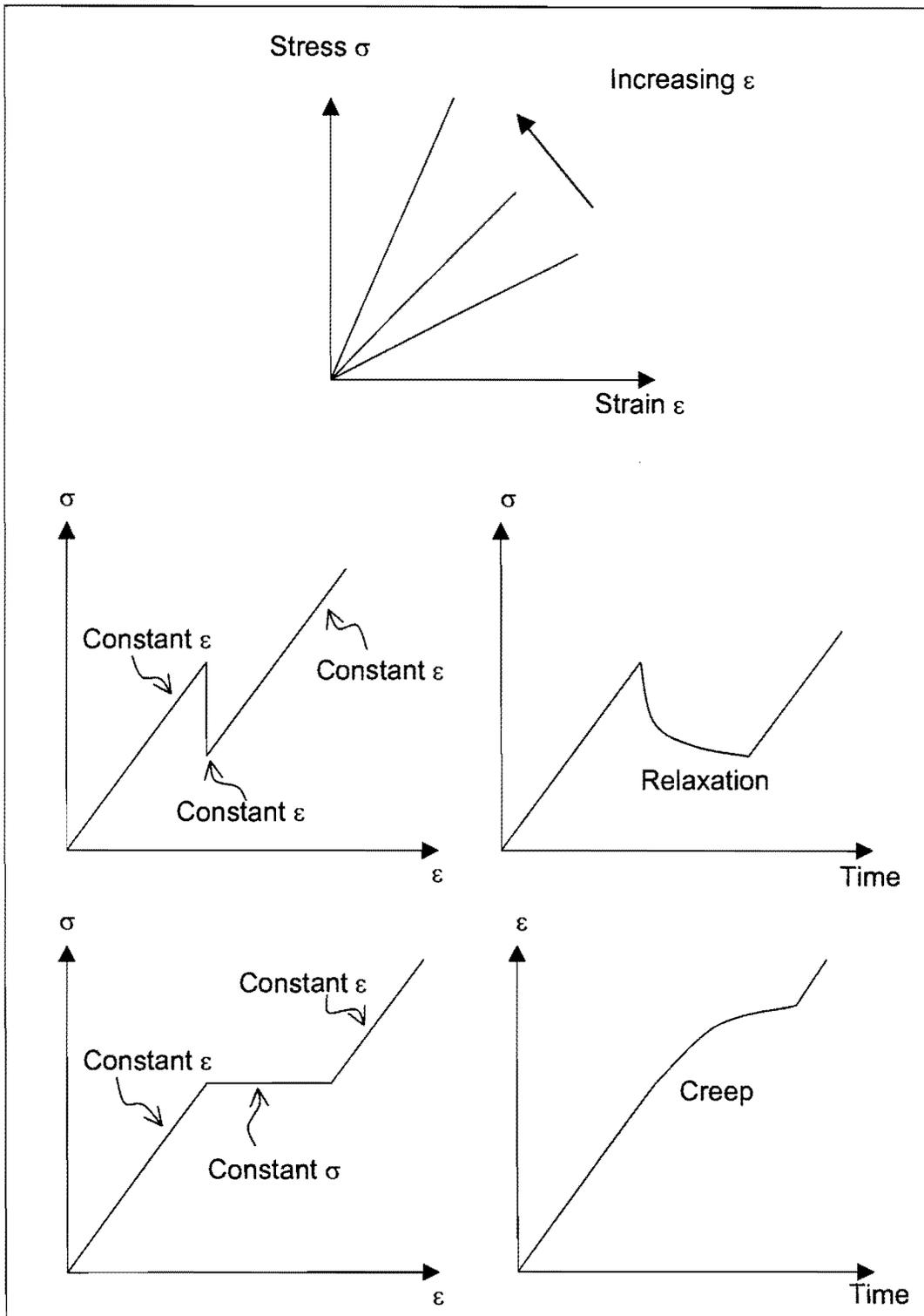
Figure 2.3. Characteristics of Linear Viscoelastic Materials (12)
