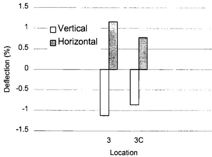
**Figure 5.18** Pipe Deflections after Installation in Laredo.
