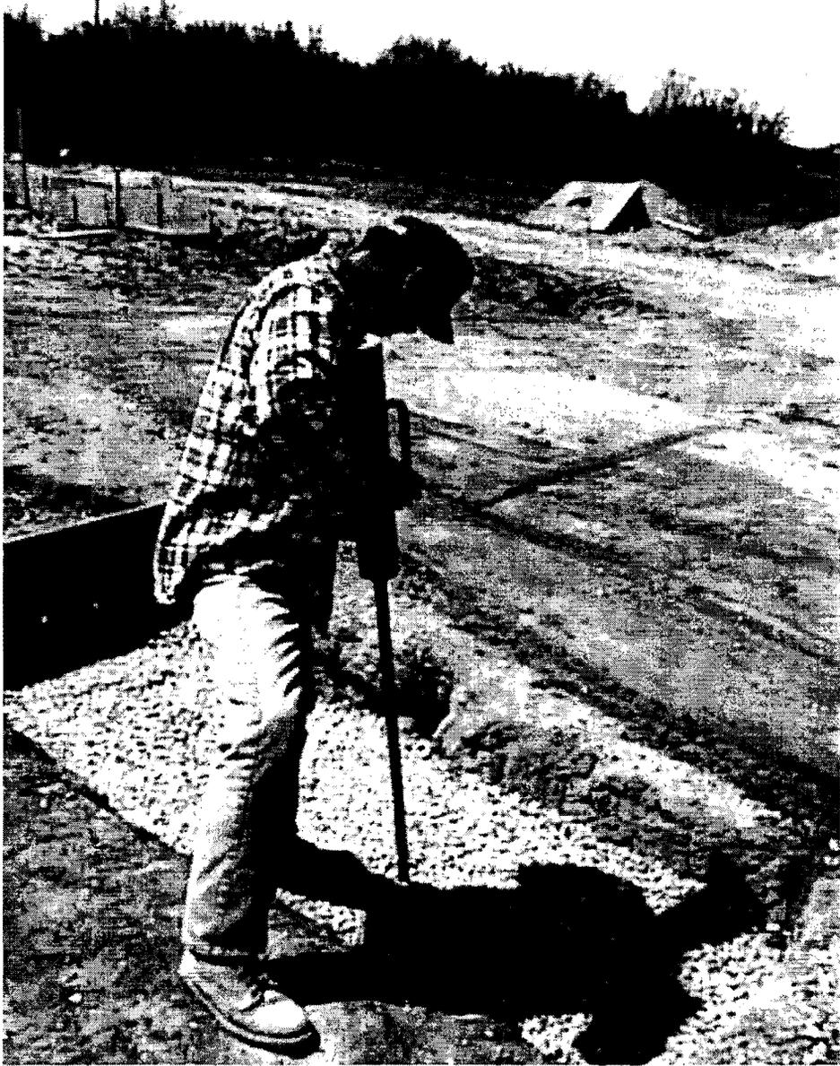
**Figure 4.4.** The Dynamic Cone Penetrometer Being Operated.
