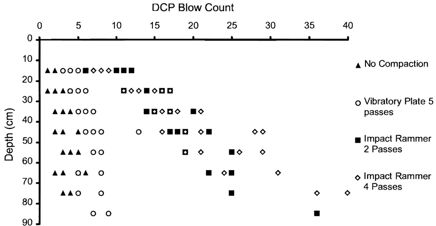
Figure 4.7. DCP Blow Count Profiles for Gravelly Sand.
