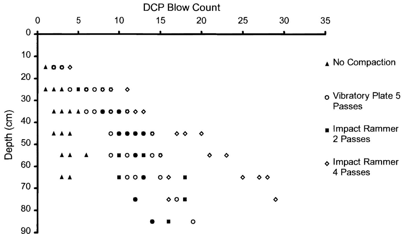
Figure 4.6. DCP Blow Count Profiles for Medium Gravel.
