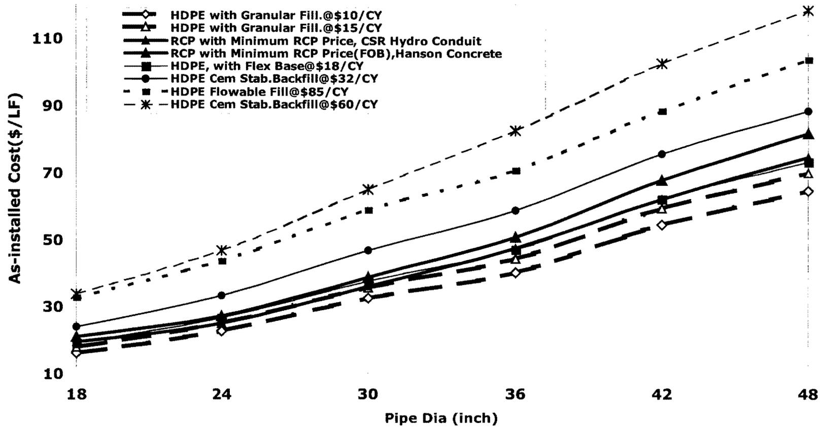
Figure 7.5. Estimated As-installed Cost of HDPE versus As-installed Cost of RCP
