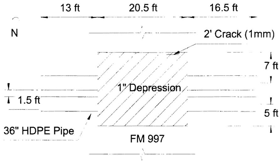
**Figure 5.36** Pavement Settlement at Installation B in Atlanta District.
