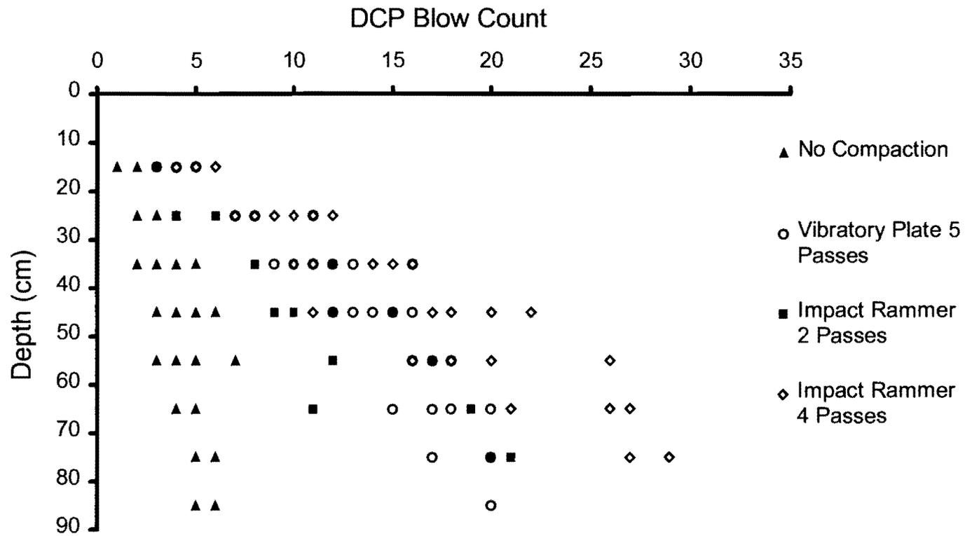
Figure 4.5. DCP Blow Count Profiles for Coarse Gravel.
