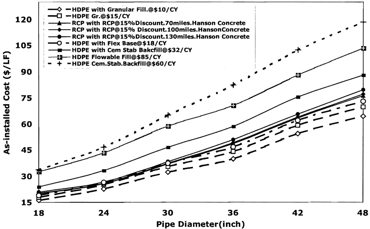
Figure 7.4. Estimated As-installed Cost of HDPE versus As-installed Cost of RCP
