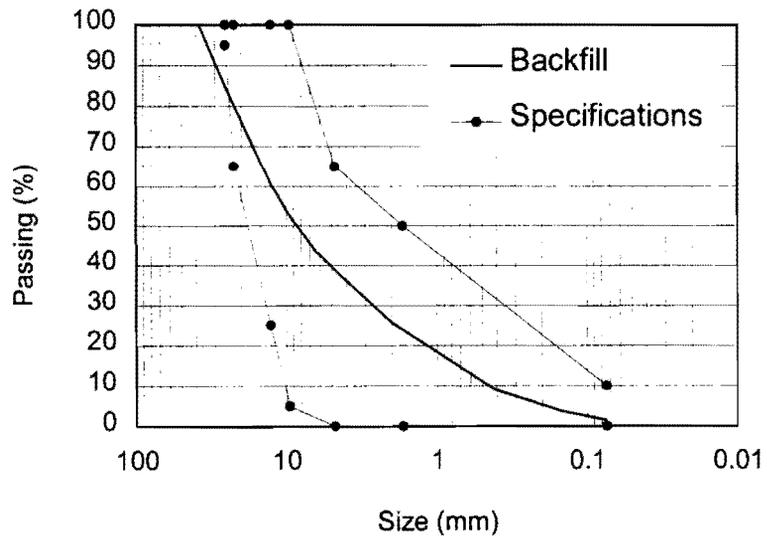
**Figure 5.31** Particle Size Distribution of Atlanta Backfill.
