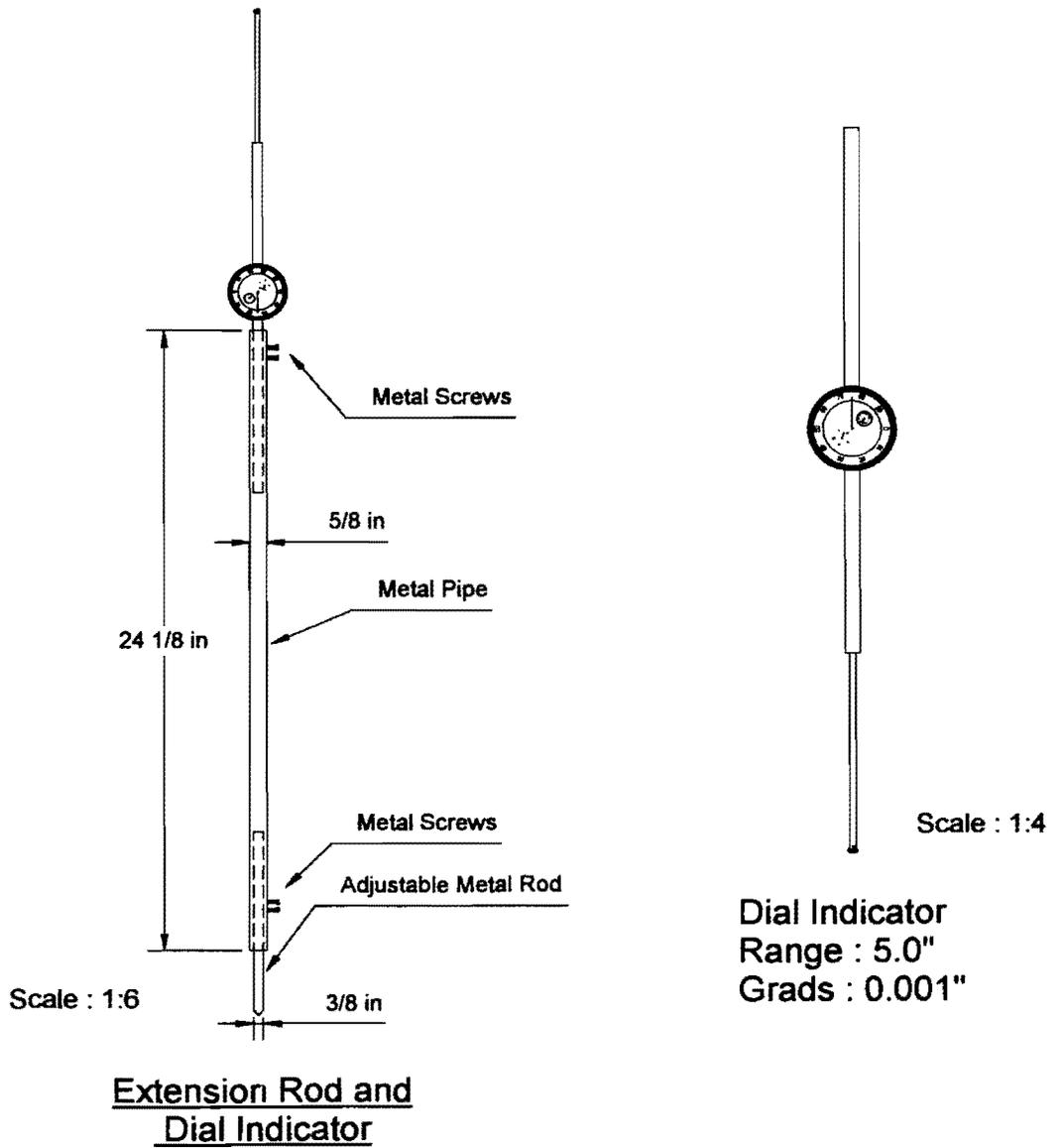
Figure 4.14. The Deflectometer.
