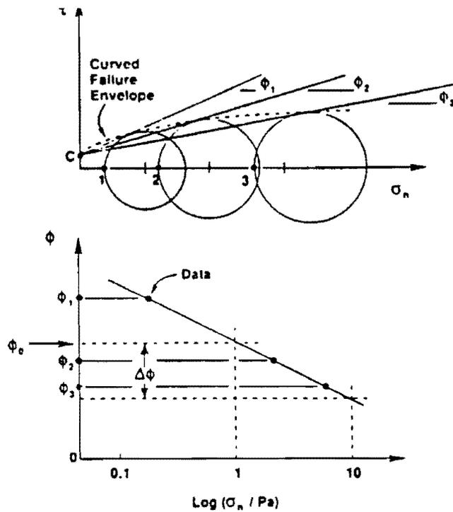
Figure 8.2. The Calculation of the Modified (1).
