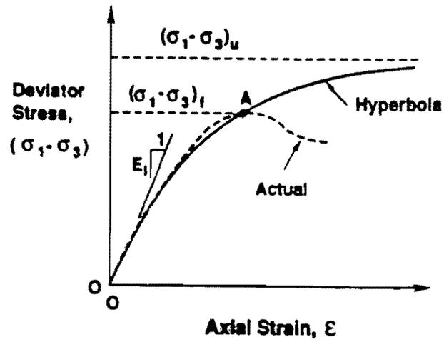
Figure 8.1. The Calculation of  $R_f$  (1).
