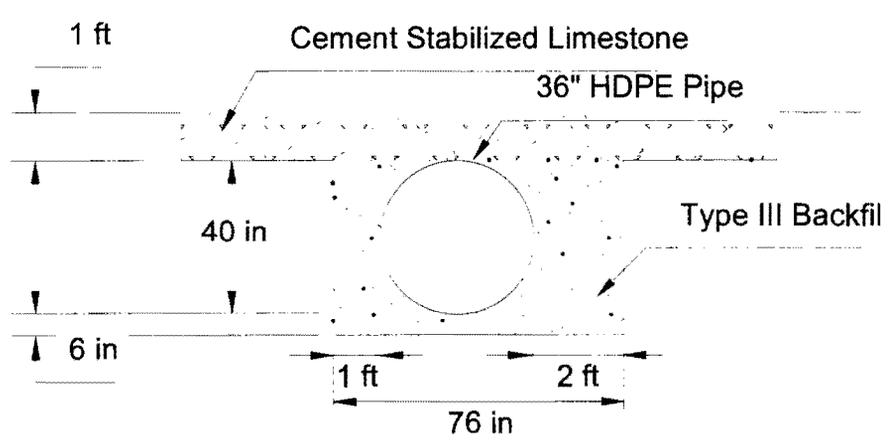
**Figure 5.39** Cross-Section of Installation Y1 in Yoakum District.
