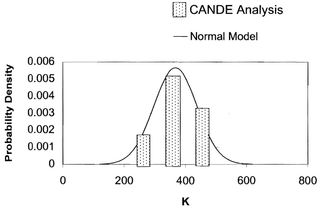
**Figure 8.6.** Variation of K Back Calculated from CANDE for Backfill with Low Compaction in Comparison with a Normal Model.
