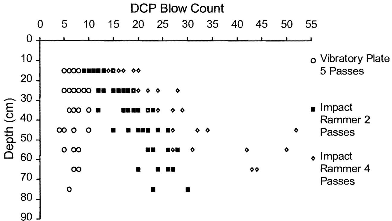
Figure 4.8. DCP Blow Count Profiles for Clayey Sand.
