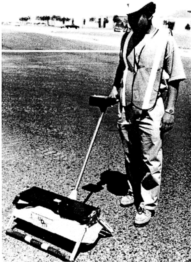
Figure 3.7 Pavement Macrotexture Measurement Using a Mini Texture Meter
