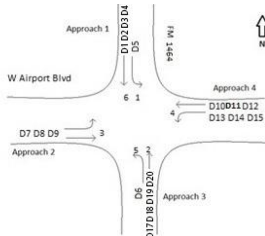
Figure 2.2.19 Specification of approaches, phases, and detectors of the intersection at W. Airport Blvd.
