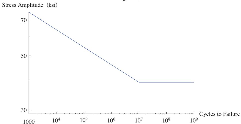
**Figure 7.10. Approximate S-N Diagram, HPS Steel.**
