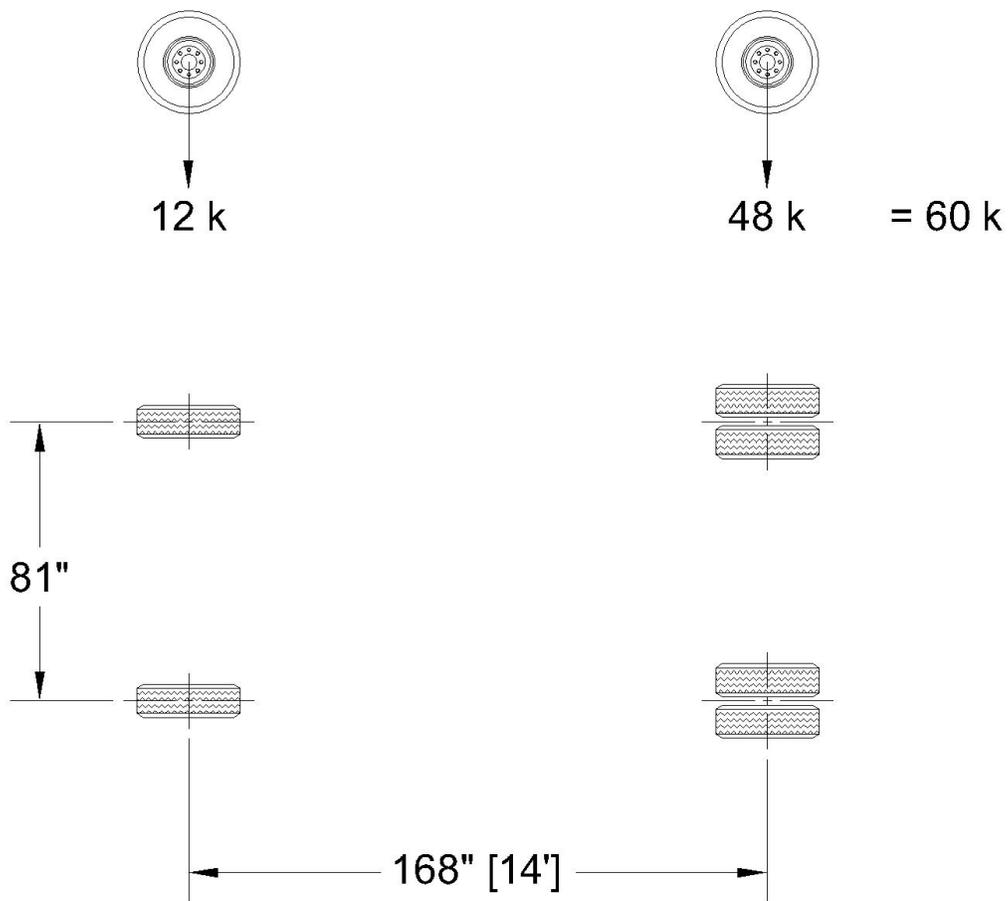
**Figure 4I-1. 2 Axle Single (2AS) Unit Loading.**
