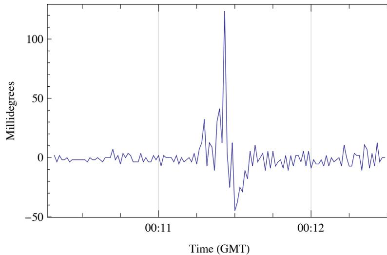
**Figure 5.3. Bridge Response to Type 3 AASHTO Load.**
