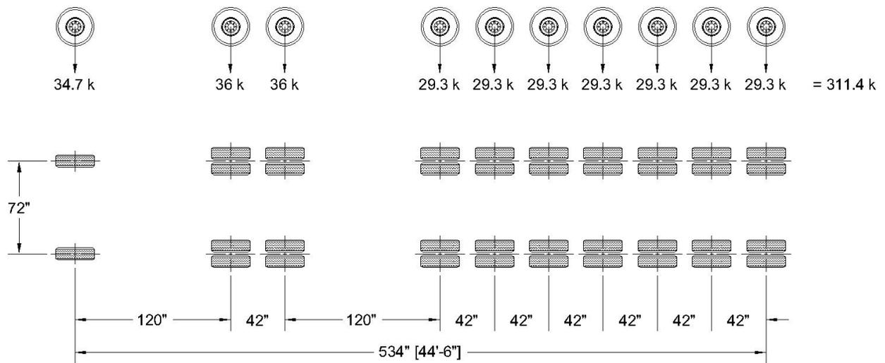
**Figure 4R-1. 10 Axle Combination (10AC) Unit Loading.**
