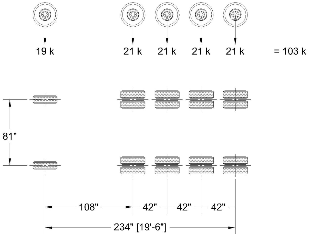
Figure 4N-1. 5 Axle Single (5AS) Unit Loading.
