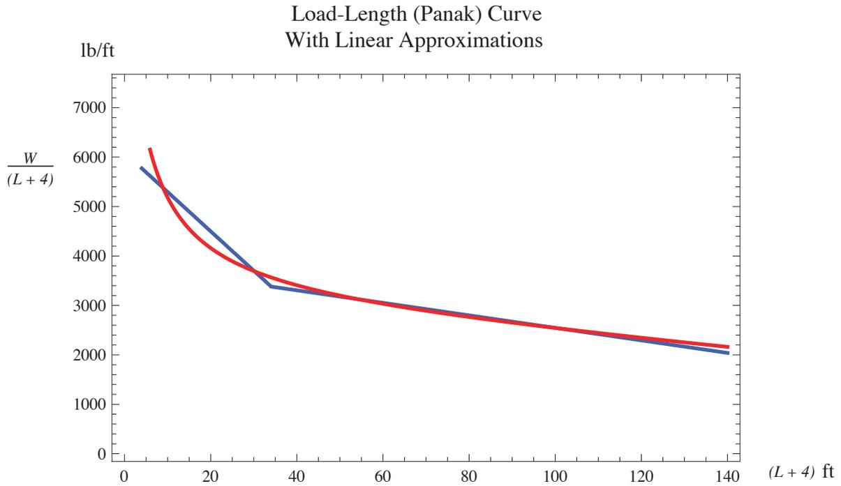
**Figure 8.5. Load-Length Graph with Piecewise Linear Fits.**
