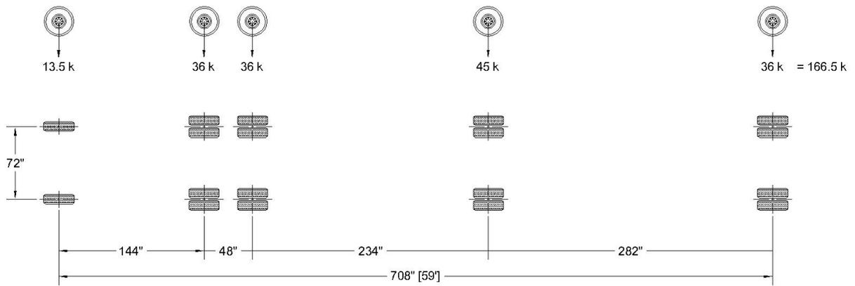
Figure 4M-1. 4 Axle Combination (5AC) Unit Loading.
