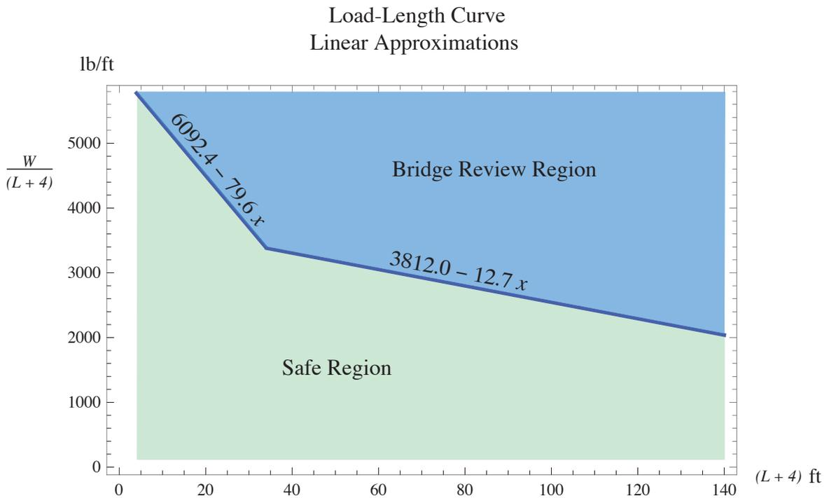
**Figure 8.6. Suggested TxDOT Graphical Superheavy Load Criteria.**
