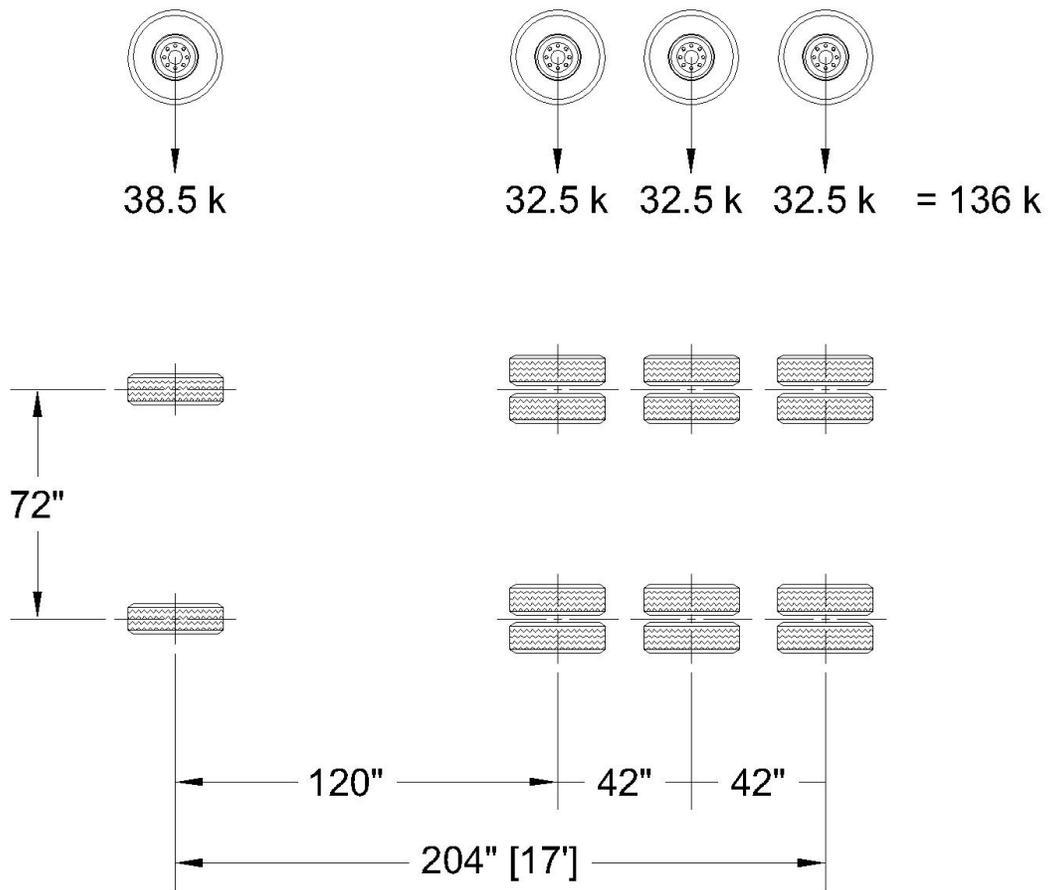
Figure 4T-1. Tridem Axle Single (TAC) Unit Loading.
