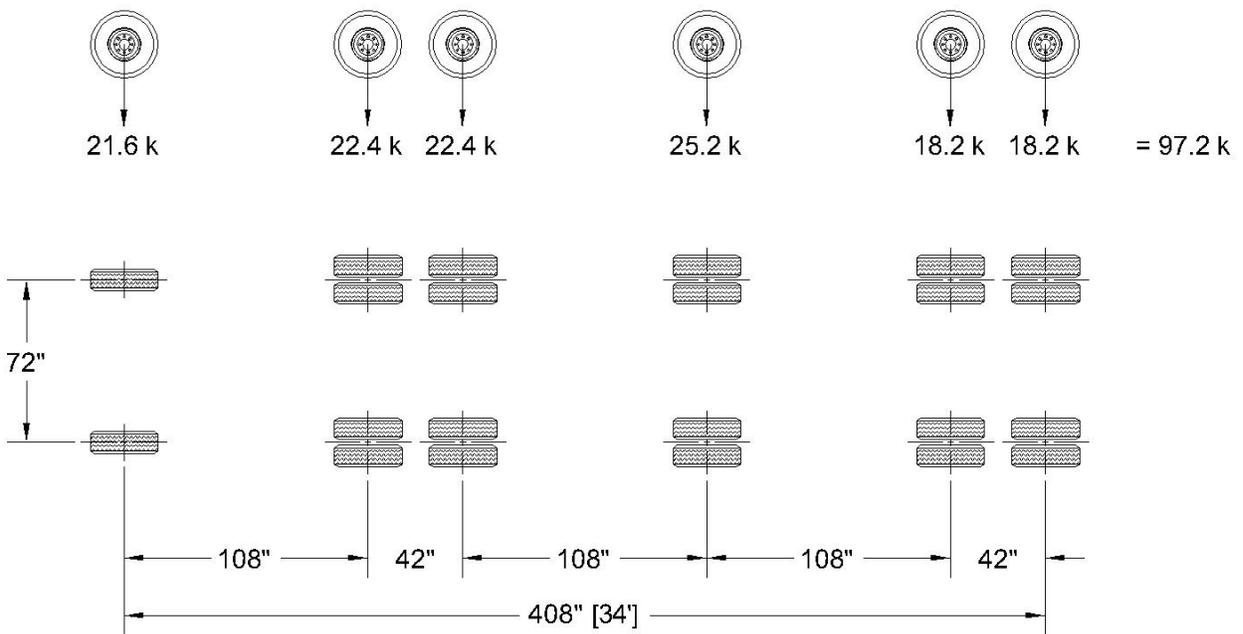
Figure 40-1. 6 Axle Combination (6AC) Unit Loading.
