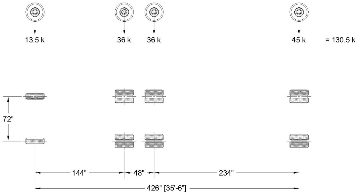
Figure 4K-1. 4 Axle Combination (4AC) Unit Loading.
