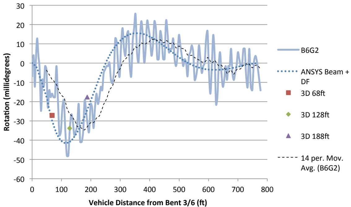
**Figure 4.18. Comparison of Interior Girder Rotation at Bent 6.**
