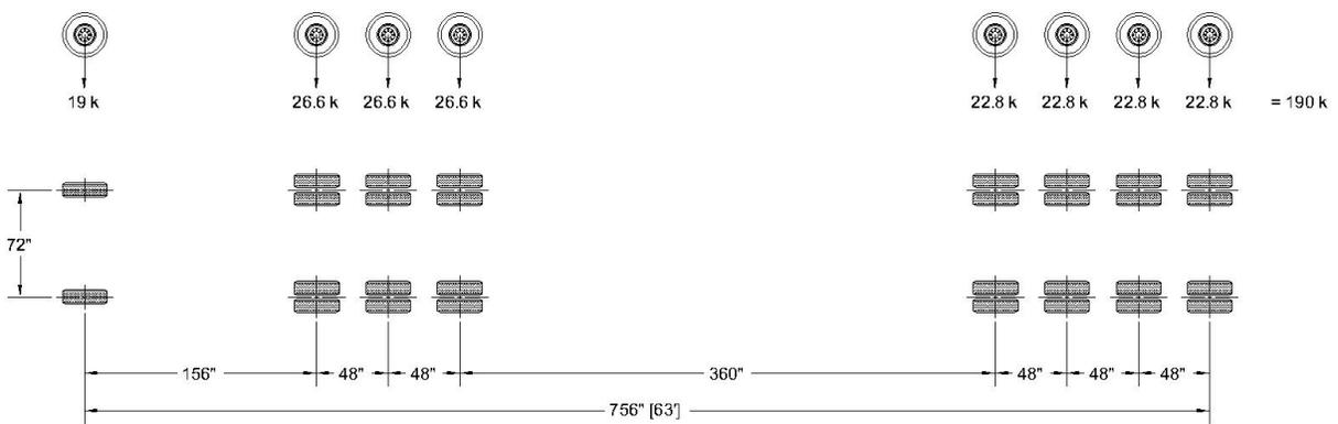
Figure 4F-1. 8 Axle Combo (8AC) Unit Loading.
