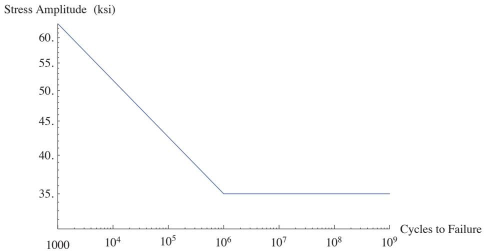
**Figure 7.9. Approximate S-N Diagram for 70-ksi Steel.**
