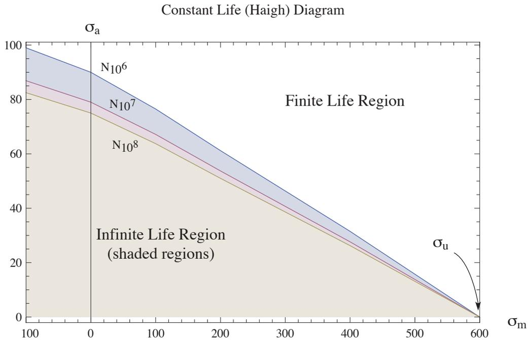
**Figure 7.8. Constant Life Diagram for a Particular Material.**
