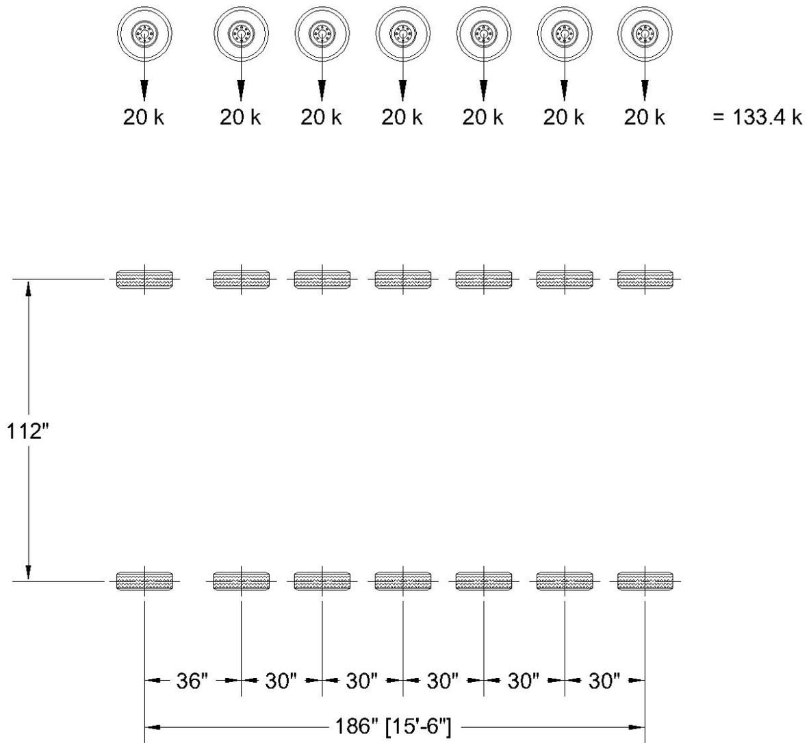
Figure 4Q-1. 7 Axle Single (7AS) Unit Loading.
