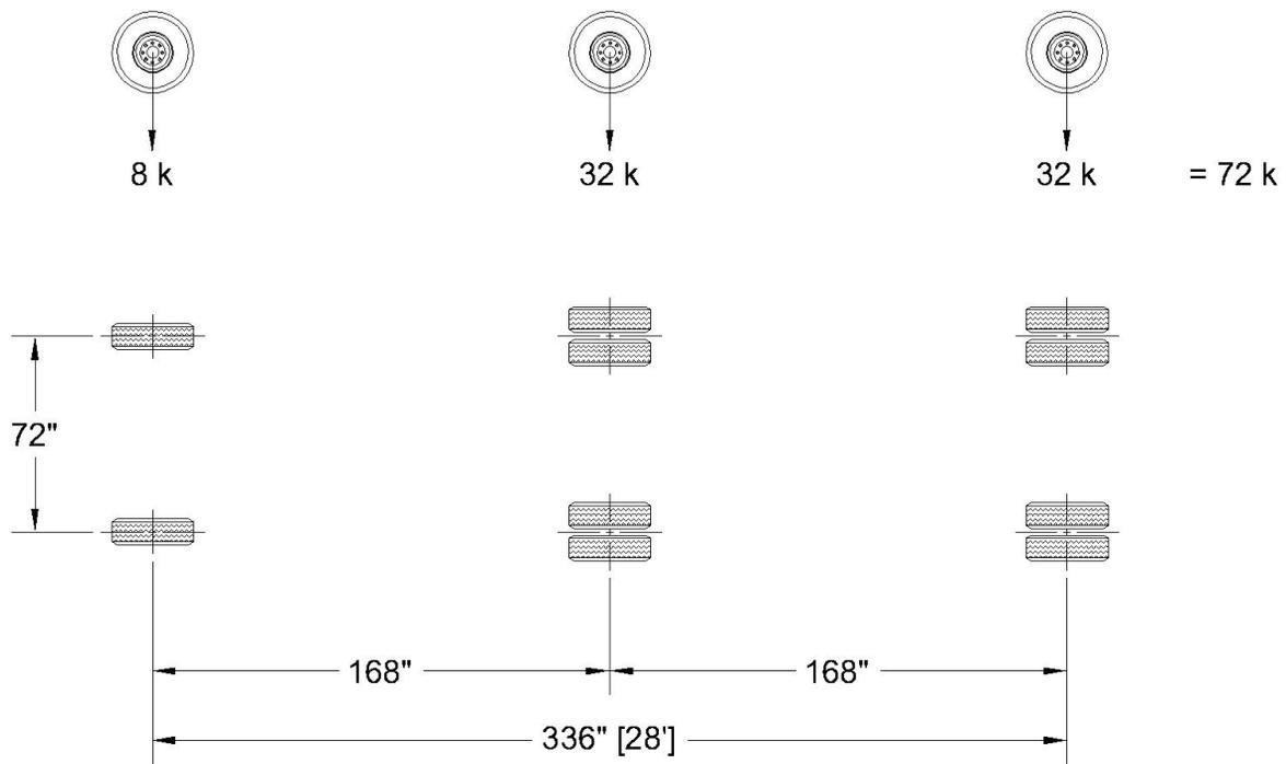
Figure 4E-1. 3 Single Axle Combo (3SAC) Unit Loading.
