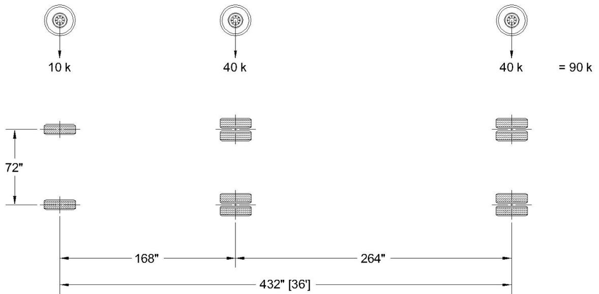
Figure 4J-1. 3 Axle Combination (3AC) Unit Loading.
