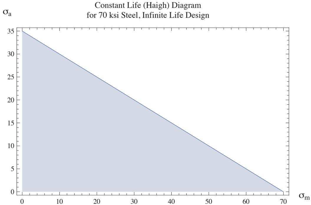
**Figure 7.11. Constant Life Diagram, 70 ksi Steel.**
