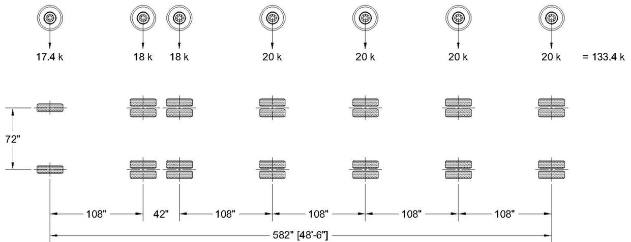
**Figure 4P-1. 7 Axle Combination (7AC) Unit Loading.**
