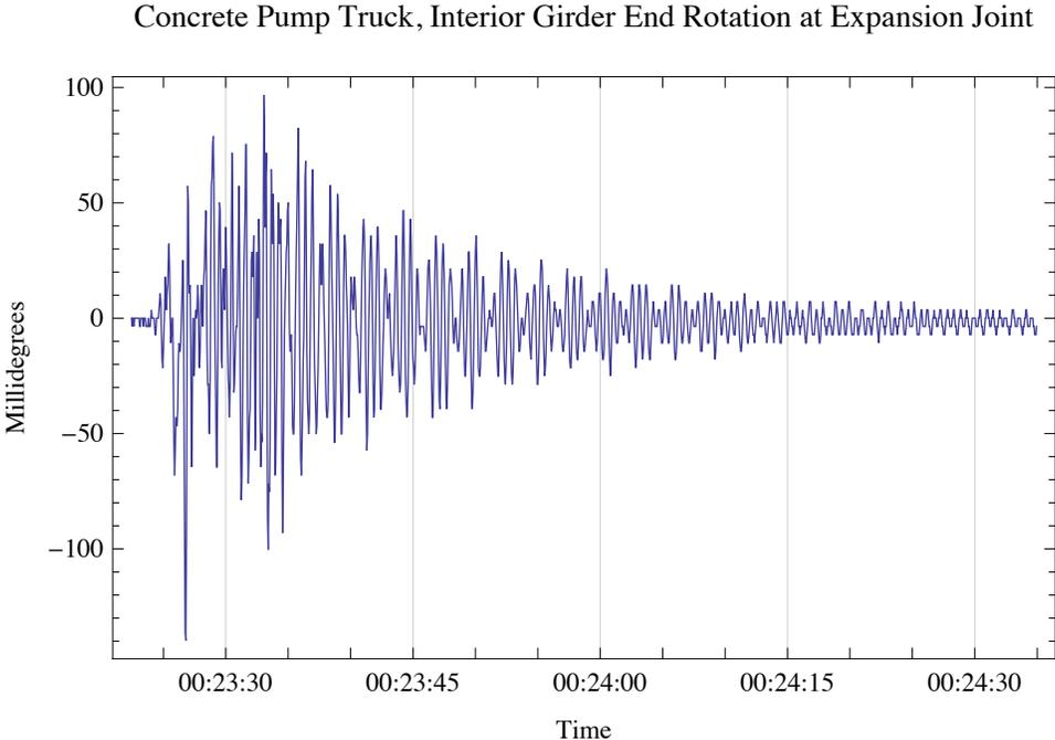
**Figure 5.4. Bridge Response with 20 Samples per Second Rate.**
