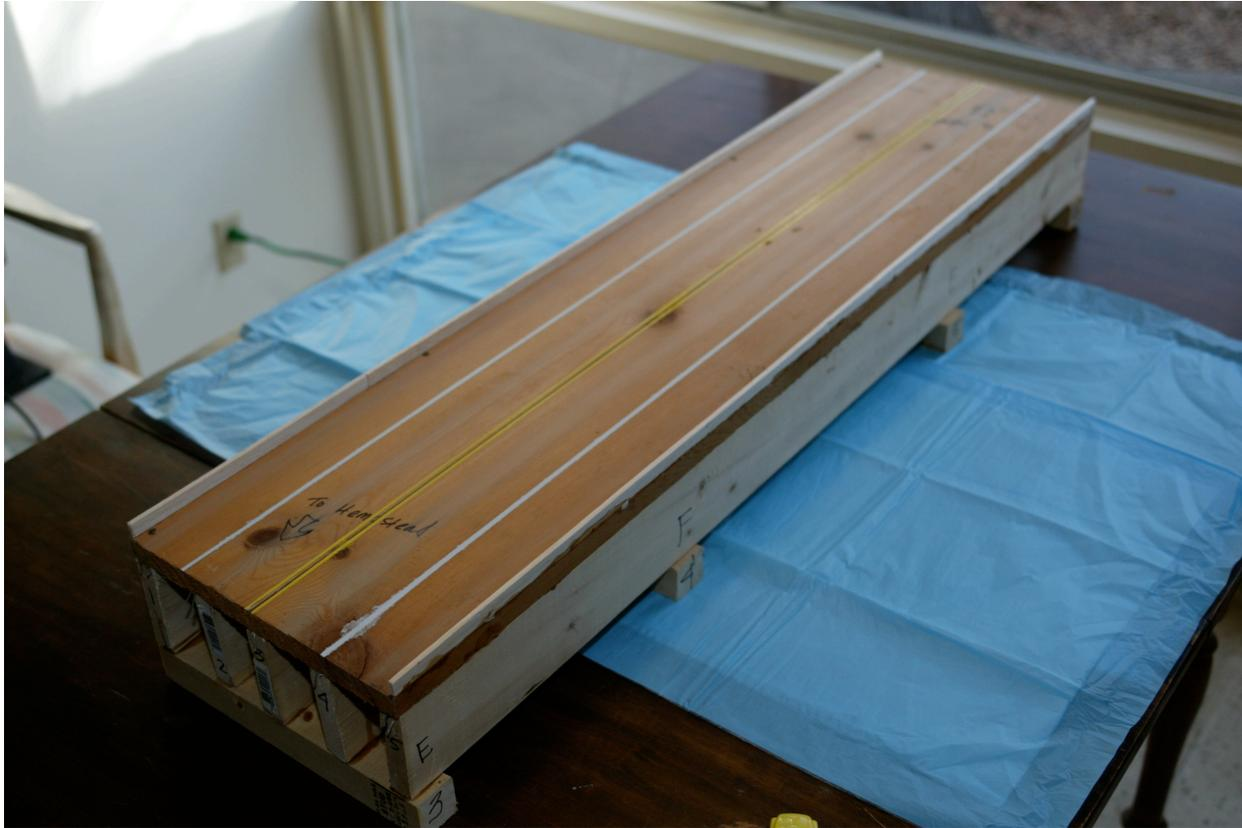
**Figure 5.22. Functional Model of Steel Girder Unit for Load Application.**
