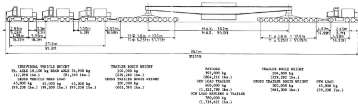
Figure 1.1. Abnormal Load Haulers and Trailer from Boulet (1977).
