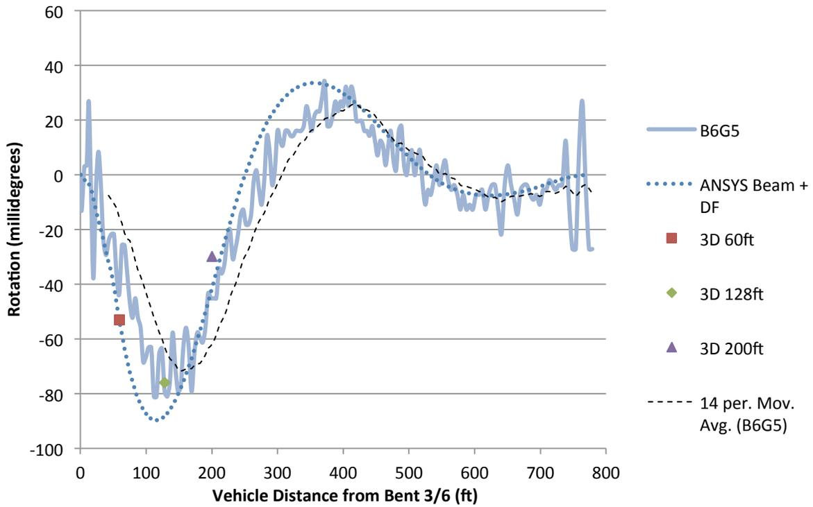
**Figure 4.17. Comparison of Exterior Girder Rotation at Bent 6.**
