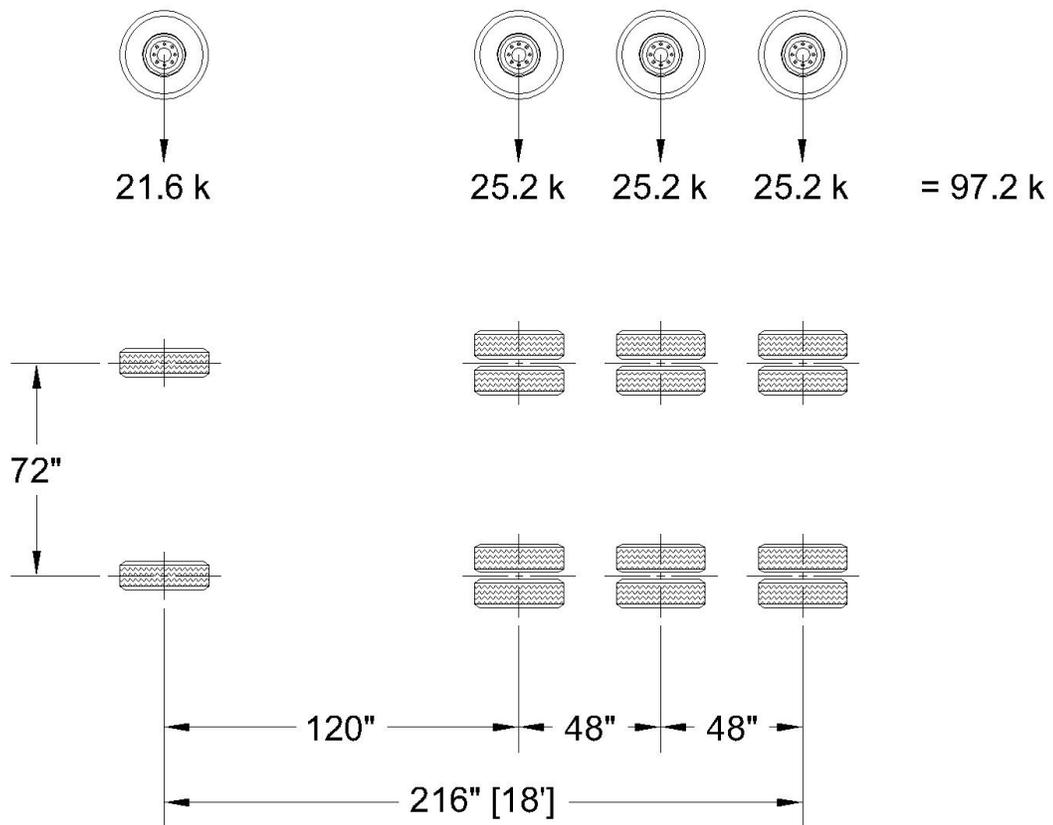
Figure 4L-1. 4 Axle Single (4AS) Unit Loading.
