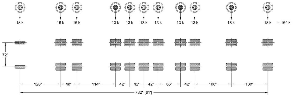
Figure 4S-1. 11 Axle Combination (11AC) Unit Loading.
