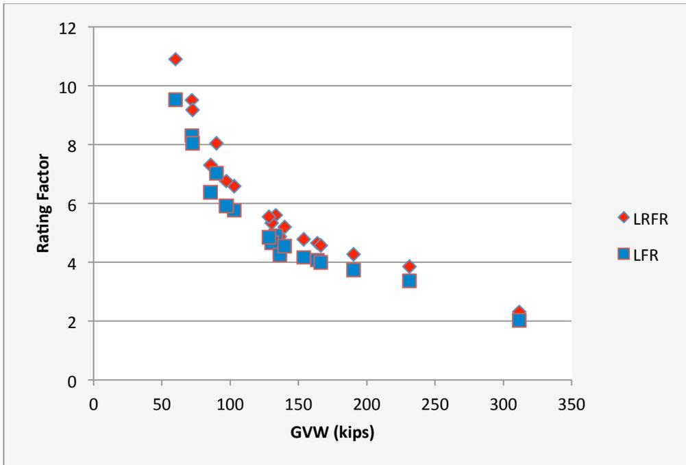
**Figure 6.2. Rating Factor vs. Gross Vehicle Weight.**
