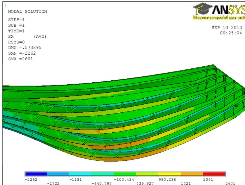
**Figure 4.16. Deflected Bridge Displaying Stress Magnitudes.**
