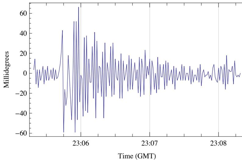
**Figure 5.2. Bridge Response to 3S2 AASHTO Load.**
