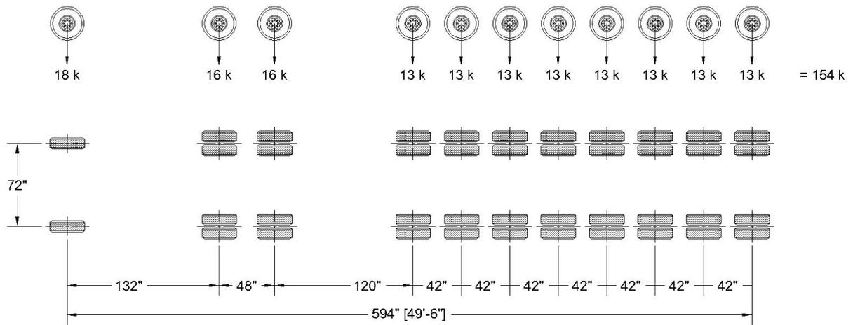
**Figure 4D-1. 11 Axle Combo Spacing (11ACS) Unit Loading.**
