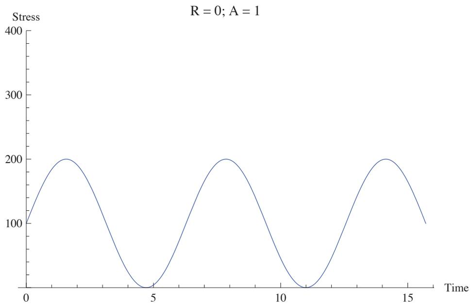
**Figure 7.5. Case 2, Zero to Maximum,  $R=0$  and  $A = 1$ .**
