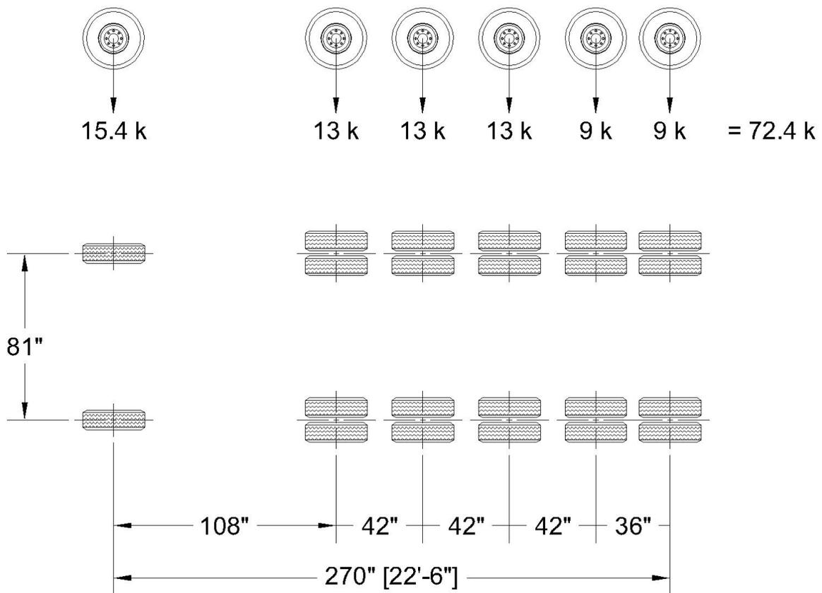
**Figure 4H-1. 5 Axle Single Group (5ASG) Unit Loading.**
