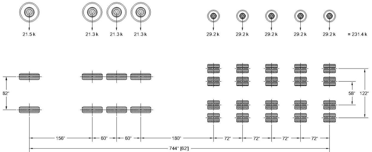
**Figure 4A-1. Heavy Equipment Transport System (HETS) Loading.**
