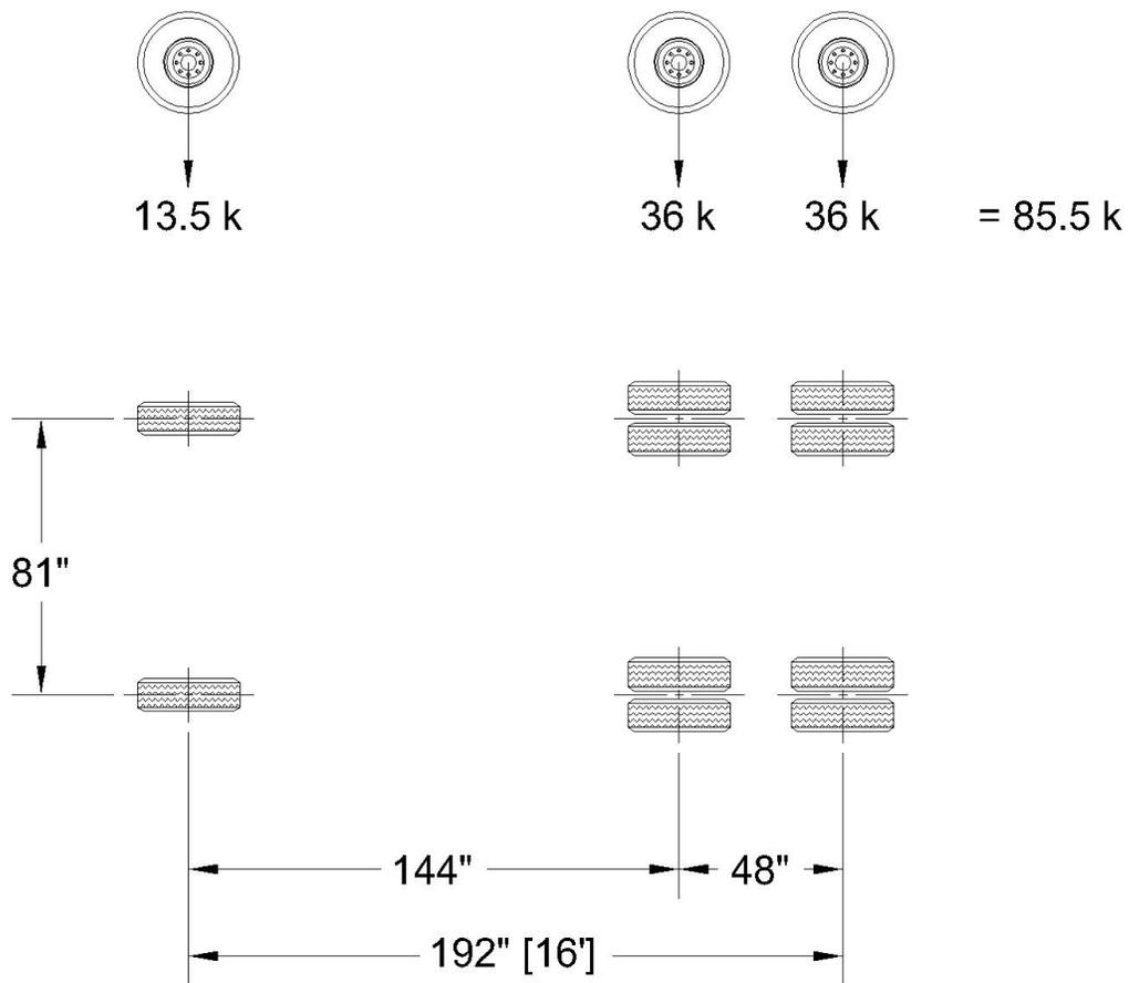
**Figure 4G-1. 3 Axle Single (3AS) Unit Loading.**
