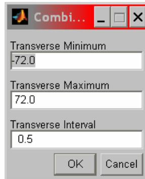
The Select button opens the Combination Settings dialog, which contains the sweep for the Transverse Profile. The data will have to be sorted and interpolated to be a fixed interval between readings.
