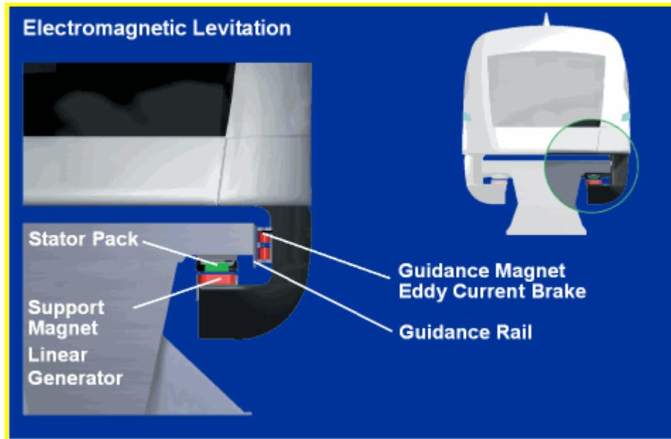
**Figure 3.6** Mechanism of Magnets (Data source: [www.transrapid.de/en/index/html](http://www.transrapid.de/en/index/html))
