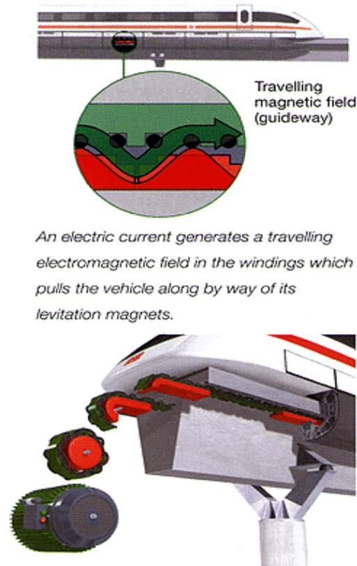
**Figure 5.4** The linear motor winding guideway used by LSM,
