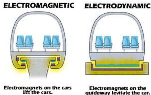
**Figure 5.3** The two basic types of levitations in Maglev,
