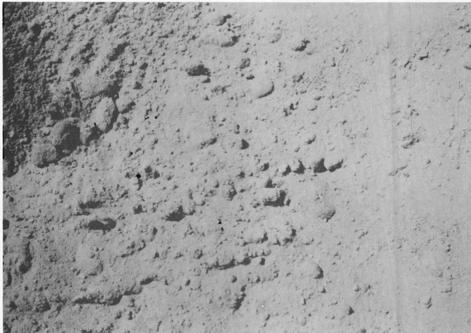
Photograph 2. Pit run bottom ash from the Monticello Power Plant, stockpiled at the HMAC plant.
