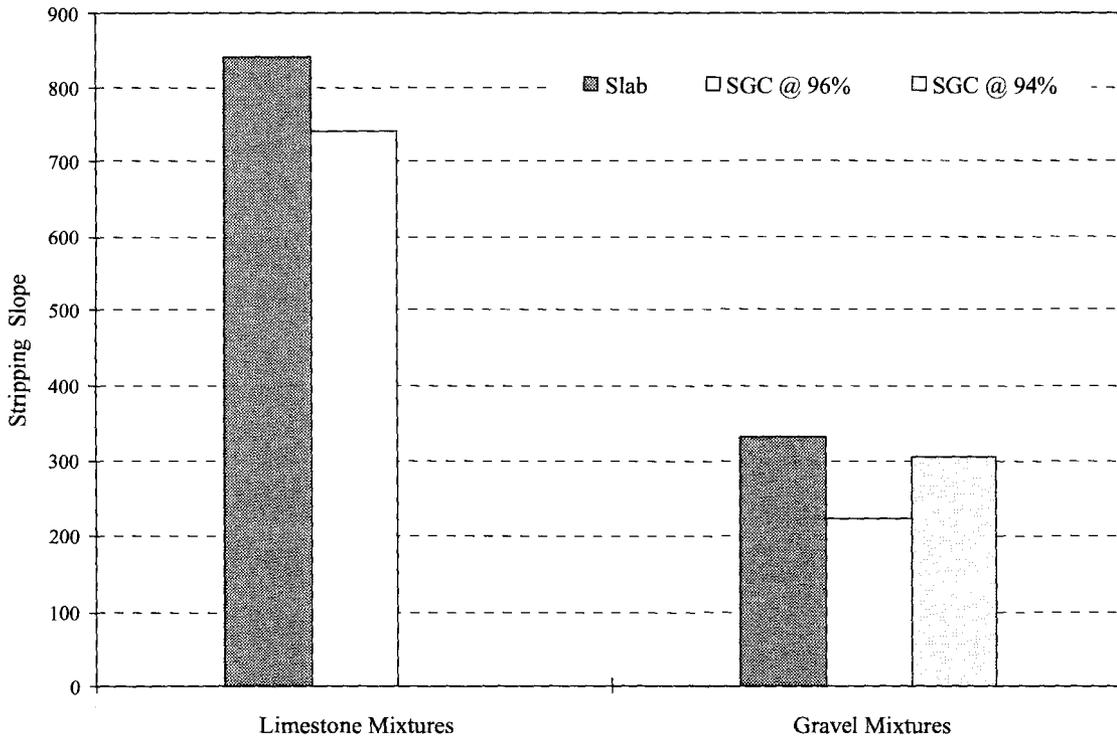
FIGURE 9: Number of passes at the stripping inflection point for slab and SGC specimens composed of limestone and gravel aggregate
