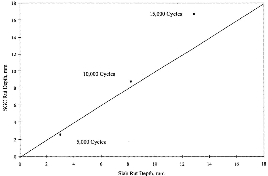
FIGURE 5: Average impression for mixtures composed of limestone @ 94% density
