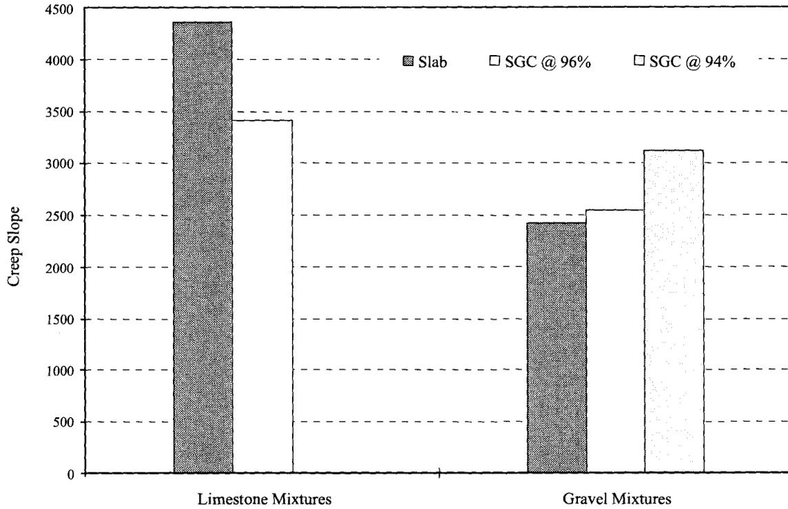
FIGURE 8: Stripping slope values for slab and SGC specimens composed of limestone and gravel aggregate
