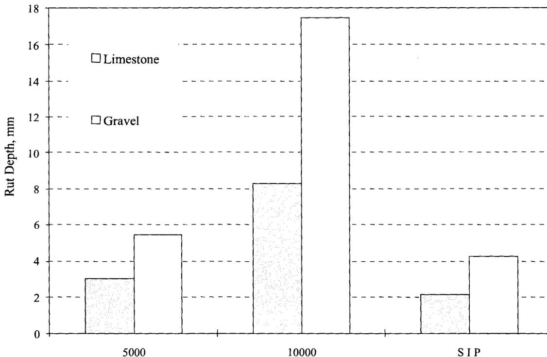
FIGURE 12: Rut depth for limestone and gravel mixtures compacted with the Superpave gyratory compactor
