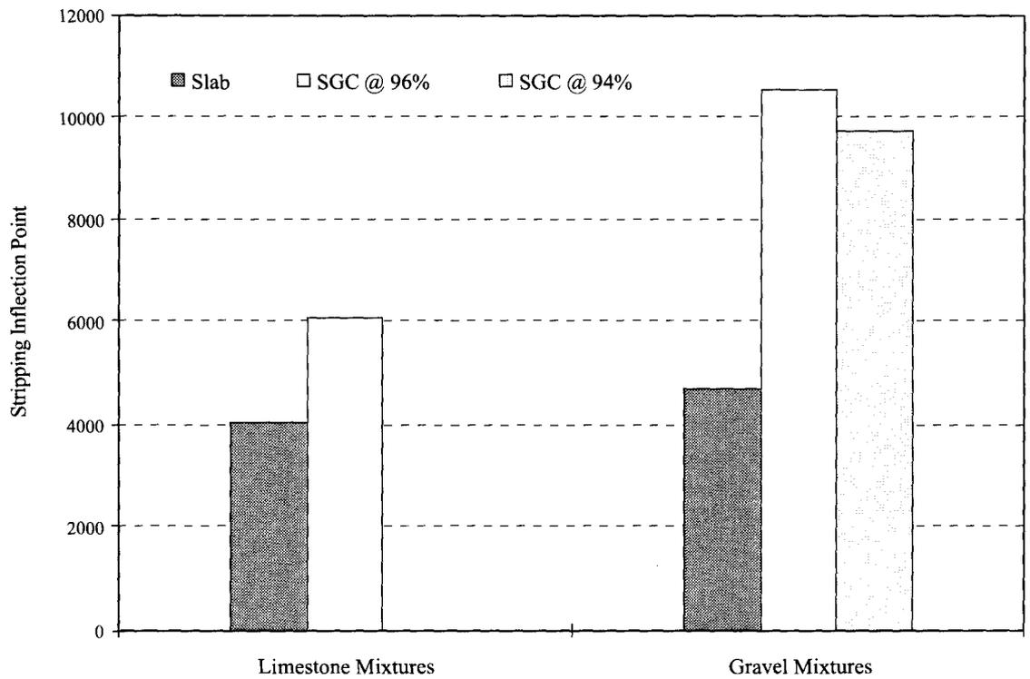
FIGURE 10: Average impression for mixtures composed of gravel at 94% and 96% density
