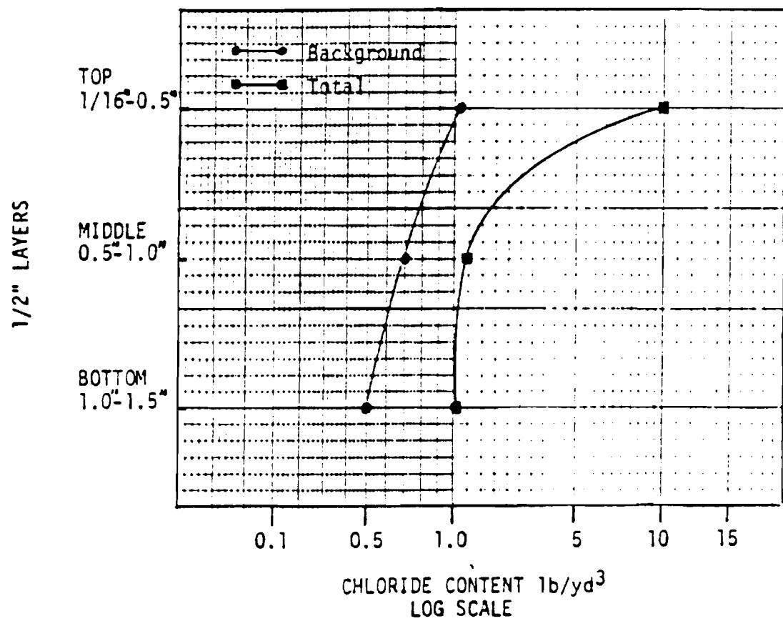
Low Water/Cement Ratio Concrete (With Super-Water Reducer)
