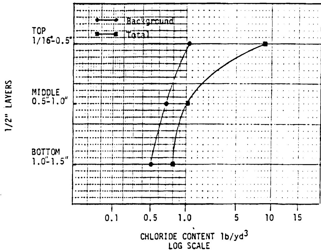
Low Water/Cement Ratio Concrete (With Super-Water Reducer)
