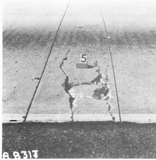
FIGURE 3 Typical saw cuts
