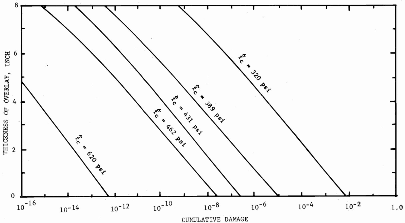
Fig 4.24. Overlay versus Damage for Normal Stiffness Pavement
