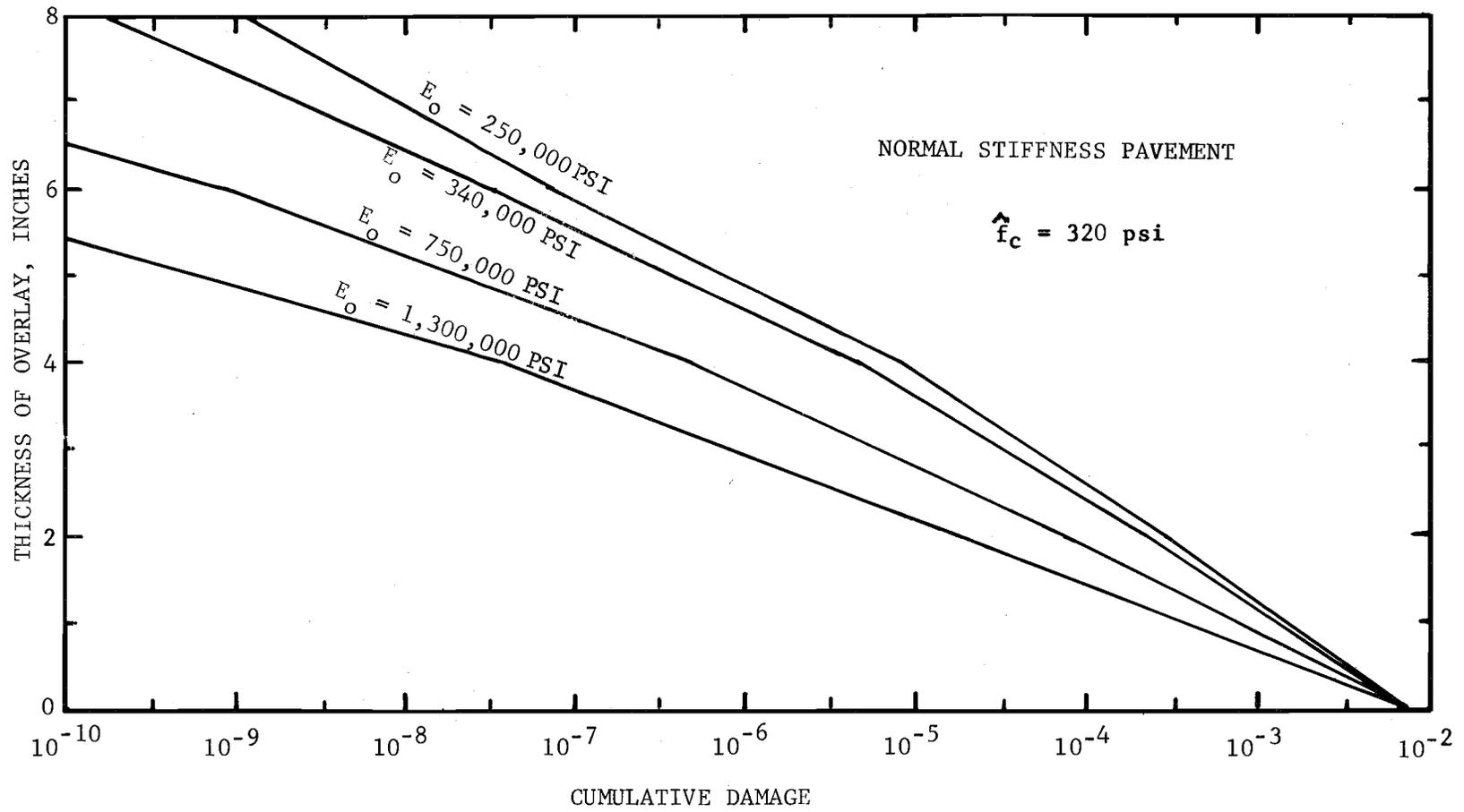
Fig 4.28. Overlay versus Damage for Normal Stiffness Pavement
