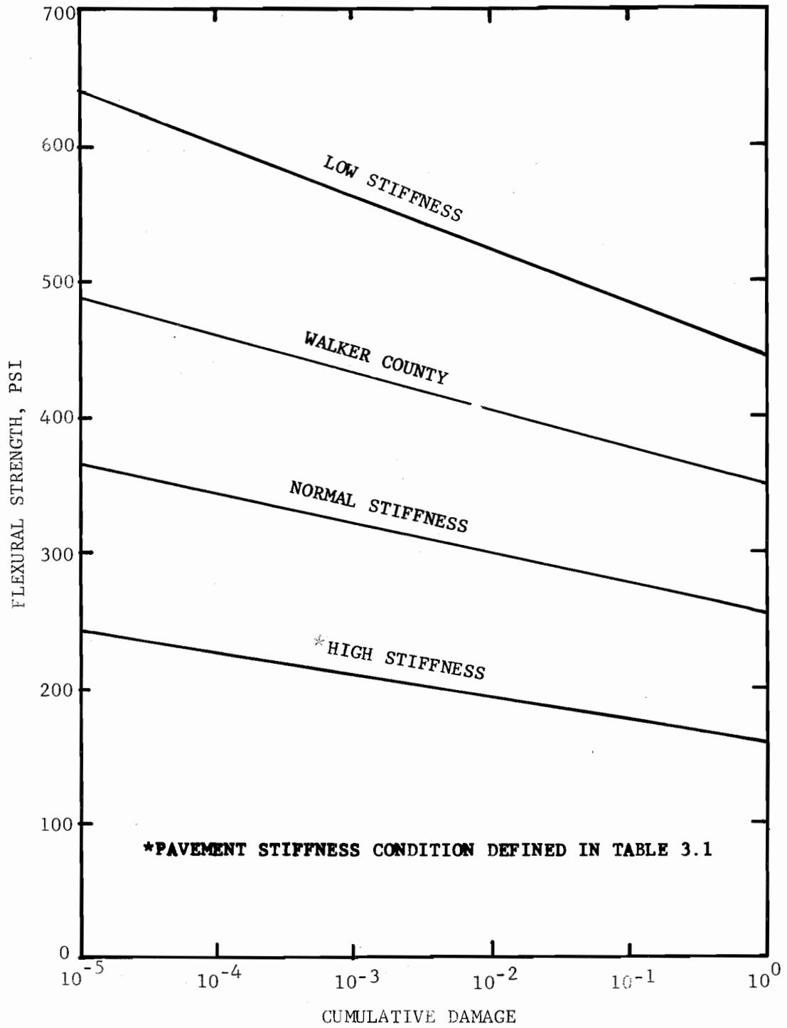
Fig 4.18. Flexural Strength versus Cumulative Damage
