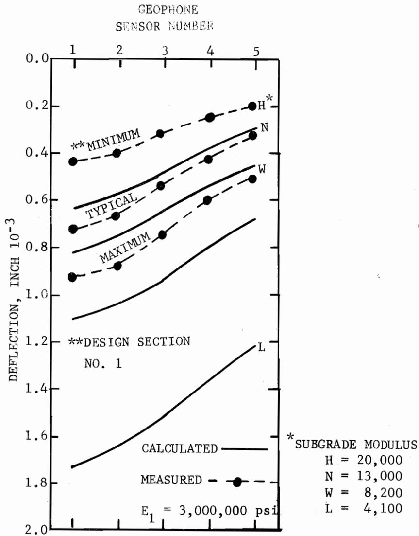
Fig B.6. Measured and Calculated Deflection Basins for Design Section No. 1
