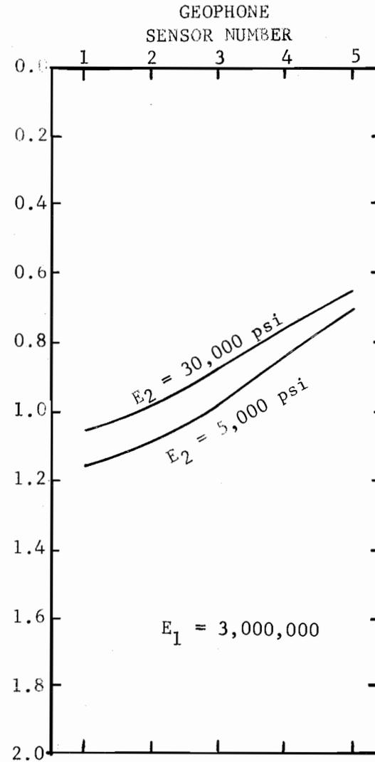
Fig. B.9. Calculated Deflection Basins Showing the Effect of Varying the Elastic Modulus of Layer 2 ( $E_1 = 3,000,000$ )
