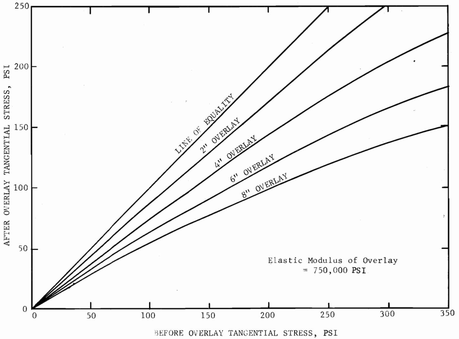
Fig 6.1. Tangential Stress Before and After Overlay
