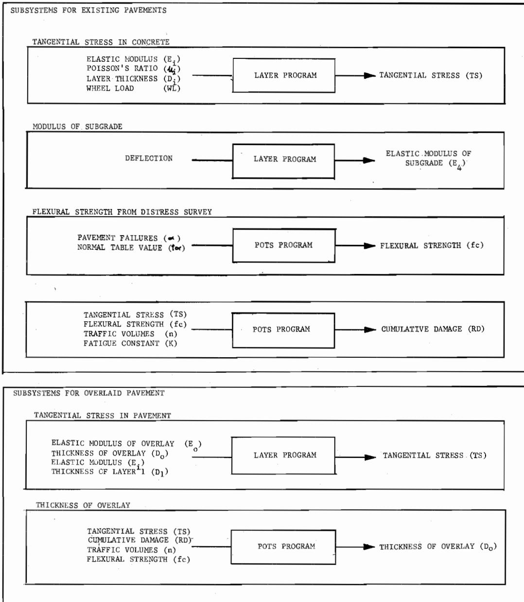
Fig 3.2. Subsystems for Analysis
