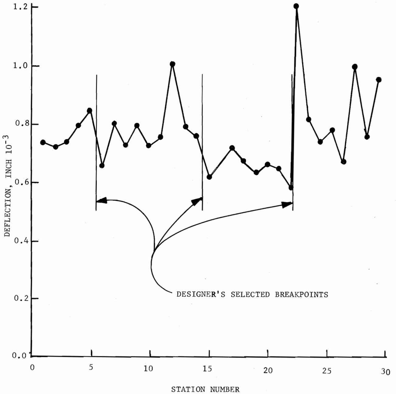
Fig 2.7. Breakpoints Chosen for Design Sections in Profile of Deflections
