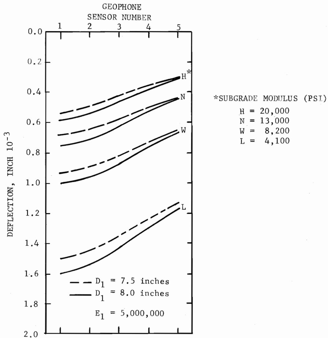
Fig B.10. Calculated Deflection Basins Showing the Effect of Varying the Thickness of Layer 1 ( $E_1 = 5,000,000$ )
