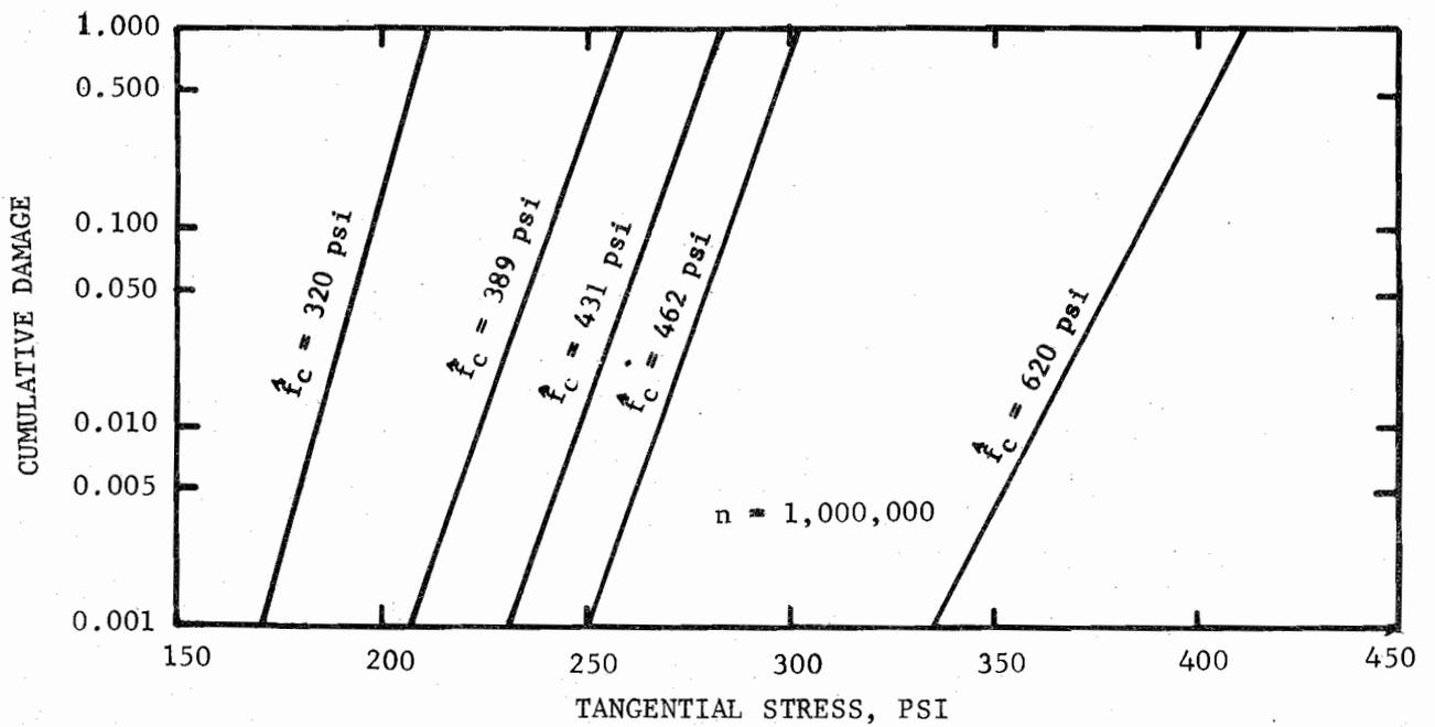
Fig 4.16. Cumulative Damage versus Tangential Stress for 1,000,000 Repetitions of Load
