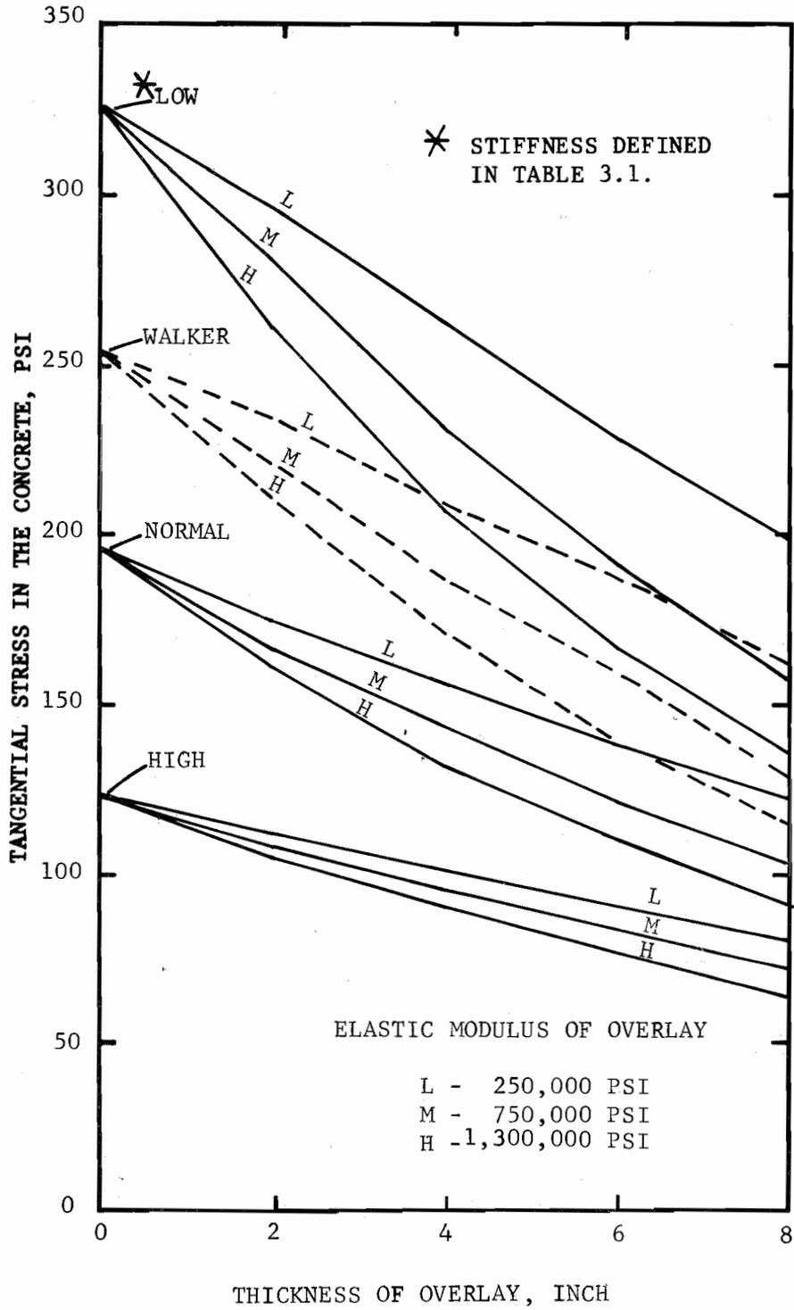
Fig 4.21. Tangential Stress versus Thickness of Overlay for Tandem Axle
