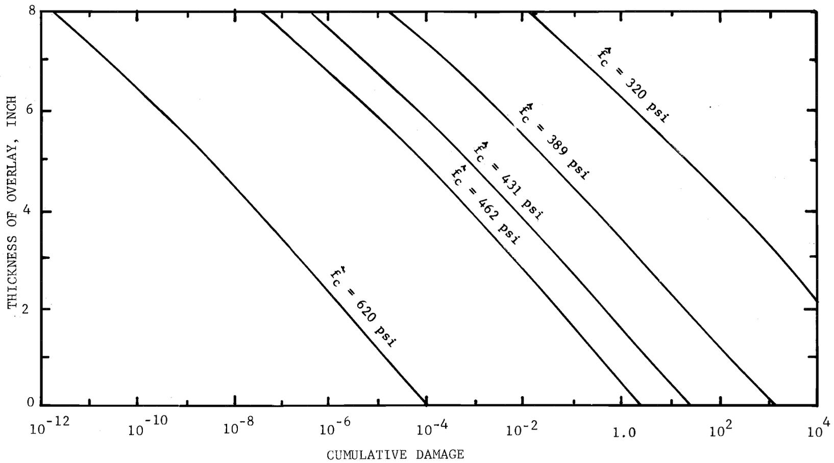
Fig 4.25. Overlay versus Damage for Low Stiffness Pavement
