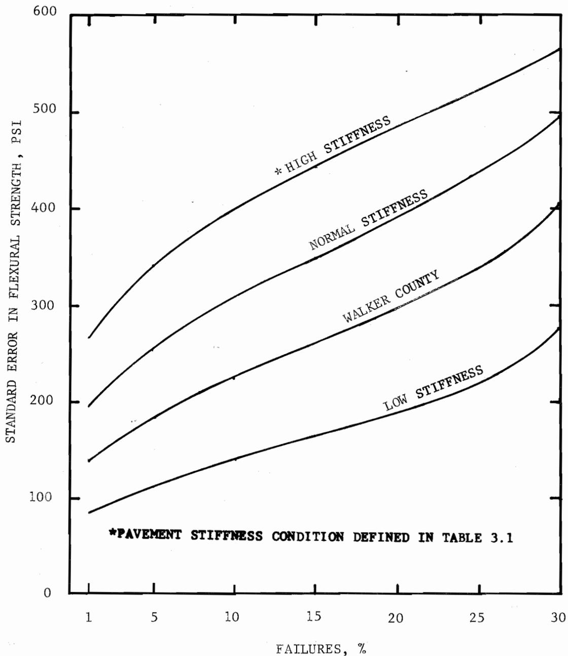
Fig 4.14. Standard Error in Flexural Strength versus Pavement Failures
