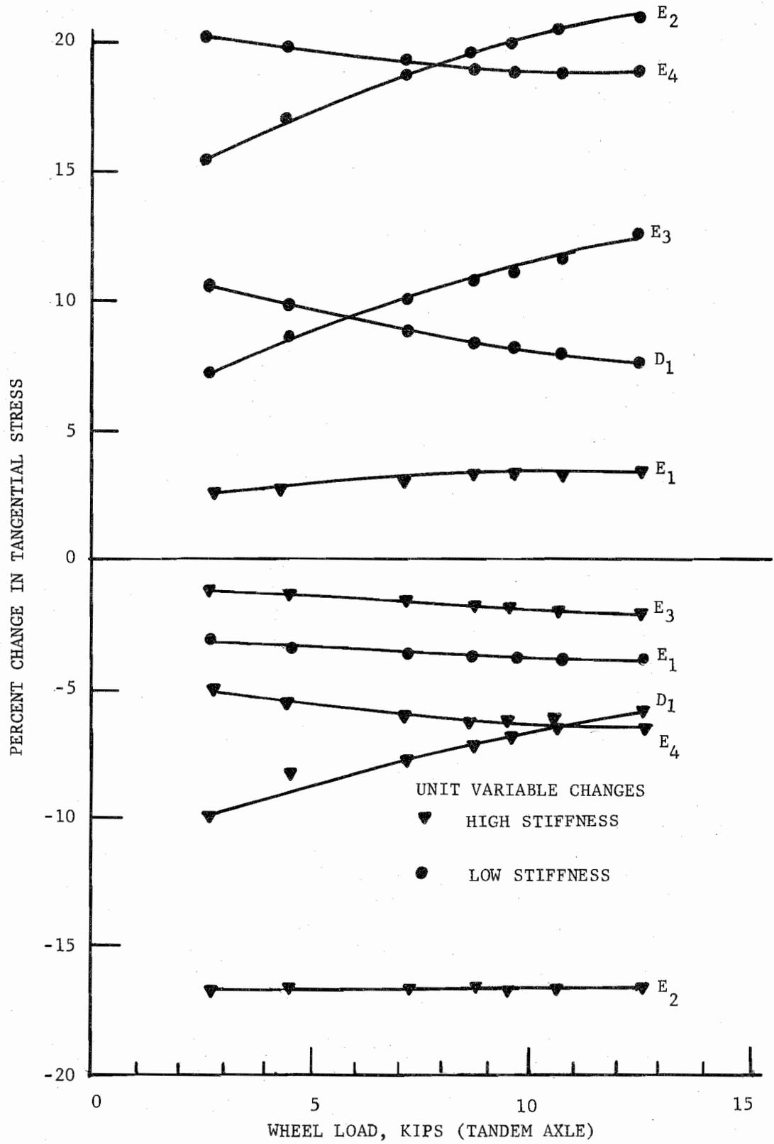
Fig 4.4 Percent Change in Tangential Stress versus Wheel Load for Unit Variable Changes
