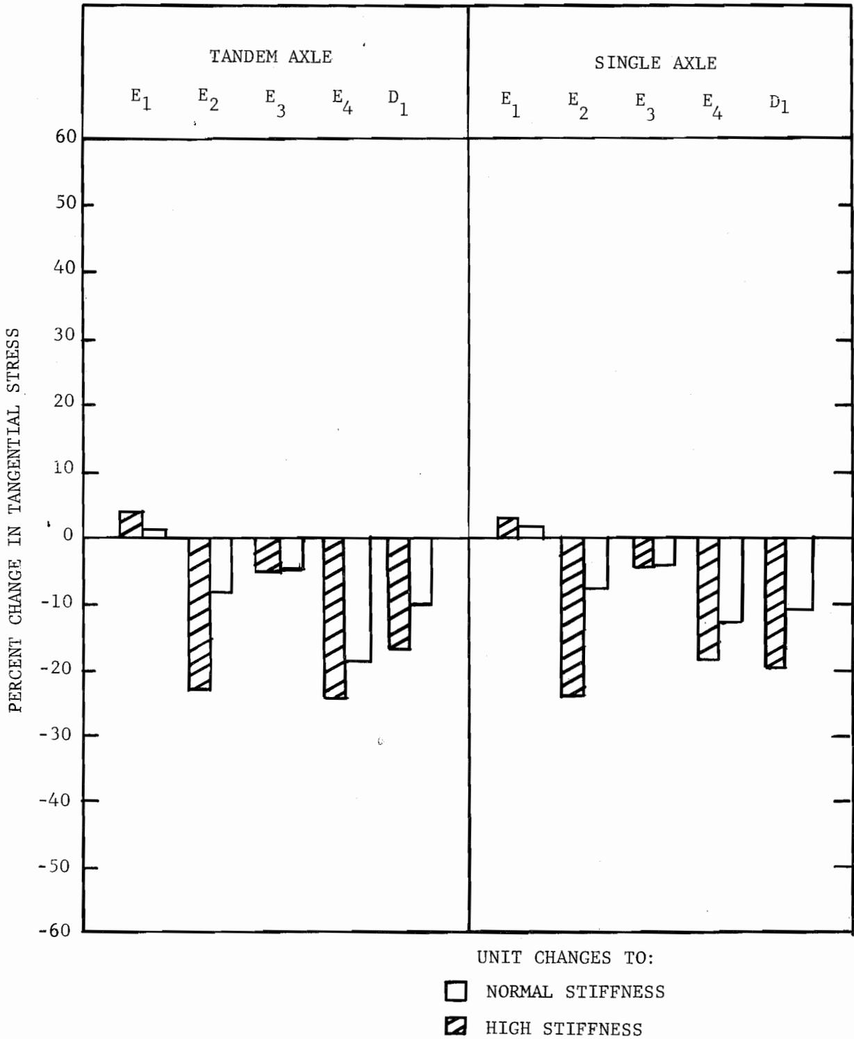
Fig 4.9. Summary of Percent Change in Tangential Stress for Low Stiffness Pavement (both Single and Tandem Axle)
