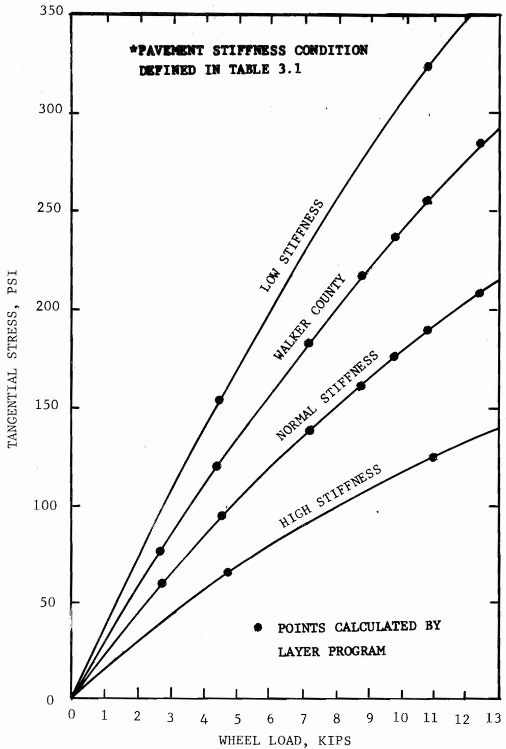
Fig 4.2. Tangential Stress versus Wheel Load for Tandem Axle
