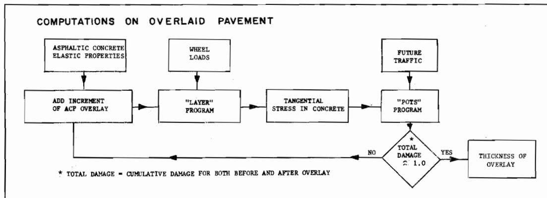
Fig 2.2. Detailed Work Flow Diagram For Each Subsystem
