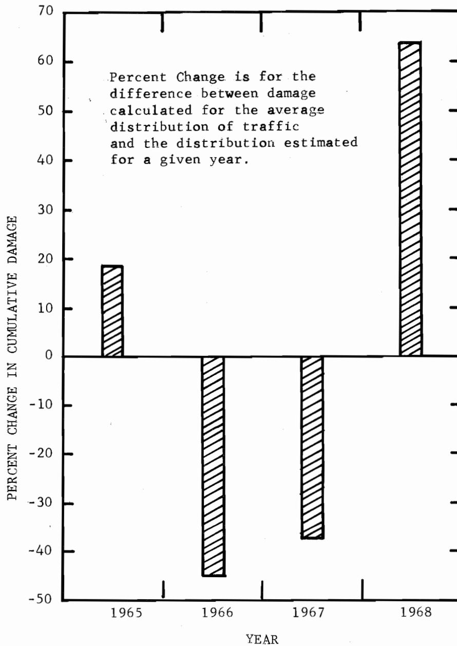
Fig 4.17. Percent Change in Cumulative Damage for the Four Estimates of Traffic Distributions given in Table 4.3.
