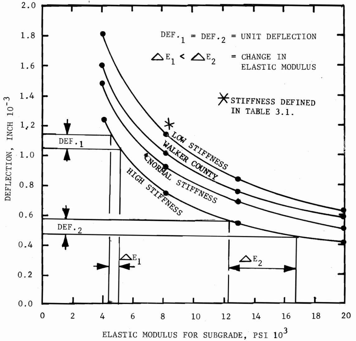
Fig 4.11. Deflection versus Subgrade Modulus ( $E_4$ )
