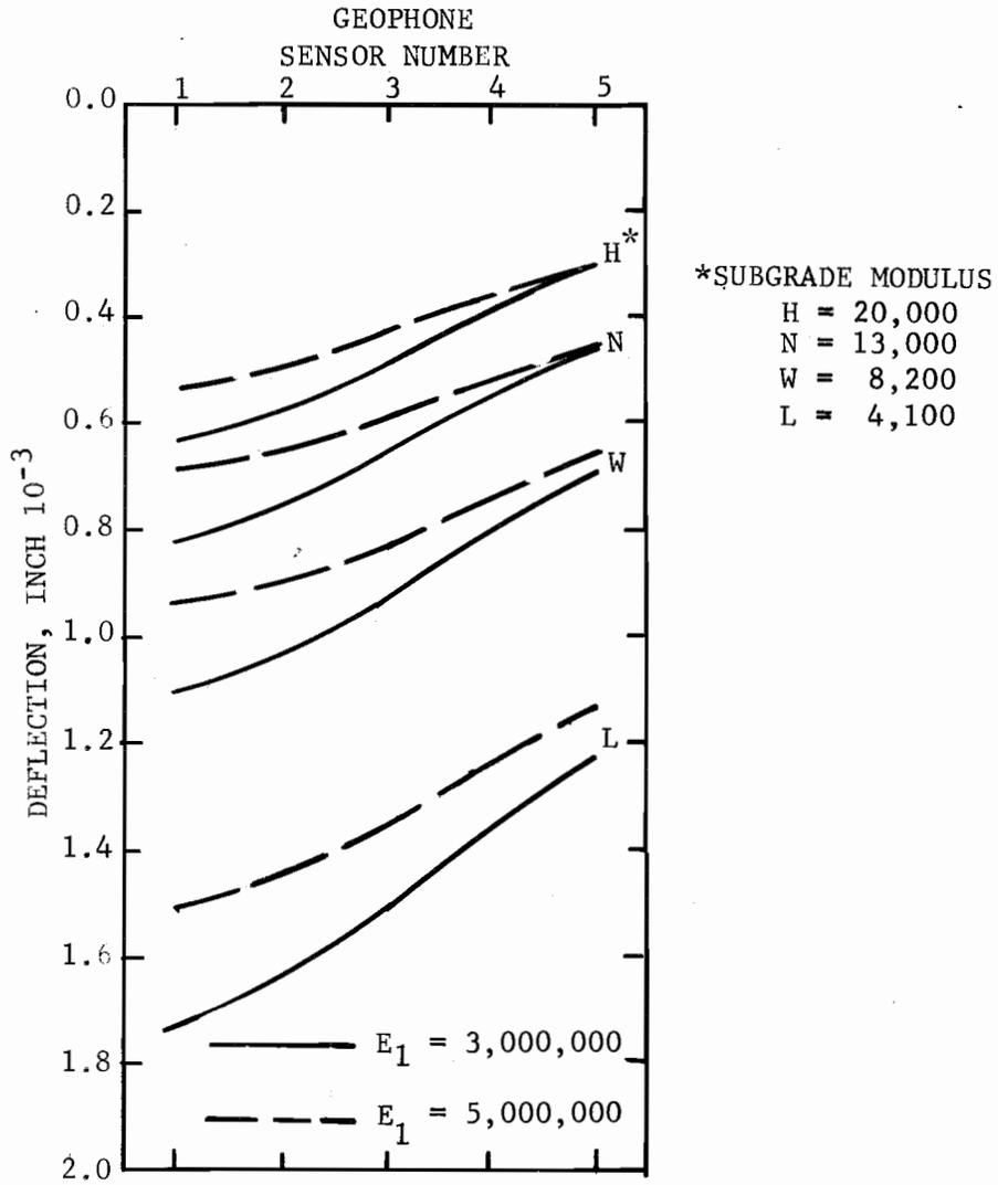
Fig B.5. Calculated Deflection Basin Showing the Effect of Varying the Elastic Modulus of Layer 1
