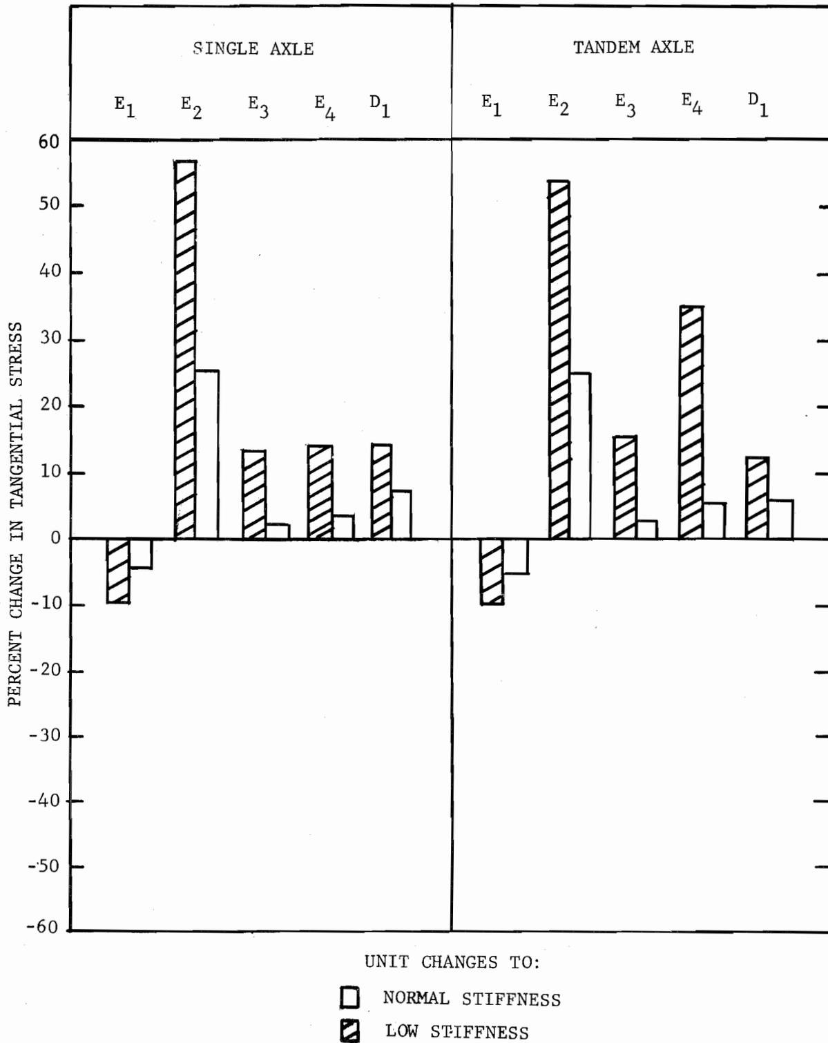
Fig 4.10. Summary of Percent Change in Tangential Stress for High Stiffness Pavement (both Single and Tandem Axle)
