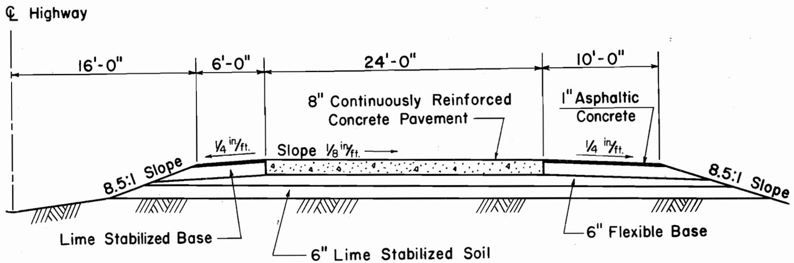
Fig B.2. Typical Half Section for Walker Project
