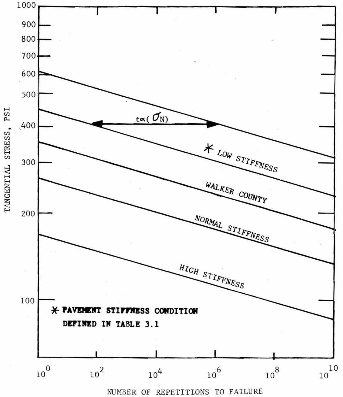
Fig 4.12. Fatigue Equation for Cumulative Damage Equal to 1.0
