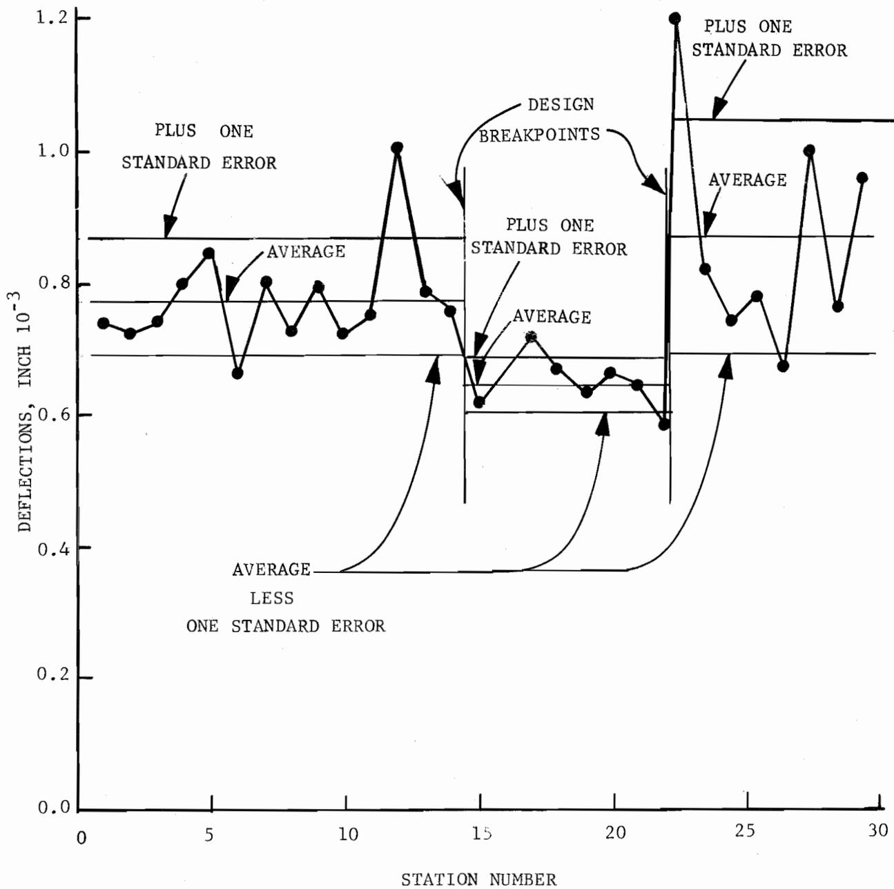
Fig 2.8. Statistically Different Design Sections in Profile of Deflections
