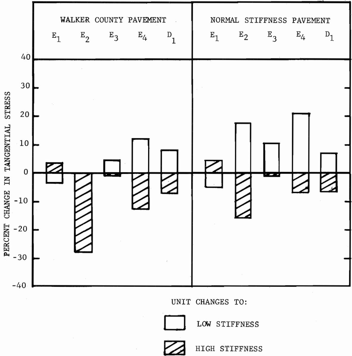
Fig 4.23. Summary of Percent Change in Tangential Stress for Overlaid Pavement (Tandem Axle)
