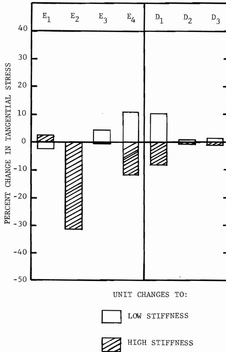
Fig 4.8. Summary of Percent Change in Tangential Stress for Walker County Pavement (Tandem Axle)
