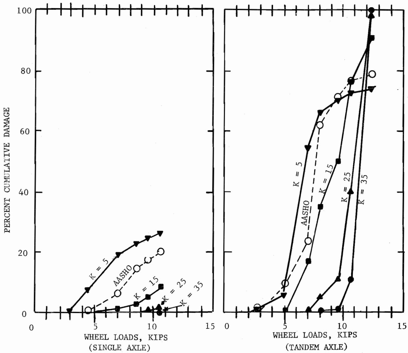
Fig 4.19. Cumulative Damage versus Wheel Load for Various Values of Slope in the Fatigue Equation
