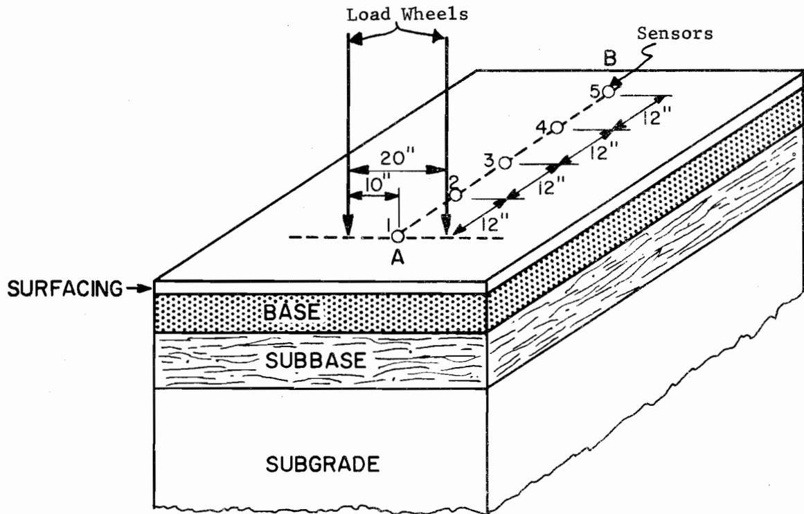
Figure B.11. Position of Dynaflect Sensors During testing
