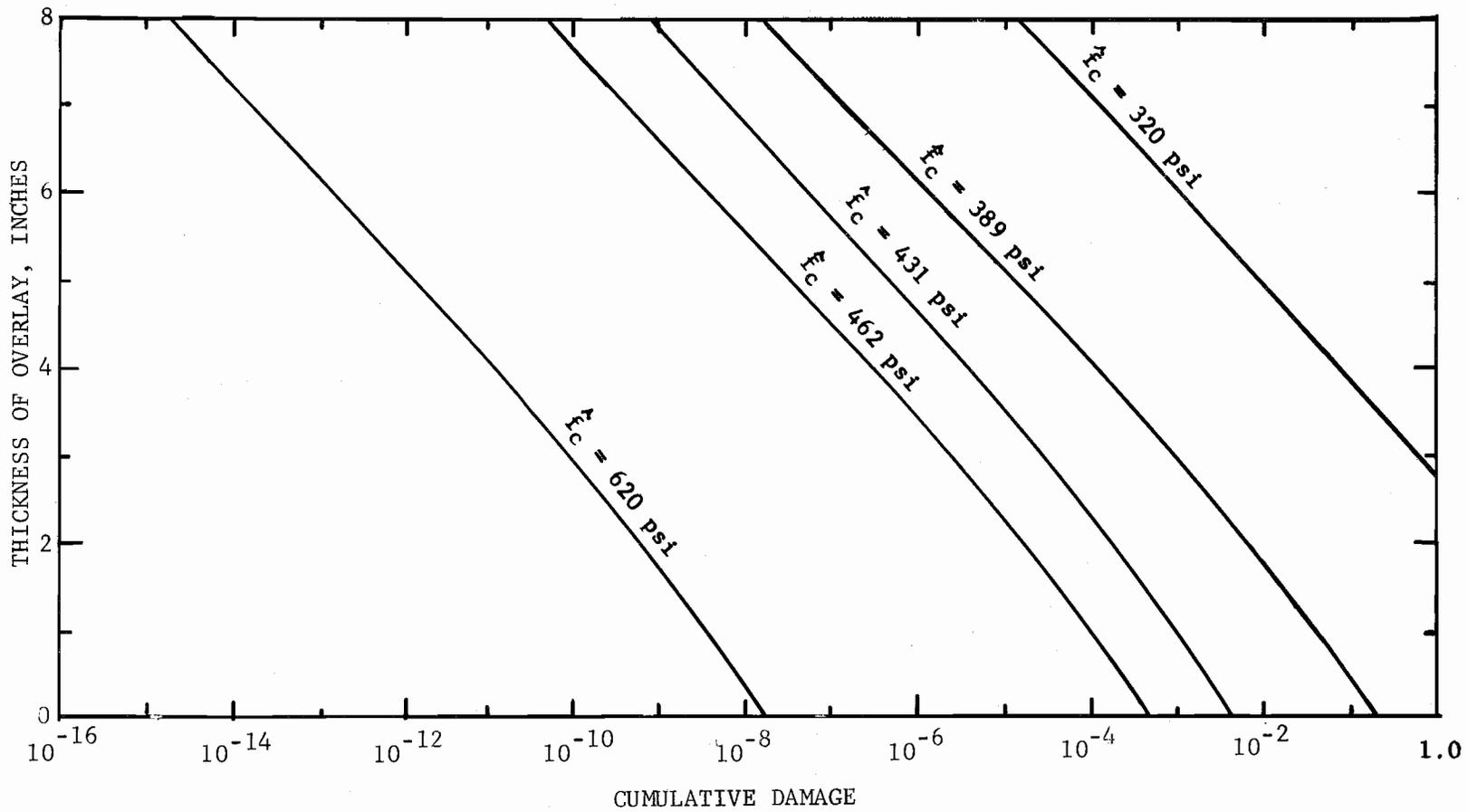
Fig 4.27. Overlay versus Damage for Walker County Pavement
