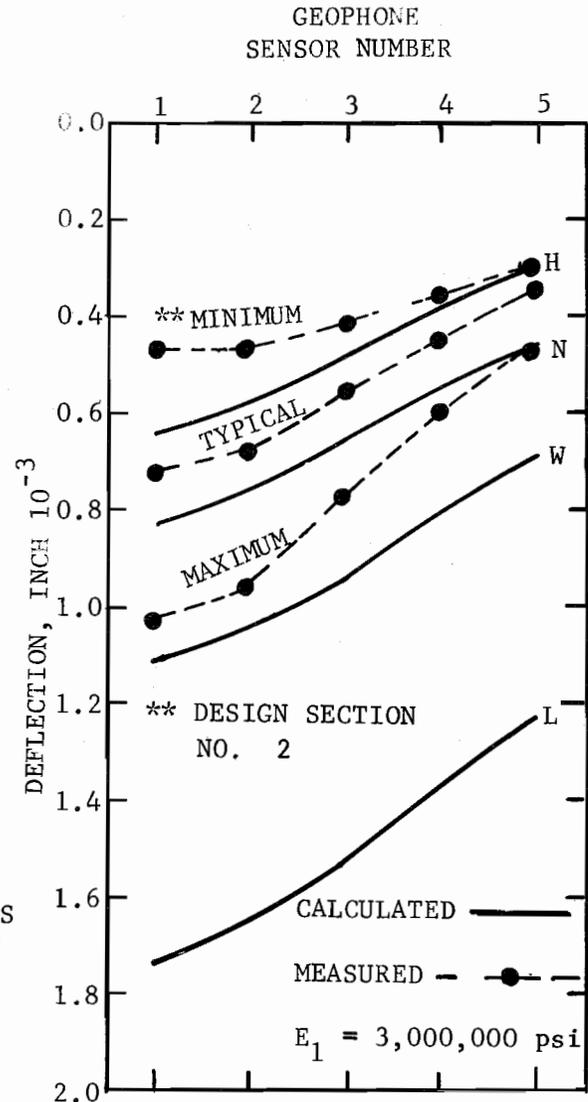
Fig B.7. Measured and Calculated Deflection Basins for Design Section No. 2
