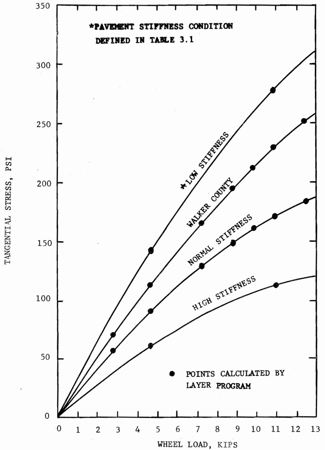
Fig 4.1. Tangential Stress versus Wheel Load for Single Axle
