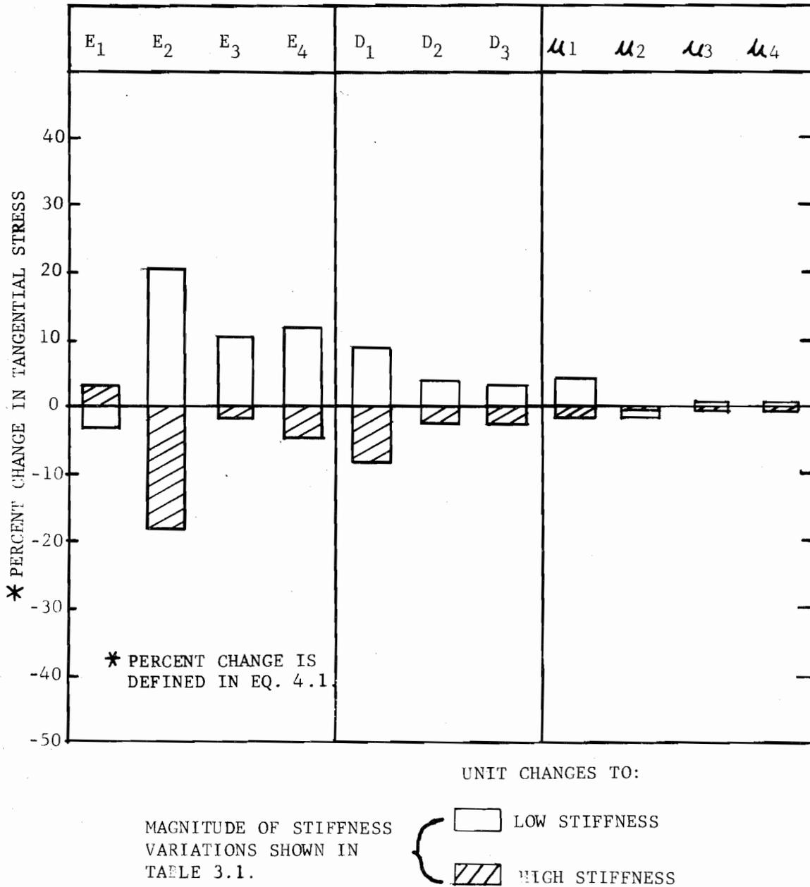
Fig 4.5. Summary of Percent Change in Tangential Stress for Normal Stiffness Pavement (Single Axle)
