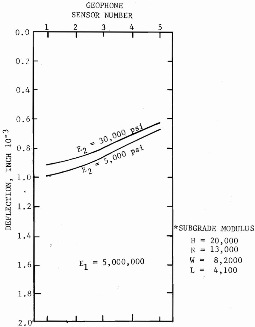
Fig. B.9. Calculated Deflection Basins Showing the Effect of Varying the Elastic Modulus of Layer 2 ( $E_1 = 5,000,000$ )
