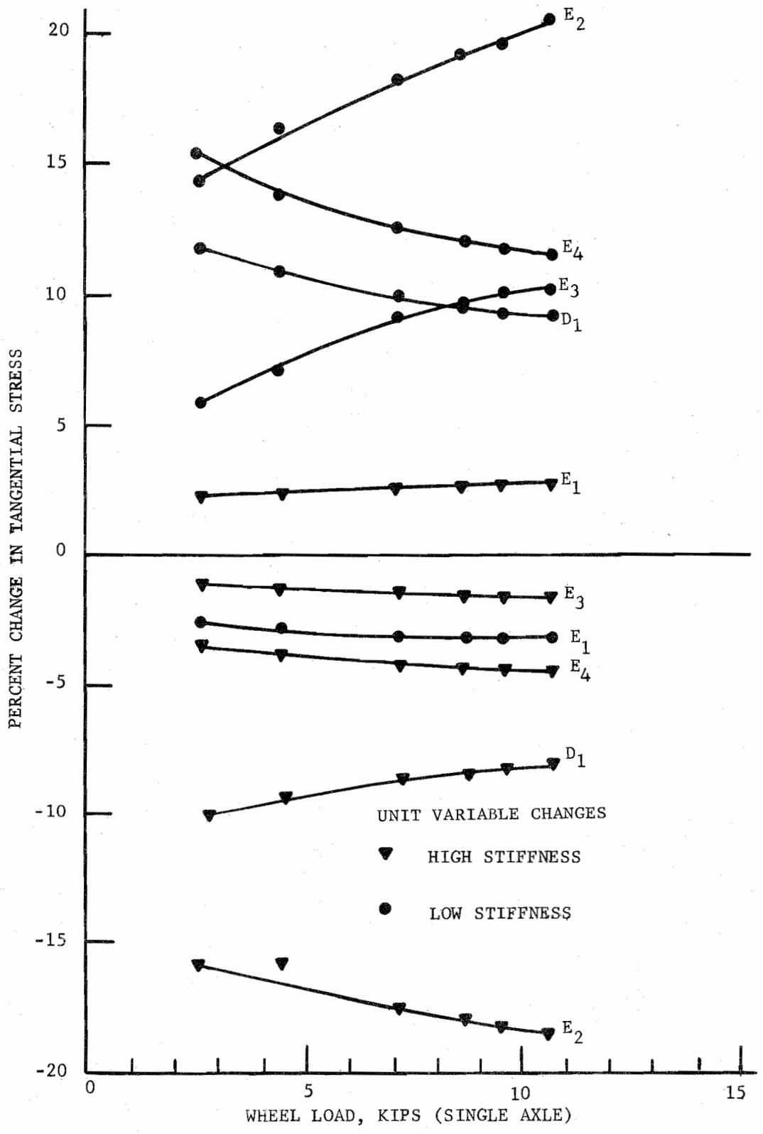
Fig 4.3. Percent Change in Tangential Stress versus Wheel Load for Unit Variable Changes
