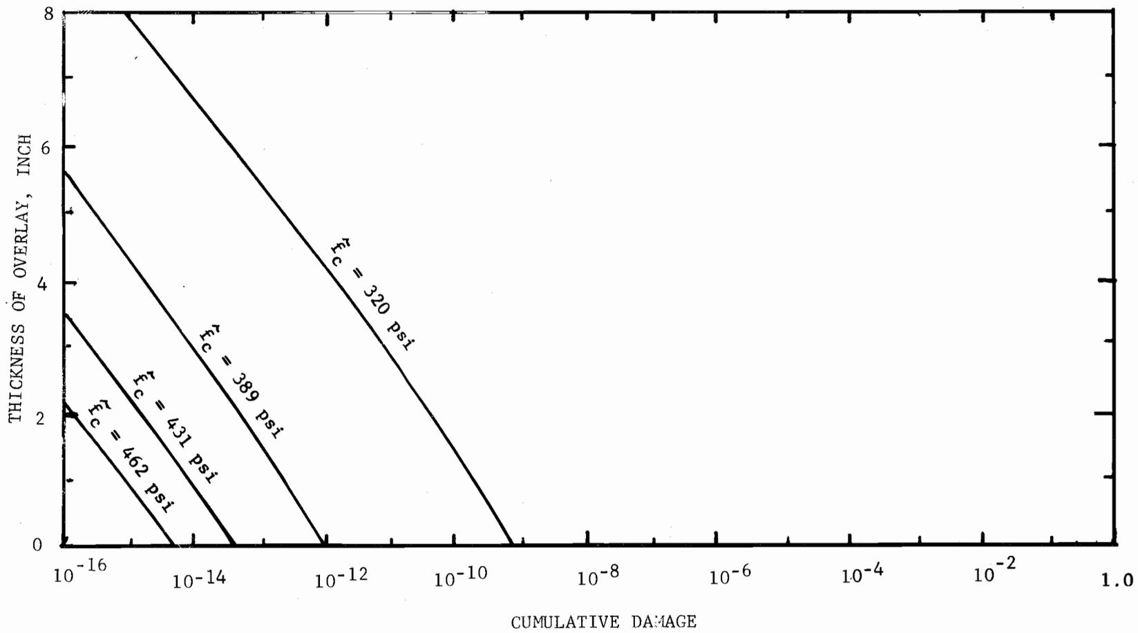
Fig 4.26. Overlay versus Damage for High Stiffness Pavement
