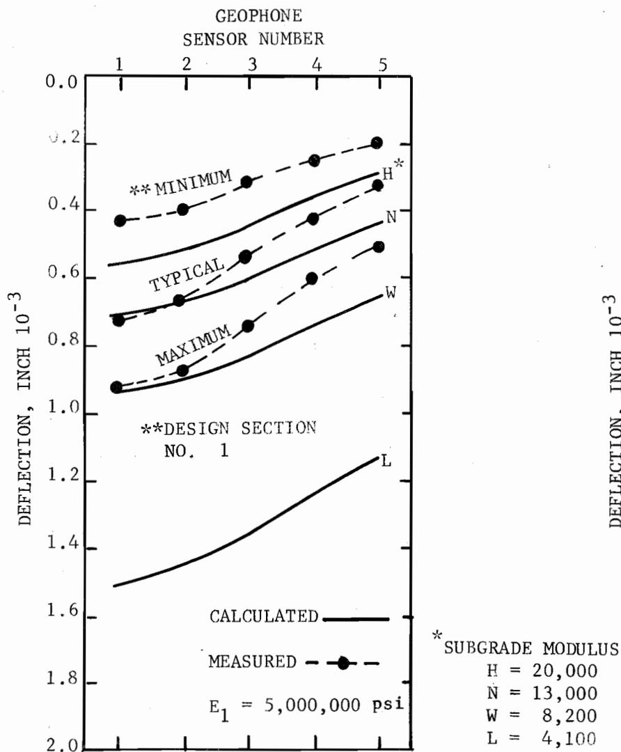
Fig B.3. Measured and Calculated Deflection Basins for Design Section No. 1 ( $E_1 = 5,000,000$  psi)
