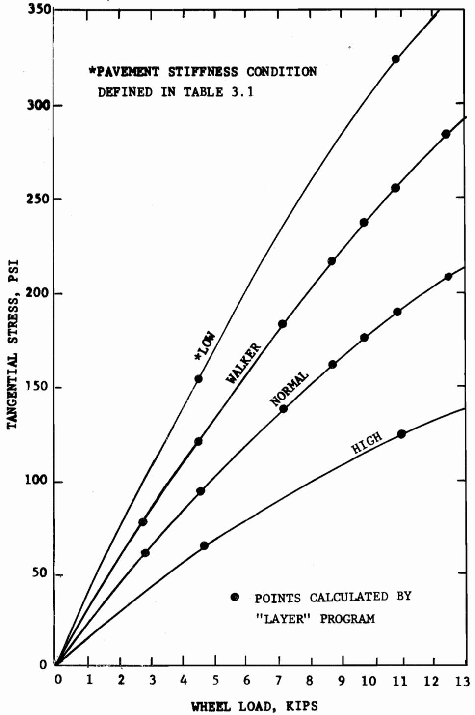
Fig A.1. Tangential Stress versus Wheel Load For Tandem Axle
