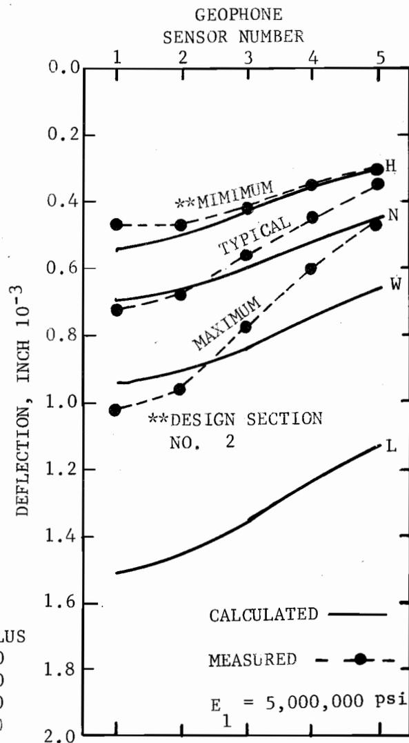
Fig B.4. Measured and Calculated Deflection Basins for Design Section No. 2 ( $E_1 = 5,000,000$  psi)
