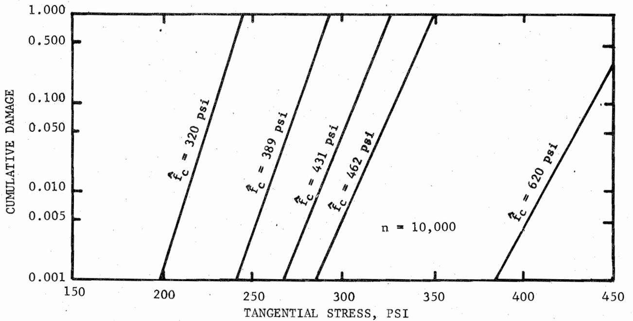
Fig 4.15. Cumulative Damage versus Tangential Stress for 10,000 Repetitions of Load
