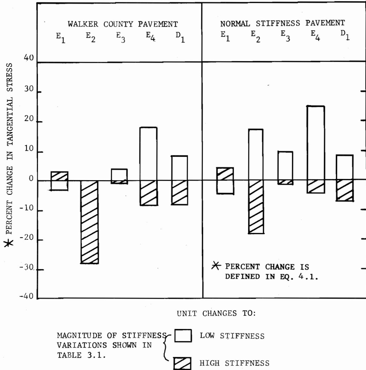
Fig 4.22. Summary of Percent Change in Tangential Stress for Overlaid Pavement (Single Axle)
