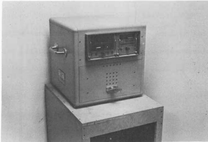
Figure 1. Nuclear Asphalt Gauge
