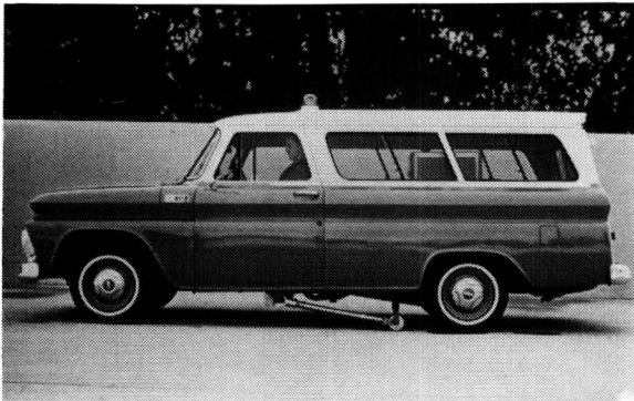
Slide 26.25. Surface Dynamics Profilometer - mounted under the vehicle.
