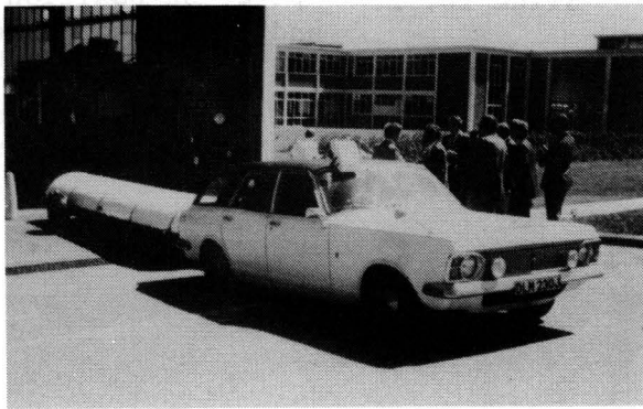
Slide 26.29. The TRRL high-speed profilometer uses four laser beams.
