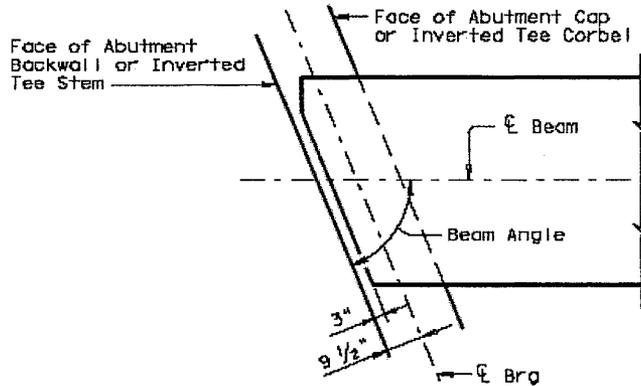
*Figure B.1.2 Beam End Detail for Texas U54 Beams (TxDOT 2001)*
