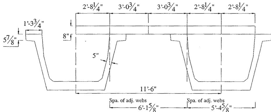
*Figure B.2.5 Effective Flange Width Calculations*
