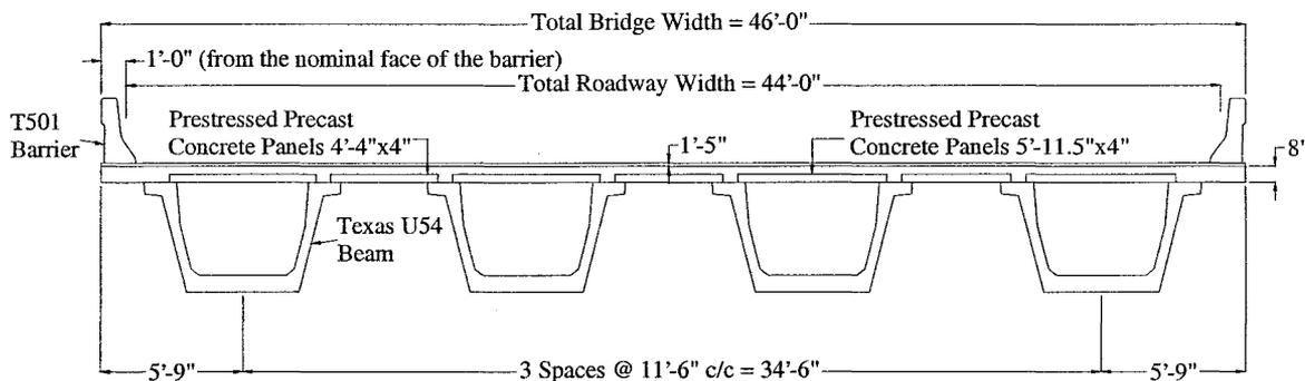
Figure B.1.1 Bridge Cross-Section Details
