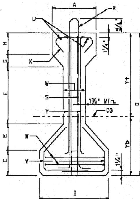
*Figure A.2.4.1 Section Geometry of AASHTO Type IV Girder (TxDOT 2001)*
