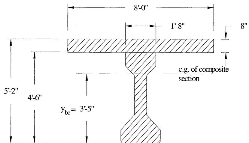
Figure A.1.4.3. Composite Section
