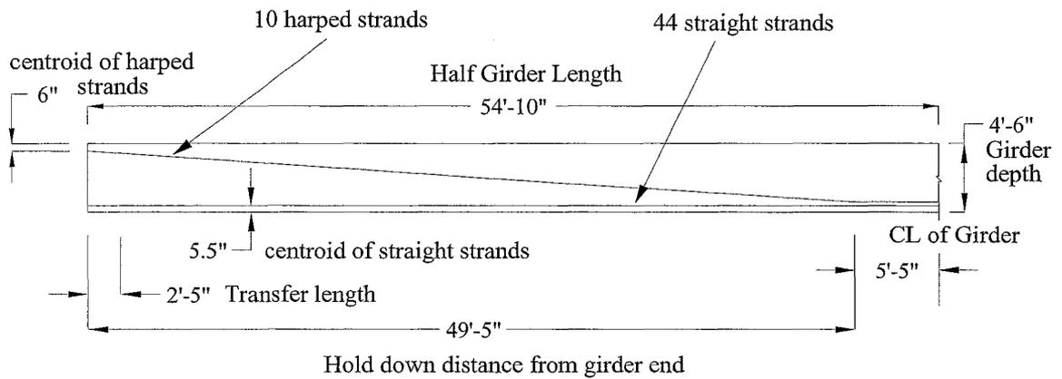
Fig. A.2.7.3 Longitudinal Strand Profile (half of the girder length is shown)
