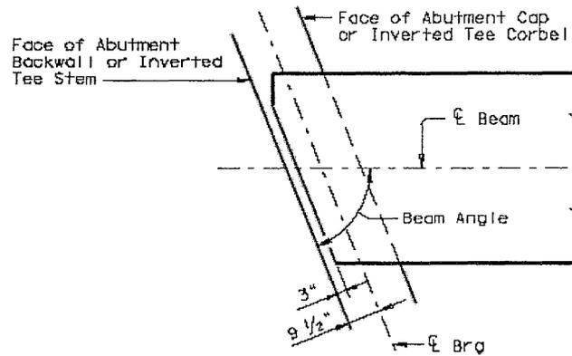
*Figure B.2.2 Beam End Detail for Texas U54 Beams (TxDOT 2001)*
