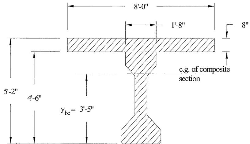
Figure A.2.4.3 Composite Section
