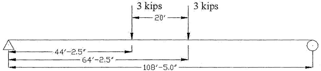
*Figure B.1.7 Location of interior diaphragms on a simply supported bridge girder.*
