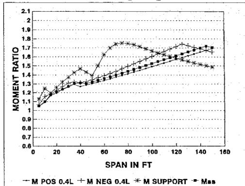
Figure C3.6.1.2.1-5 - Moment Ratios - Notional Model to HS20 (truck or lane) or two 24.0-KIP Axles at 4.0 FT
