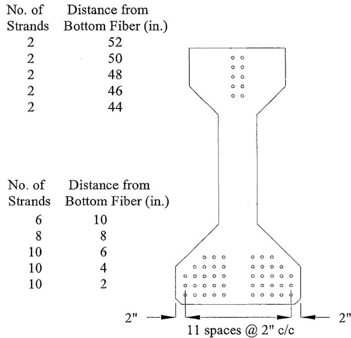
Fig. A.2.7.2 Final Strand Pattern at Girder End
