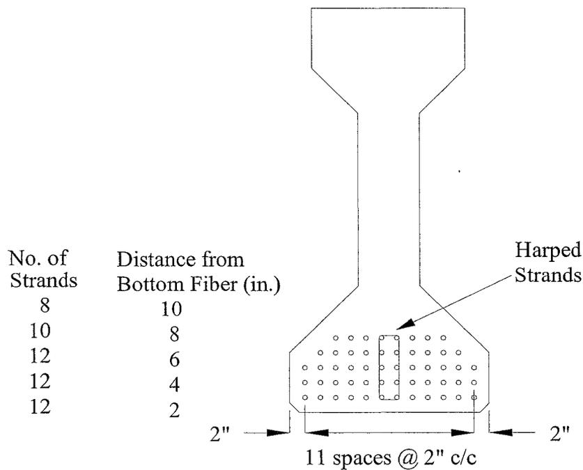
*Fig.A.2.7.1 Final Strand Pattern at Midspan Section*
