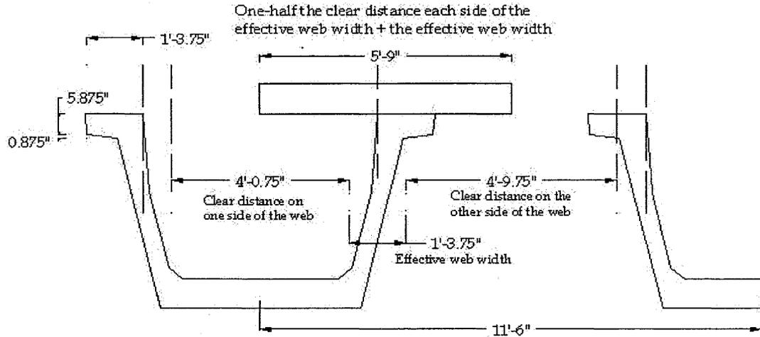
Figure B.1.5 Effective Flange Width Calculation
