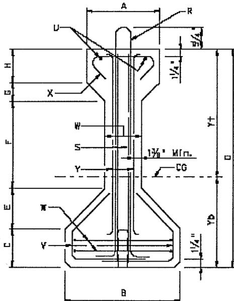
Figure A.1.4.1. Section Geometry of AASHTO Type IV Girder (TxDOT 2001)
