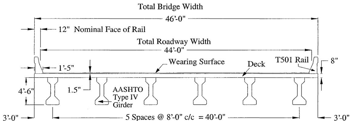
Figure A.1.2.1. Bridge Cross-Section Details
