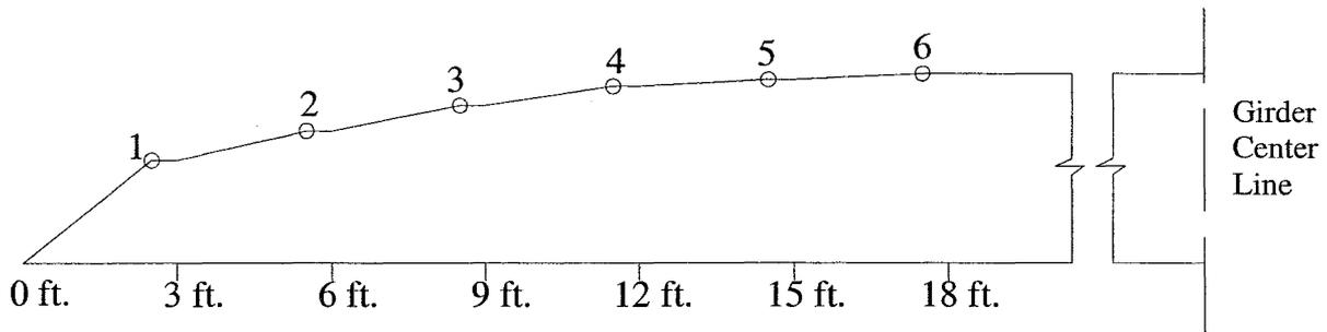
Figure B.1.9  $M/EI$  Diagram to Calculate the Initial Camber due to Prestress
