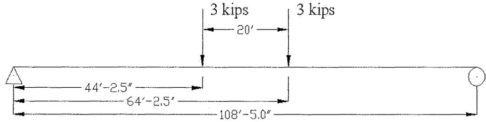
Figure B.2.7 Location of interior diaphragms on a simply supported bridge girder.
