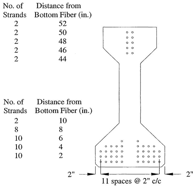
Figure A.1.7.2. Final Strand Pattern at Girder End
