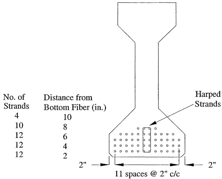
Figure A.1.7.1. Final Strand Pattern at Midspan
