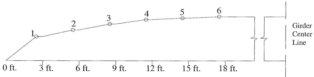
Figure B.2.9  $M/EI$  Diagram to Calculate the Initial Camber due to Prestress
