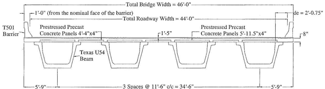
Figure B.2.1 Bridge Cross-Section Details
