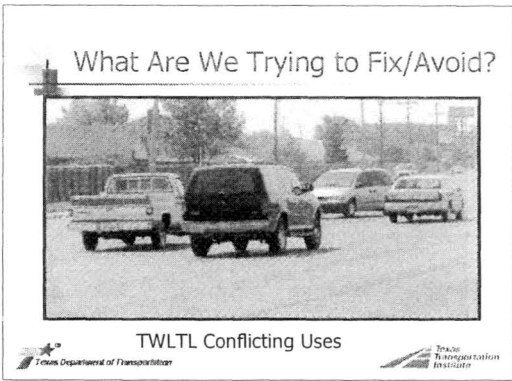
This photograph shows the conflicting uses (head-on turning traffic) that can occur in a TWLTL.
