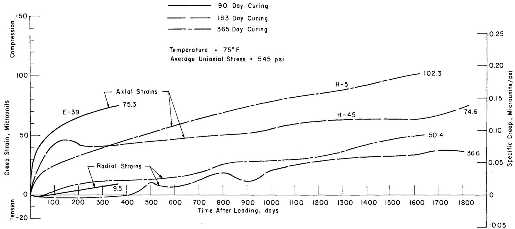
Fig 15. Axial and radial creep strain relationships for as-cast specimens with uniaxial stress of 600 psi.
