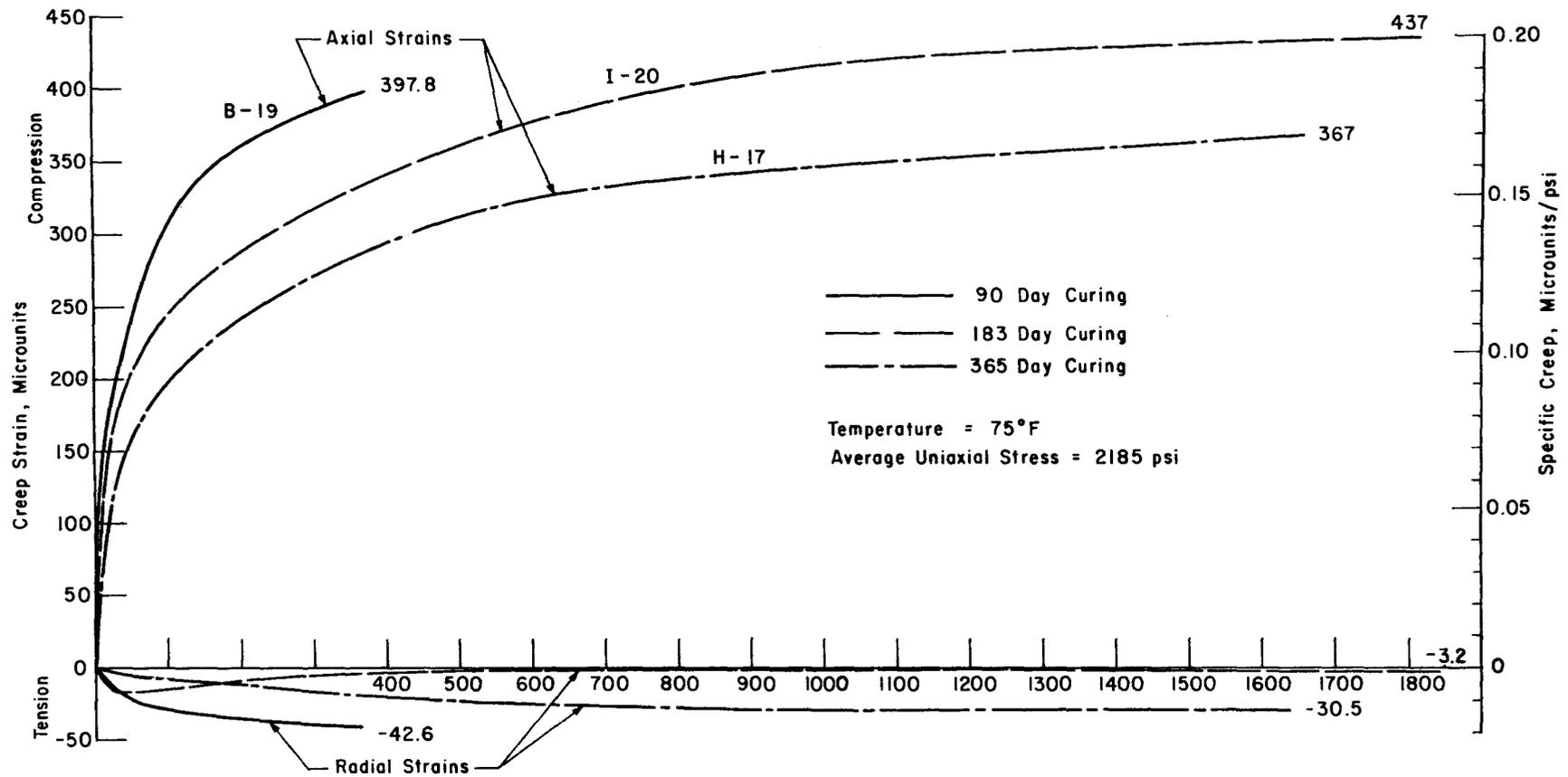
Fig 14. Axial and radial creep strain relationships for air-dried specimens with uniaxial stress of 2400 psi.
