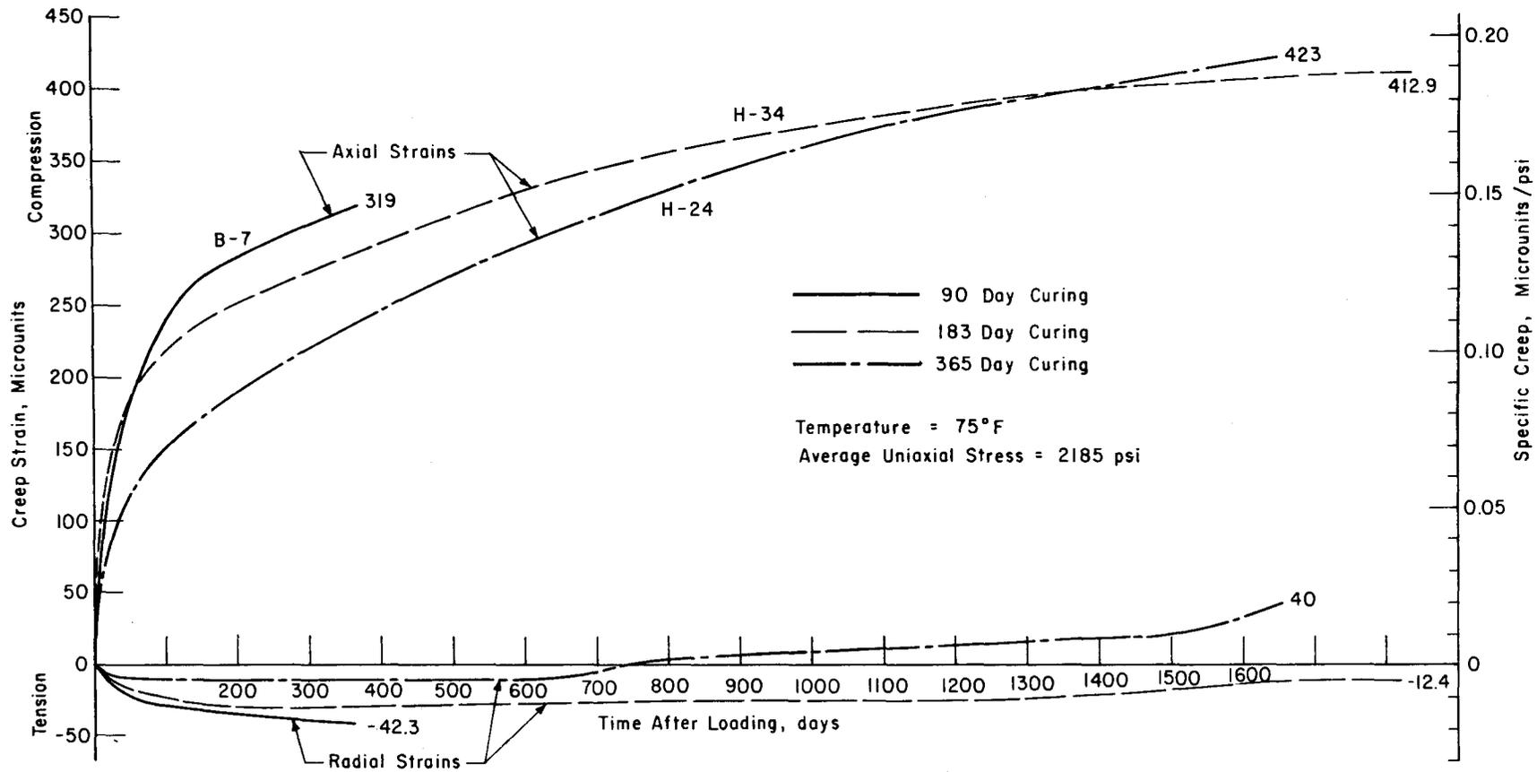
Fig 13. Axial and radial creep strain relationships for as-cast specimens with uniaxial stress of 2400 psi.
