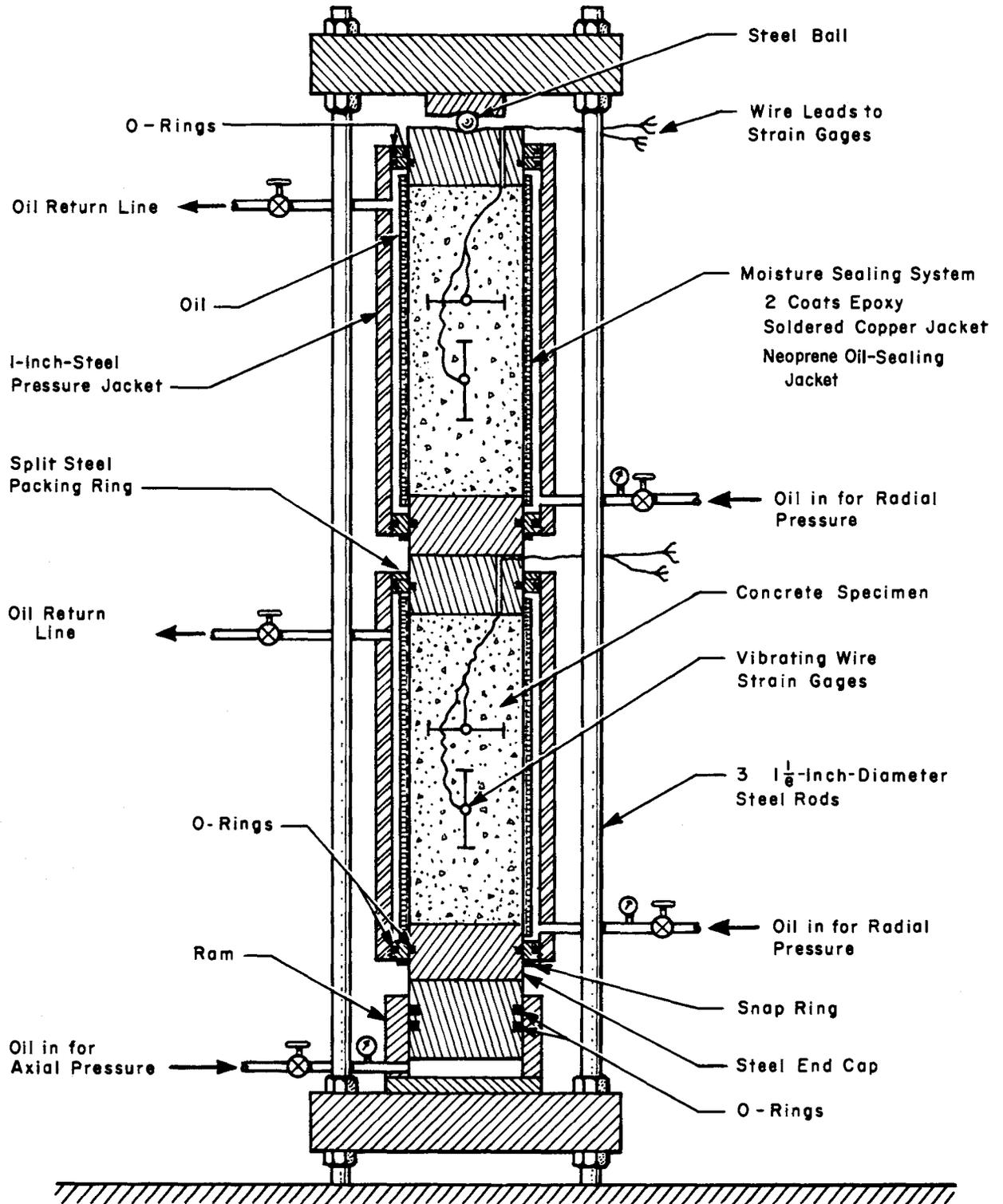
Fig 1. Schematic of triaxial test unit.
