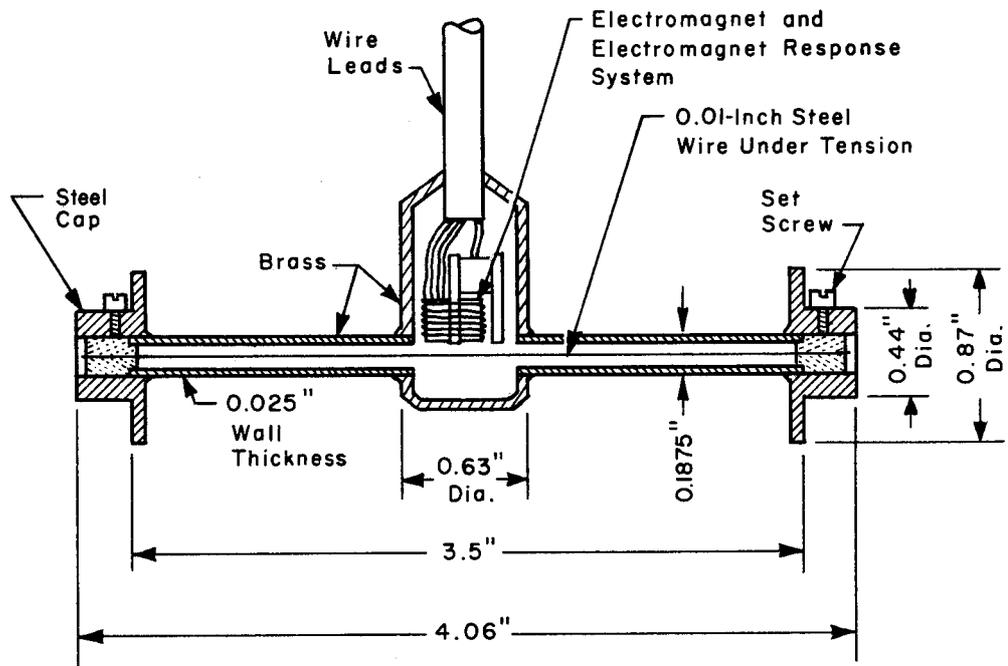
Fig 4. Cross section of Perivale vibrating wire strain gage.
