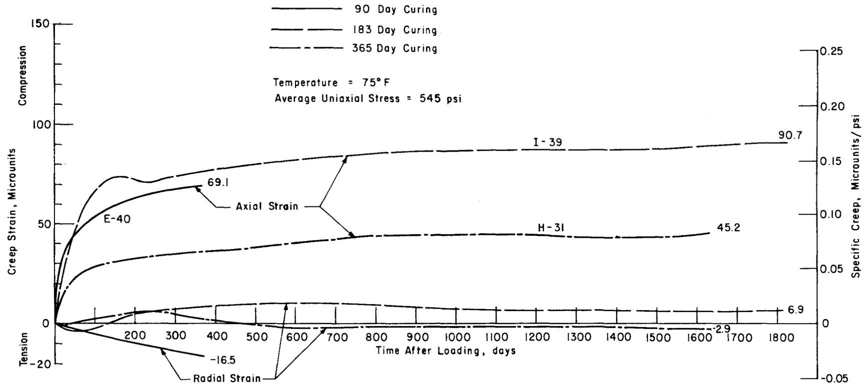
Fig 16. Axial and radial creep strain relationships for air-dried specimens with uniaxial stress of 600 psi.
