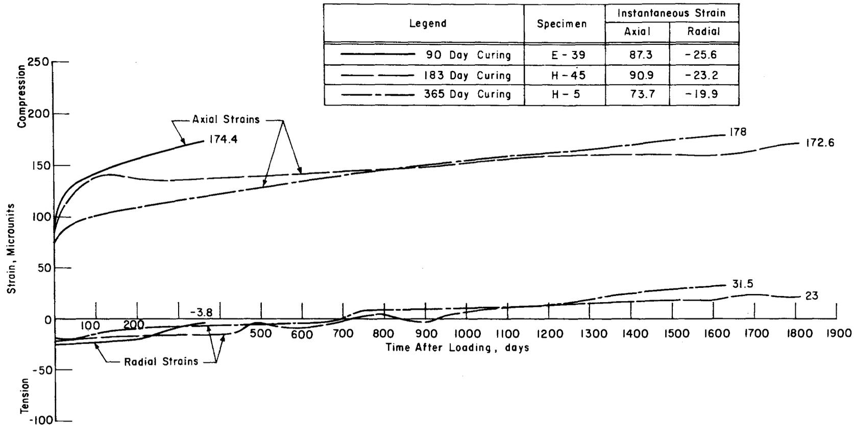
Fig 9. Total axial and radial strain relationships for as-cast specimens with uniaxial stress of 600 psi.
