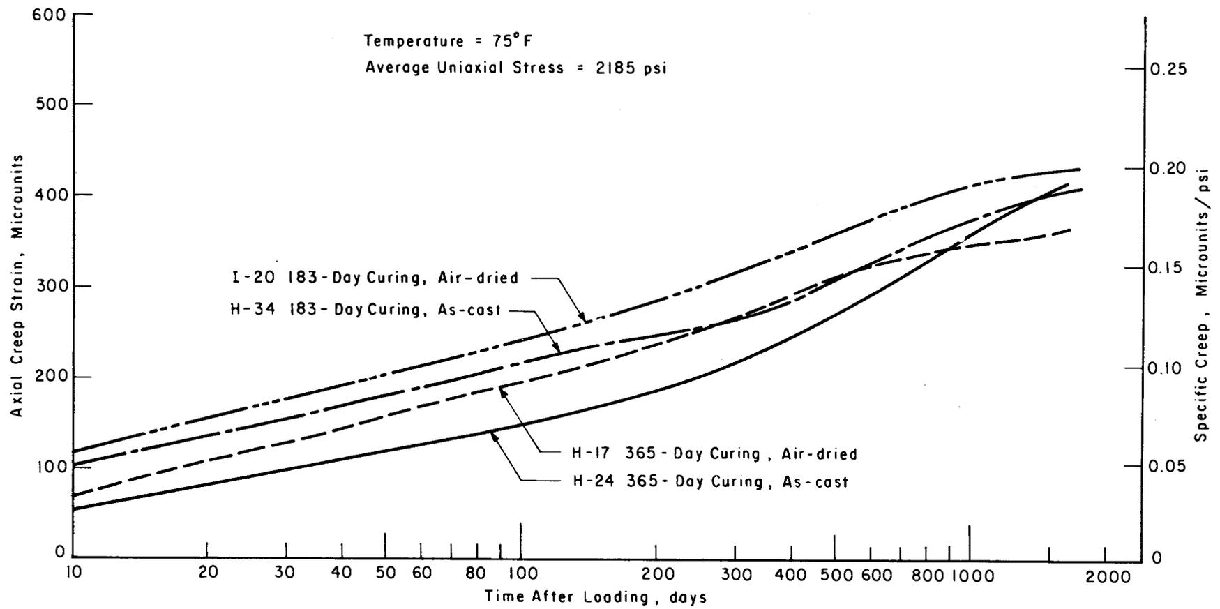
Fig 17. Relationship between axial creep strain and logarithm of time for specimens with uniaxial stress of 2400 psi.
