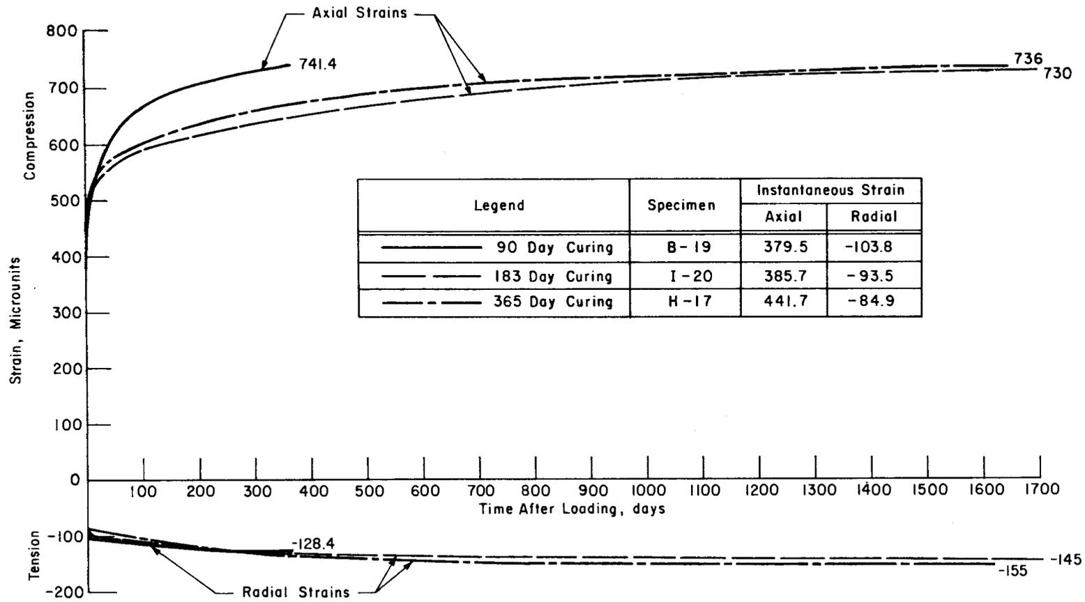
Fig 8. Total axial and radial strain relationships for air-dried specimens with uniaxial stress of 2400 psi.
