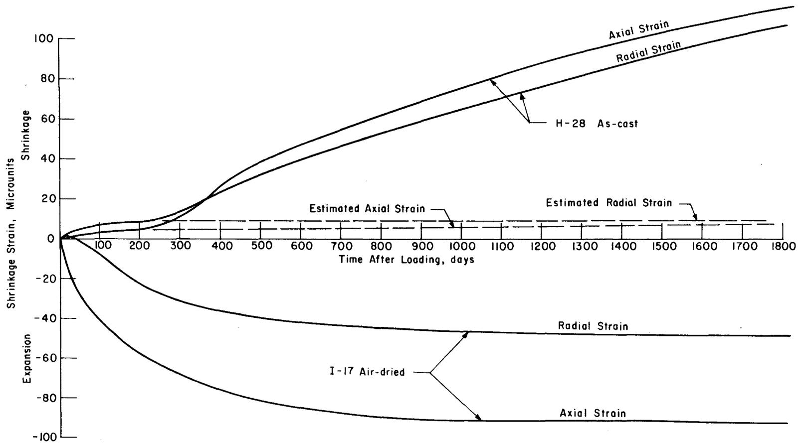
Fig 11. Shrinkage strains during the loaded periods for creep specimens cured 183 days.
