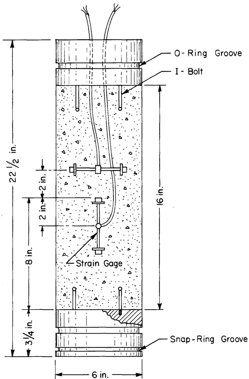
Fig 3. Test specimen and gage locations.
