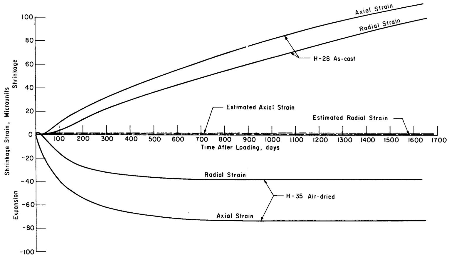
Fig 12. Shrinkage strains during the loaded periods for creep specimens cured 365 days.
