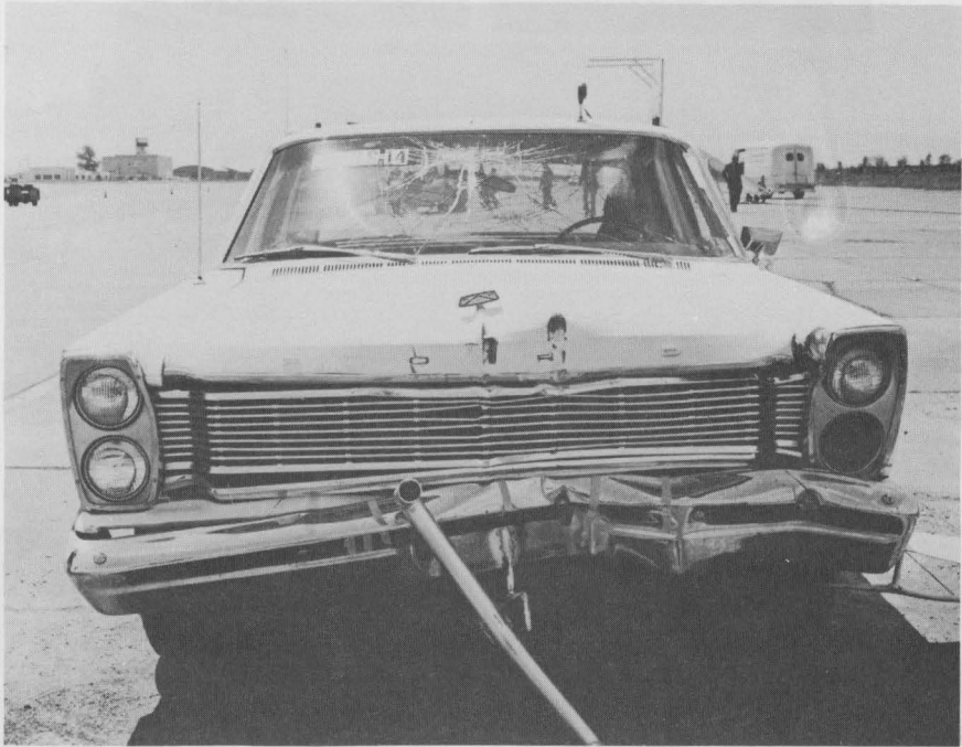
Figure 27. Vehicle after Tests S-14. Windshield was cracked in Test S-12.
