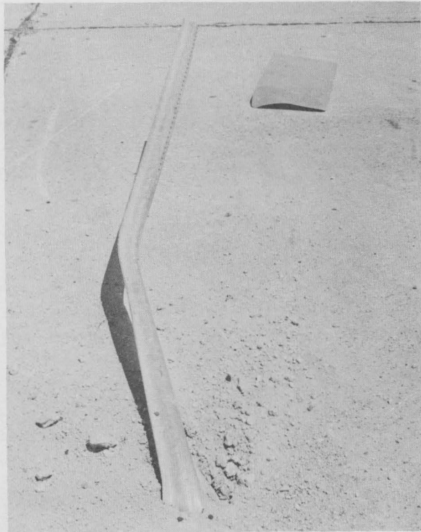
Figure 19. "Before" and "After" photographs of Texas Mile Post Marker mounted on delineator post driven into soil. Test S-15, 28.1 mph, \Delta V = 0.5 mph.
