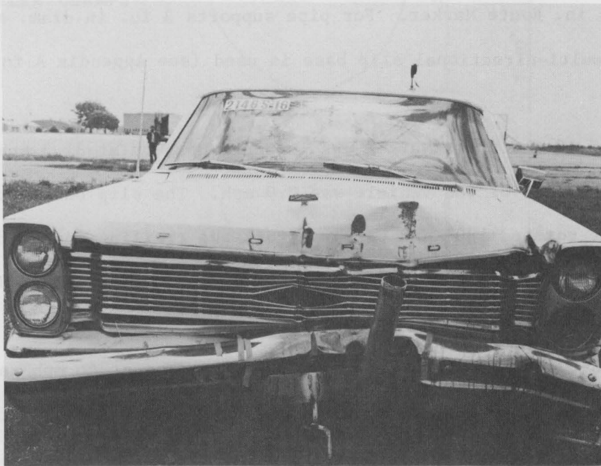
Figure 31. Vehicle after Test S-16. Windshield was cracked in Test S-12.
