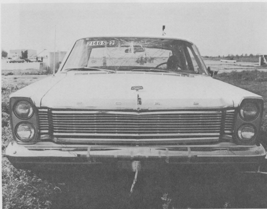
Figure 10. Vehicle after Test S-12. (Note cracked windshield) 56.9 mph, \Delta V = 0.9 mph.
