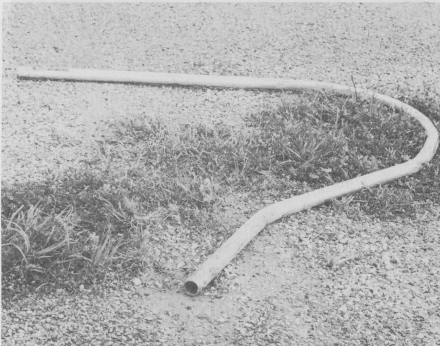
Figure 16. "Before" and "After" photographs of Mile Post Marker mounted on 1.25" pipe driven into soil. Test S-4, 59.4 mph, \Delta V = 0.5 mph.
