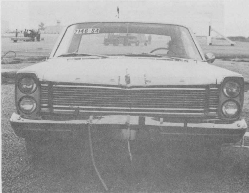
Figure 17. Vehicle after Test S-4, 59.4 mph, \Delta V = 0.5 mph.
