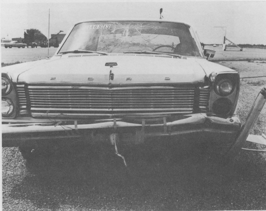
Figure 29.. Vehicle after Test S-13. Windshield was cracked in Test S-12.
