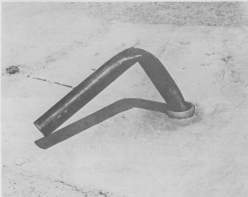
Figure 4. 2" pipe post and 1.5" pipe insert after crash. Test S-7, 47.5 mph, \Delta V = 2.6 mph.
