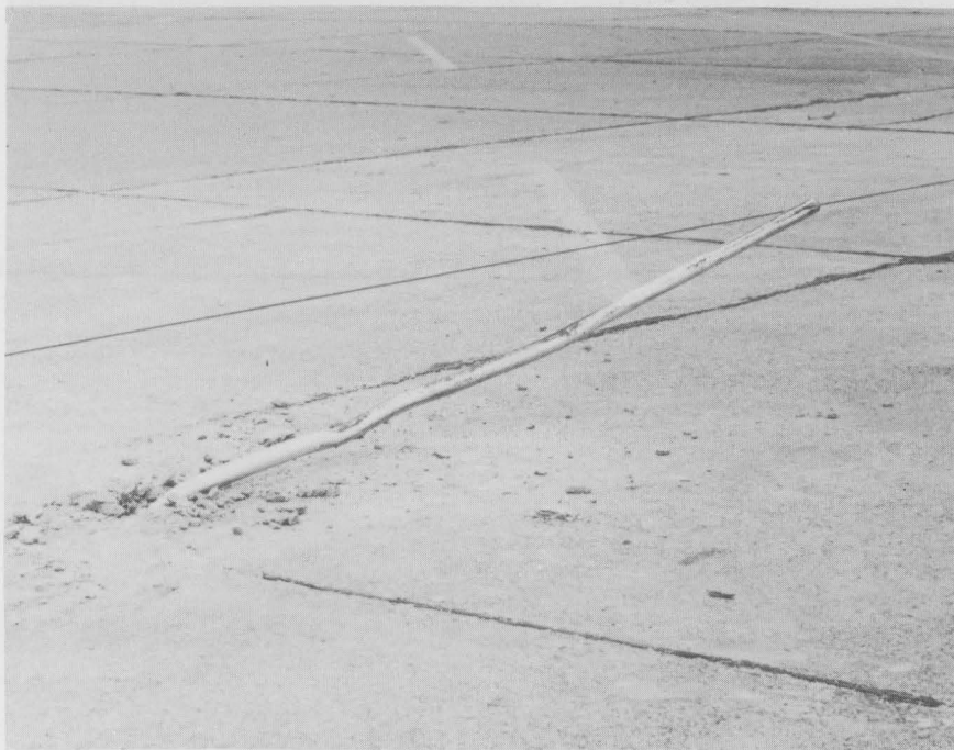
Figure 12. "Before" and "After" photographs of Mile Post Marker mounted on 1.25" pipe driven into soil. Test S-3, 31 mph, \Delta V = 1.4 mph.
