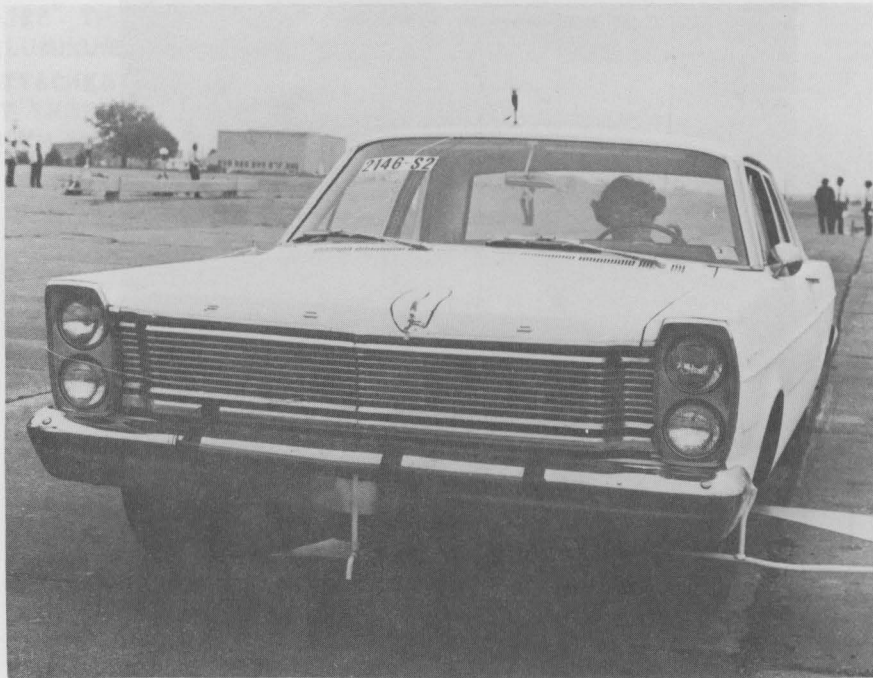
Figure 8. Vehicle after Test S-2, 38.2 mph, \Delta V = 1.3 mph.
