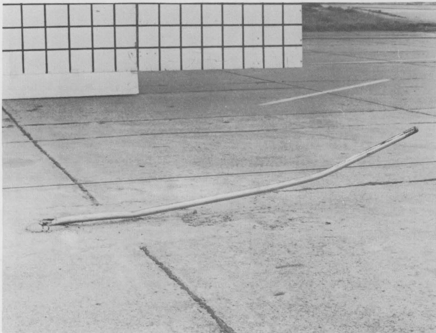
Figure 7. "Before" and "After" photographs of Mile Post Marker mounted on 1.25" pipe embedded in 8" diam. concrete shaft. Test S-2, 38.2 mph, \Delta V \approx 1.3 mph.
