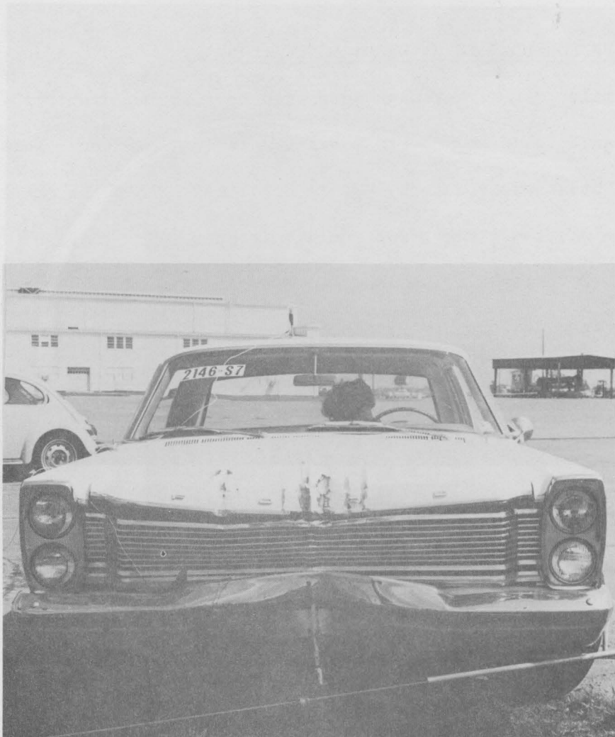
Figure 5. Vehicle after Test S-7, 47.5 mph, \Delta V = 2.6 mph.
