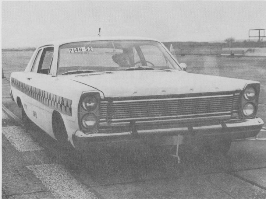
Figure B1. This vehicle was used in Tests S-2 through S-11. 1965 Ford sedan, weight 3970 lb.
