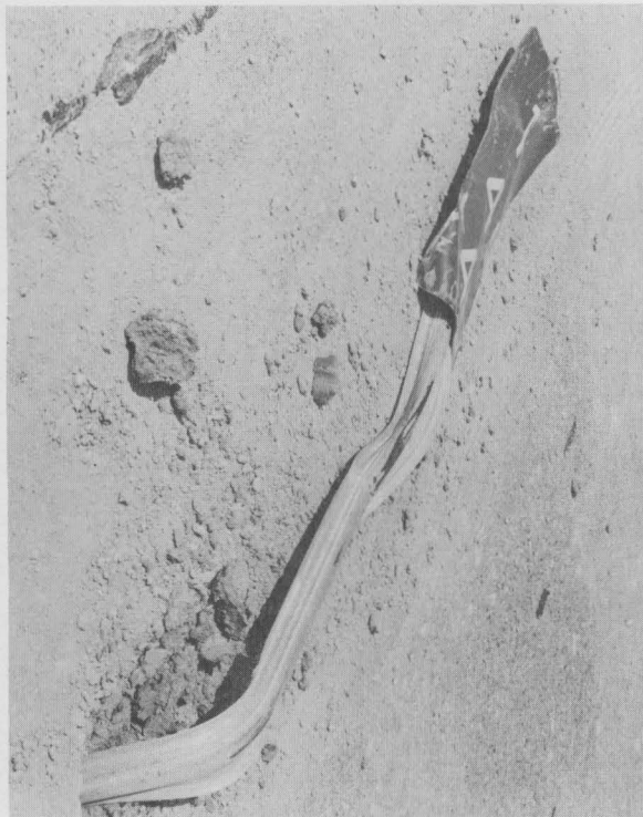
Figure 20. "Before" and "After" photographs of Texas Mile Marker mounted on delineator post driven into soil. Test S-9, 45.2 mph, \Delta V = 0.9 mph.
