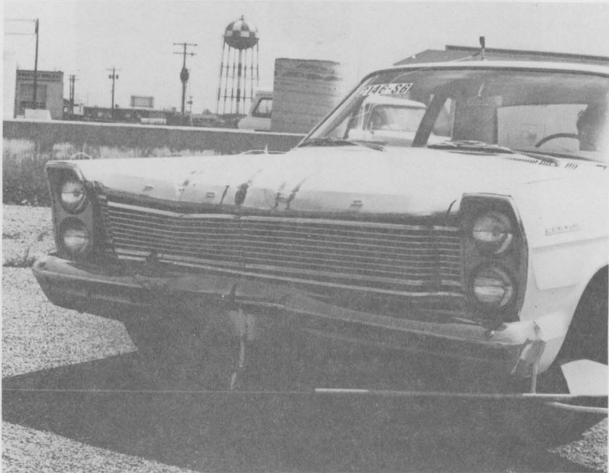
Figure 22. Vehicle after Test S-6, 61.3 mph, \Delta = 0.9 mph.
