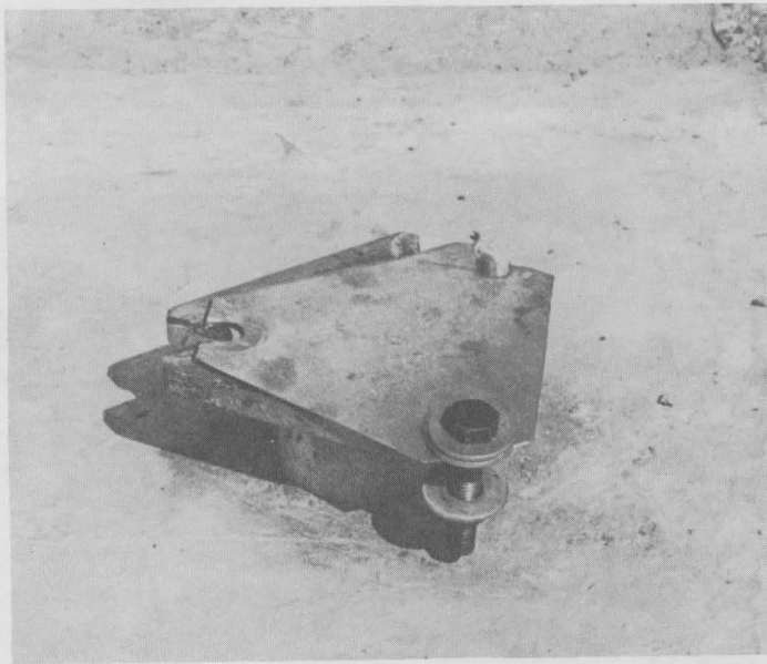
Figure 35. Route Marker and base after crash. Test S-8, 46 mph, \Delta V = 0.8 mph.
