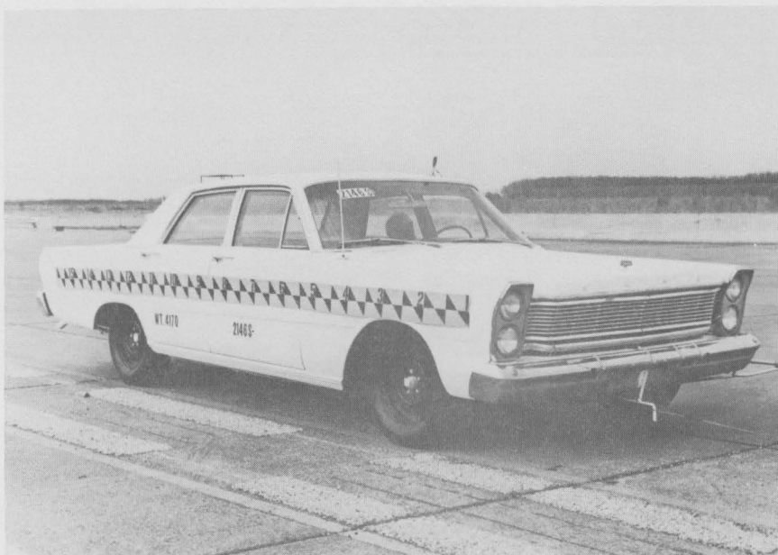
Figure B3. This vehicle was used in Tests S-12 through S-18. 1965 Ford sedan, weight 4170 lb.
