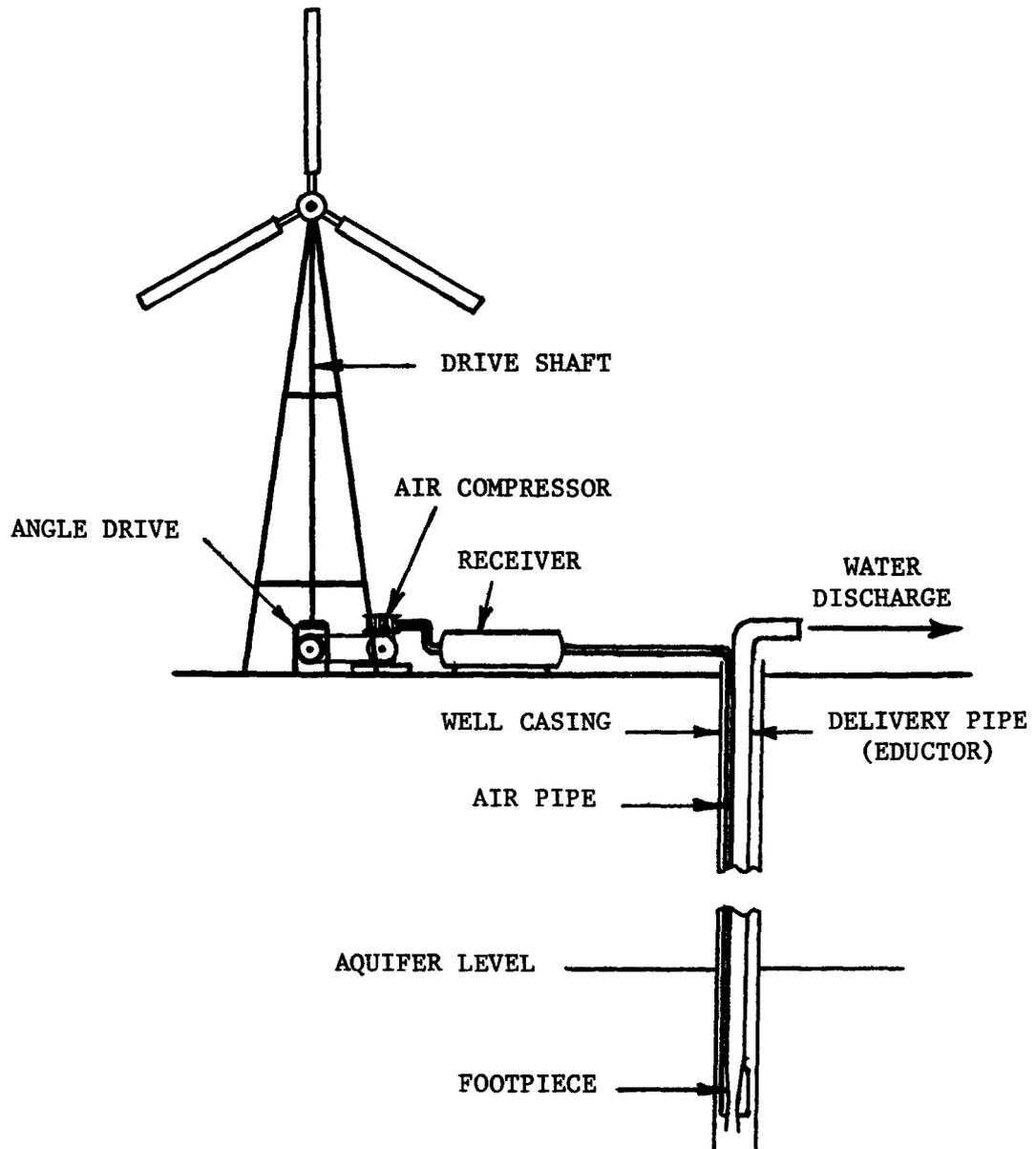
FIGURE 16: AIRLIFT PUMPING SYSTEM. ROTOR DIAMETER = 33 FT,
