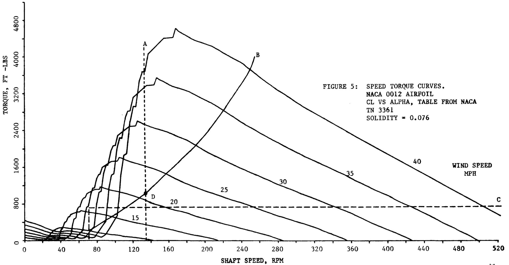
1. Constant RPM.  $C_p$  is a maximum at point D (the design point) in Figure 5 and  $C_p$  decreases (Figure 3) along the dotted line A on either side of point D. The load can vary only by means of torque changes and the problem is to determine the maximum size of load to provide for the most cost-efficient system. For example, if the load was held constant at D (23 kw) then the pitch of the blades would have to be changed to hold that constant load for all wind speeds above that point.
