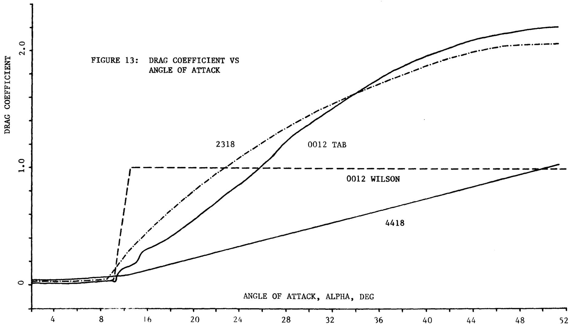
The 0012 Tabular airfoil is an adequate airfoil for the computer model of an optimum rotor. Probably a number of airfoils would give satisfactory performance, but until more experimental data are available (13), a decision on which type of airfoil to use involving 2 to 5 percent differences in overall efficiency will be difficult to make from computer models.
