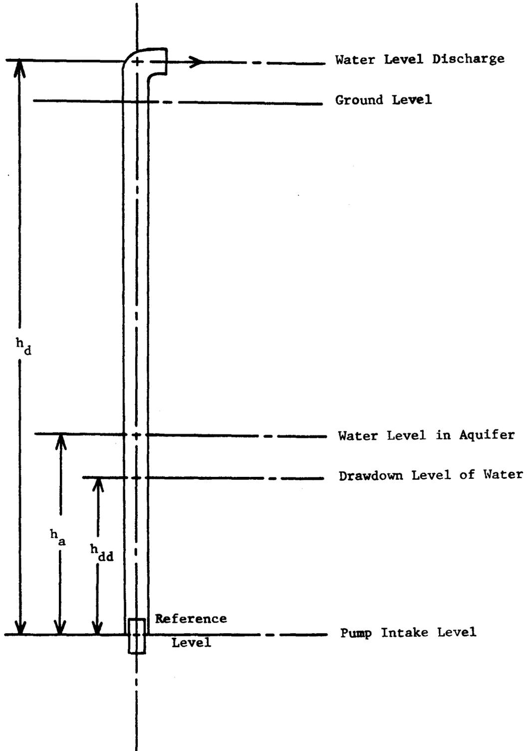
FIGURE 14: REFERENCE FRAME FOR ANALYSIS OF PUMPING SYSTEMS
