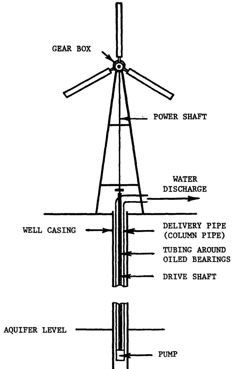
FIGURE 15. ROTARY POSITIVE DISPLACEMENT PUMPING SYSTEM. ROTOR DIAMETER = 33 FT, TOWER HEIGHT = 40 FT.
