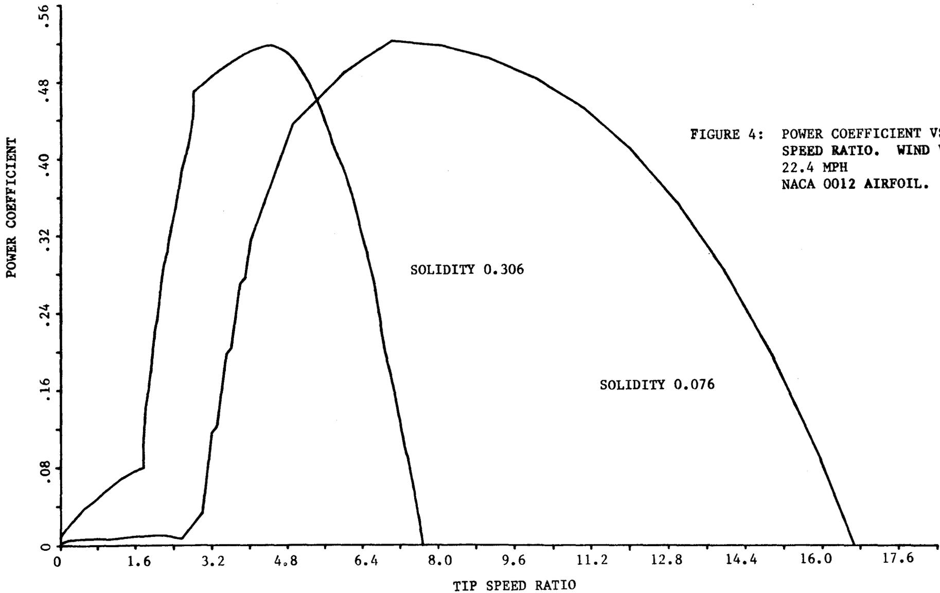
FIGURE 4: POWER COEFFICIENT VS TIP SPEED RATIO. WIND VELOCITY = 22.4 MPH
