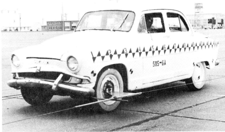
Figure 1, Vehicle Before Test 505-6A. 1959 Simca, Weight 2060 pounds. (Note Cable Guidance System and Stadia Board)
