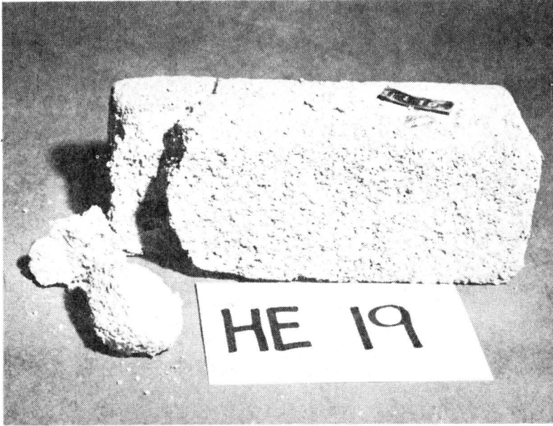
Figure C12 Condition of specimen HE1-19 after 24 cycles of freezing and thawing.
