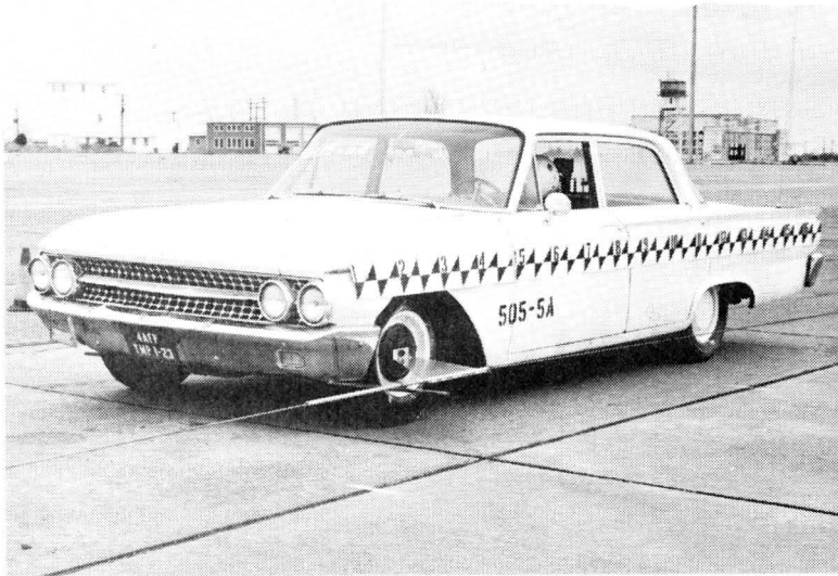
FIGURE 5. VEHICLE BEFORE COLLISION. 1961 FORD, WEIGHT 3880 LB.
