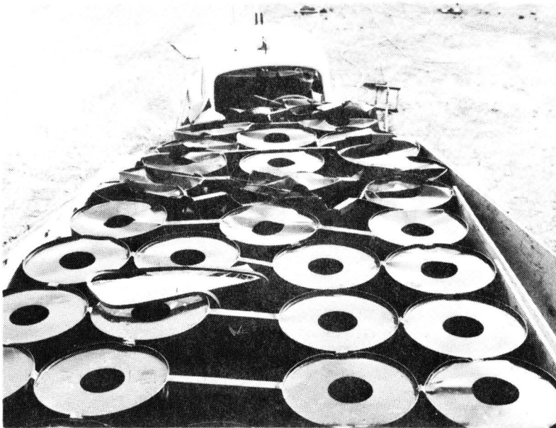
Figure 33, Modular Crash Cushion After Test 505 B-E.
