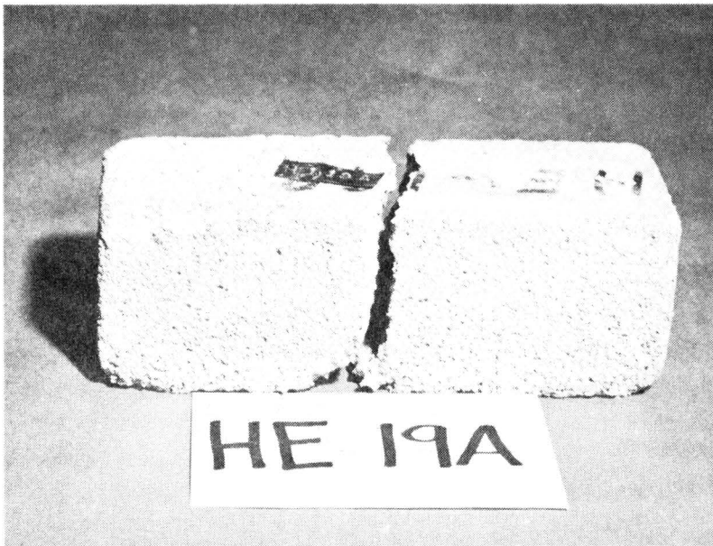
Figure C13 Condition of specimen HE1-19A after 24 cycles of freezing and thawing.
