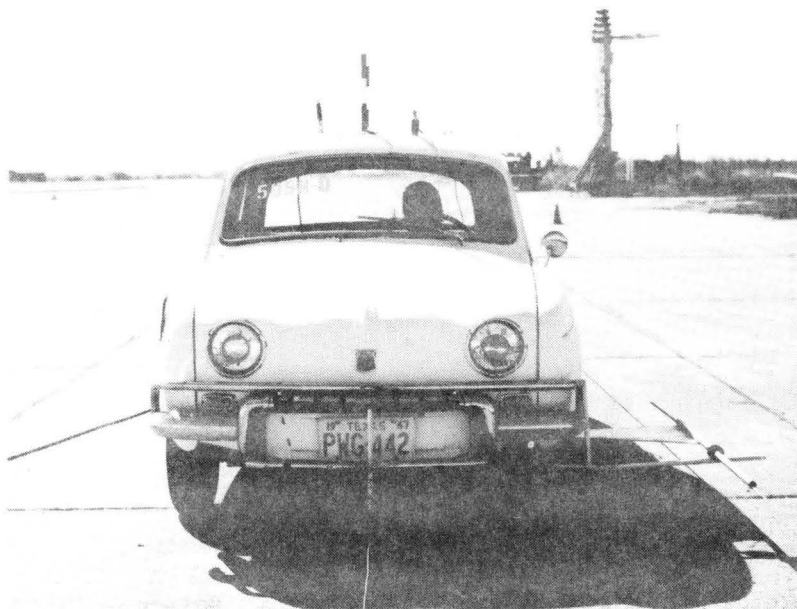
Figure 24, Front of Vehicle Showing Tow Cable (center) and Guidance Cable (right).
