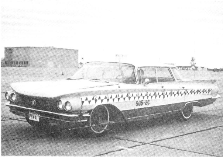
FIGURE 12. VEHICLE BEFORE COLLISION. TEST 2C, 1960 BUICK, WEIGHT 4940 LB.
