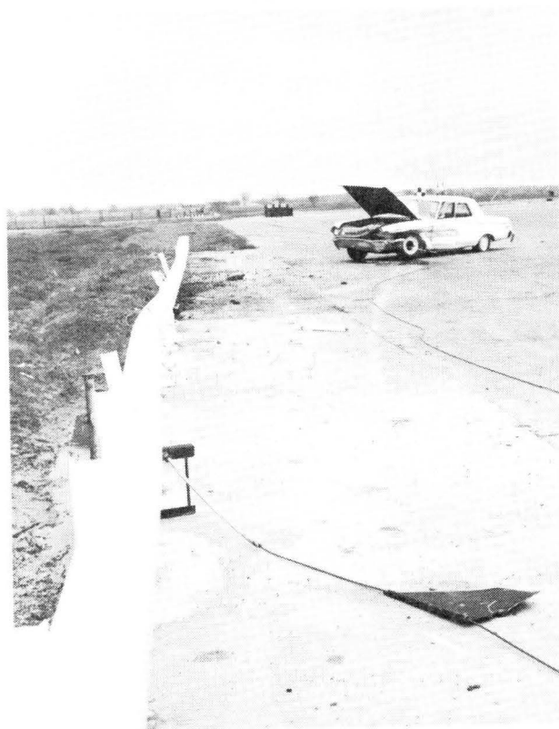
Figure 12, Deflection of Bridge Rail-Guardrail in Test NY-A.
