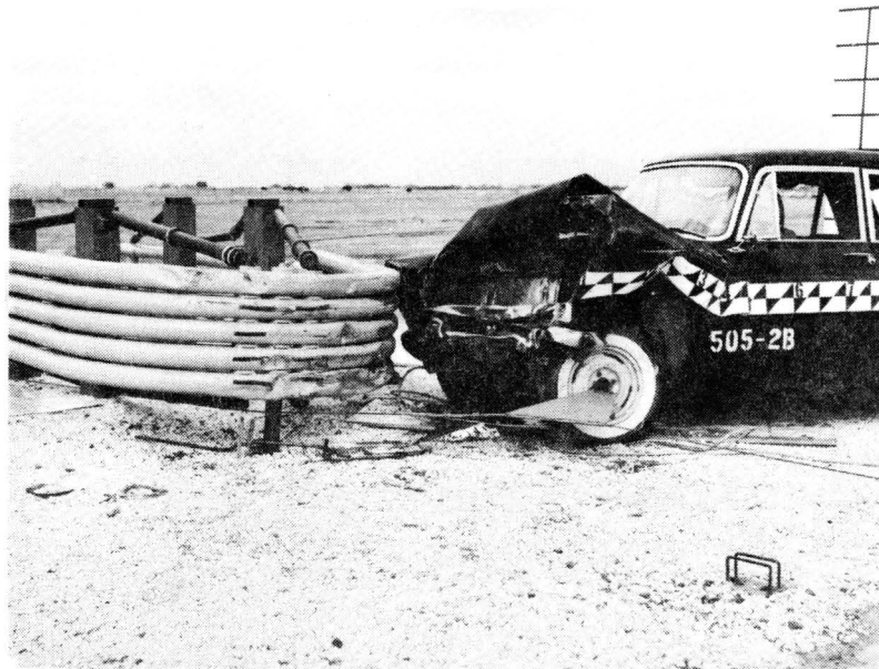
CONDITIONS AFTER TEST (VEHICLE STRUCK BARRIER HEAD-ON)
