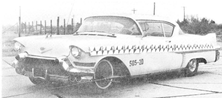
FIGURE 17. VEHICLE BEFORE COLLISION. TEST 2D. 1957 CAD., WEIGHT 5000 LB.
