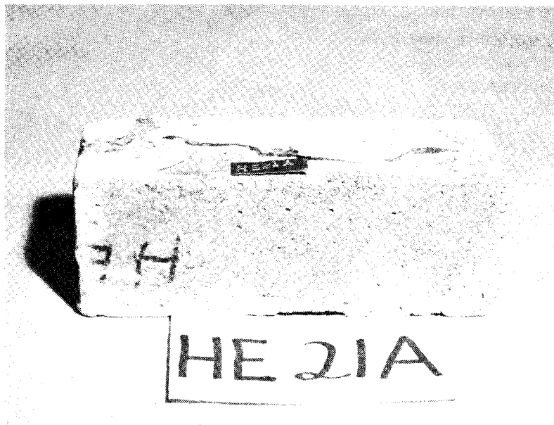
Figure C17 Condition of specimen HE1-21A after 16 cycles of freezing and thawing.
