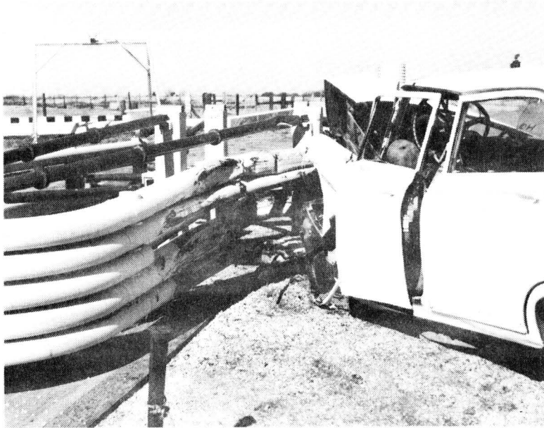
Figure S-8, Damage To Left Front Of Vehicle
