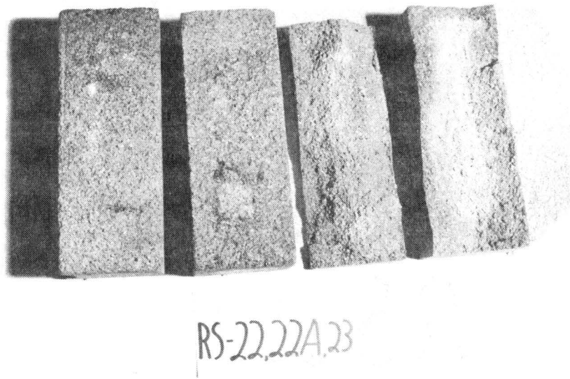
Figure C7 Conditions of specimens RS-22, 22A after 27 cycles, and RS-23 after 4 cycles of freezing and thawing.
