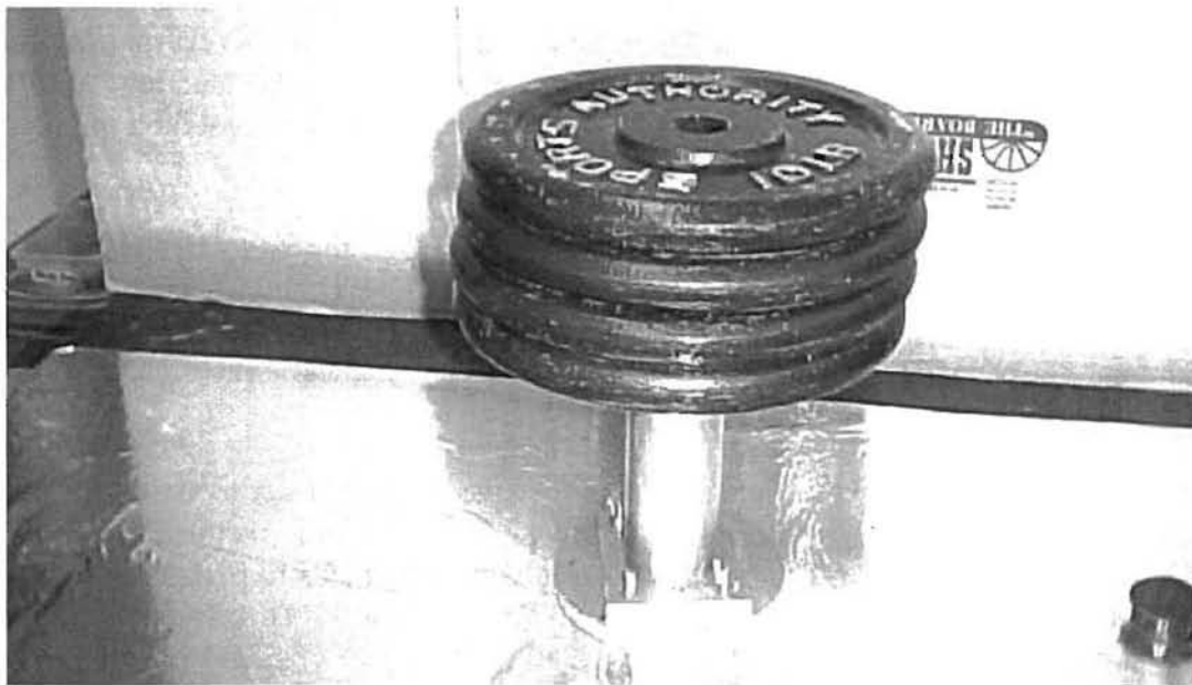
Figure 6.13 - Loading Arrangement for Simple Pull-Off Test
