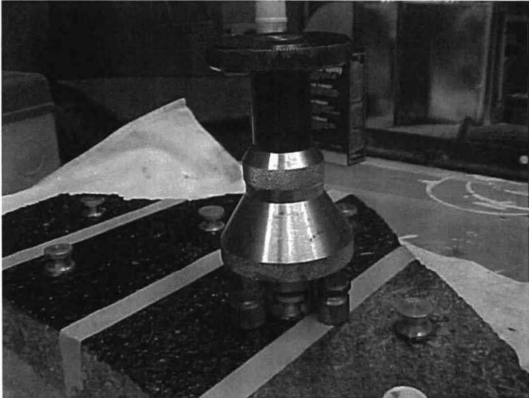
Figure 3.5 - Test Performed using ELCOMETER106
