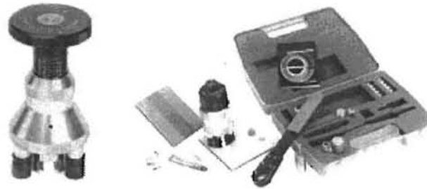
Figure 2.28 - Elcometer106 Mechanical Adhesion Tester
