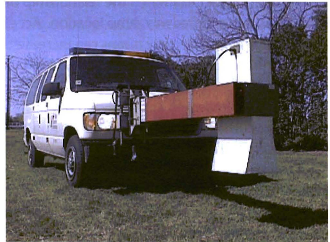
GPR mounted on the front of a vehicle
