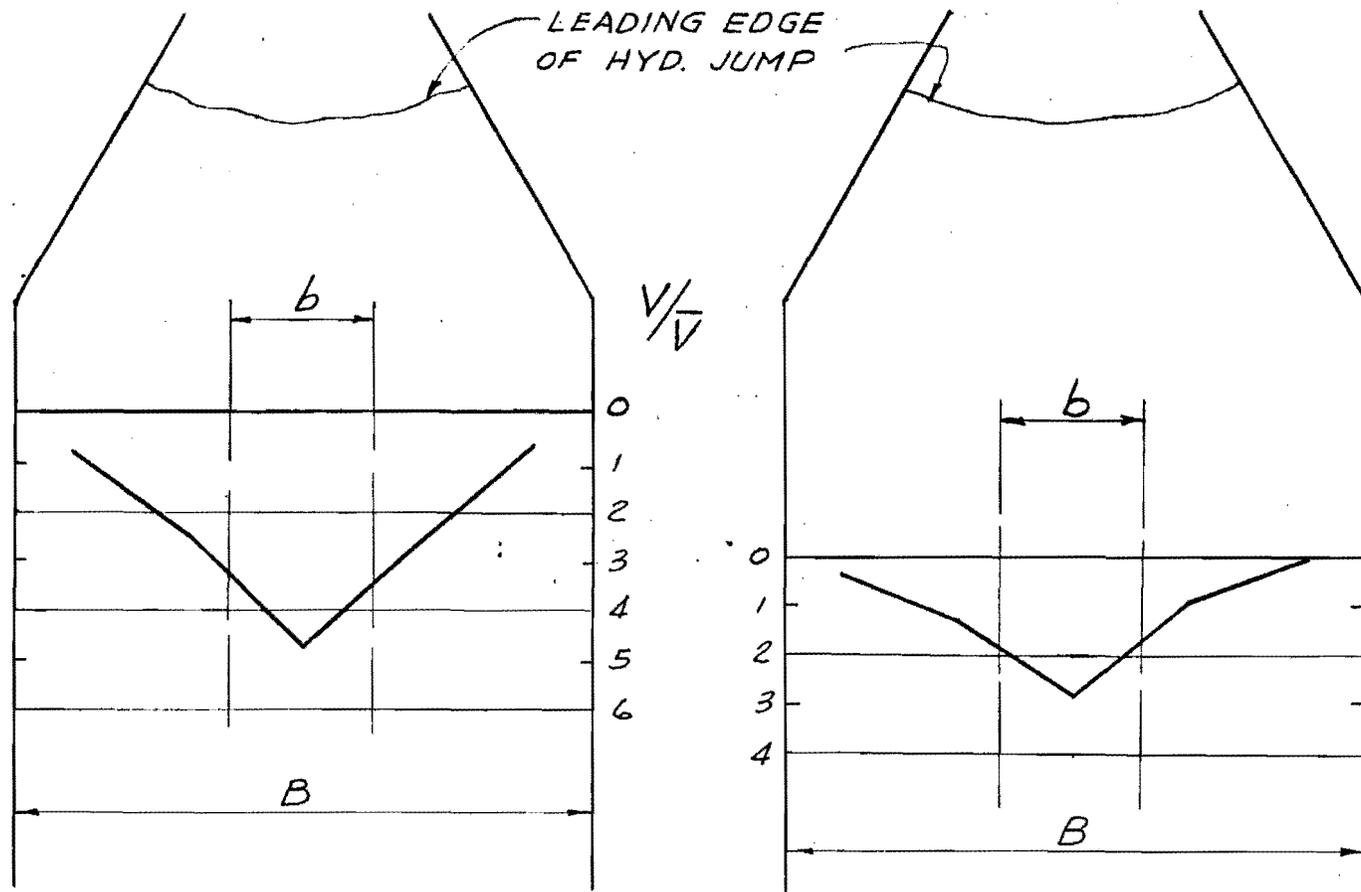
FIGURE 5 VELOCITY VARIATION ACROSS CHANNEL WIDTH
