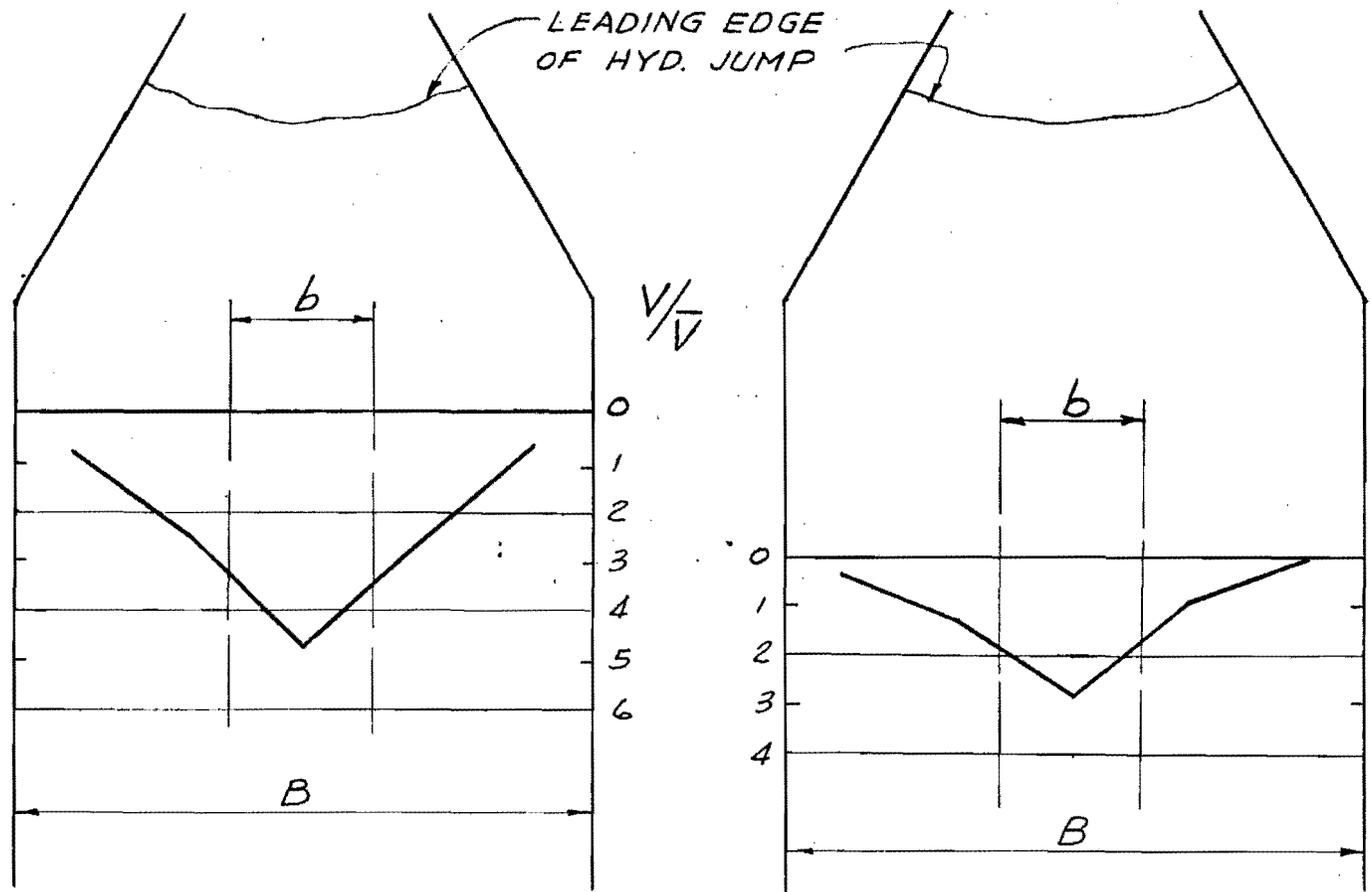
FIGURE 5 VELOCITY VARIATION ACROSS CHANNEL WIDTH
