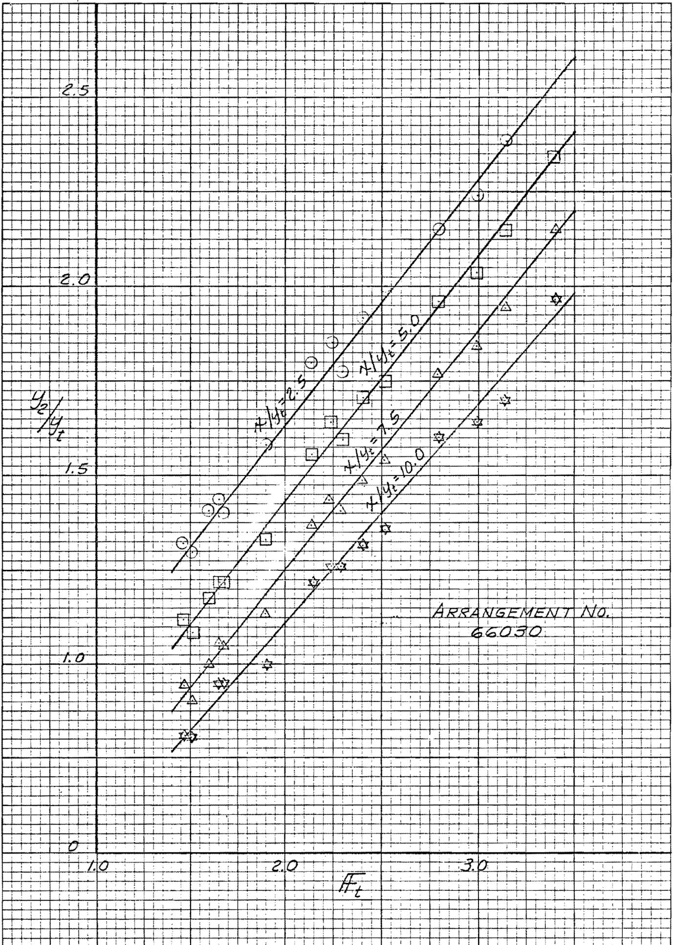
FIGURE 4 STABILITY OF HYDRAULIC JUMP IN RADIAL-FLOW STILLING BASIN
