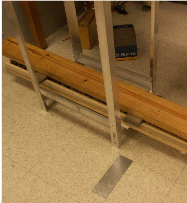
Figure 4-6 wood plank is raised up 1 mm for each measurement by inserting metal sheets
