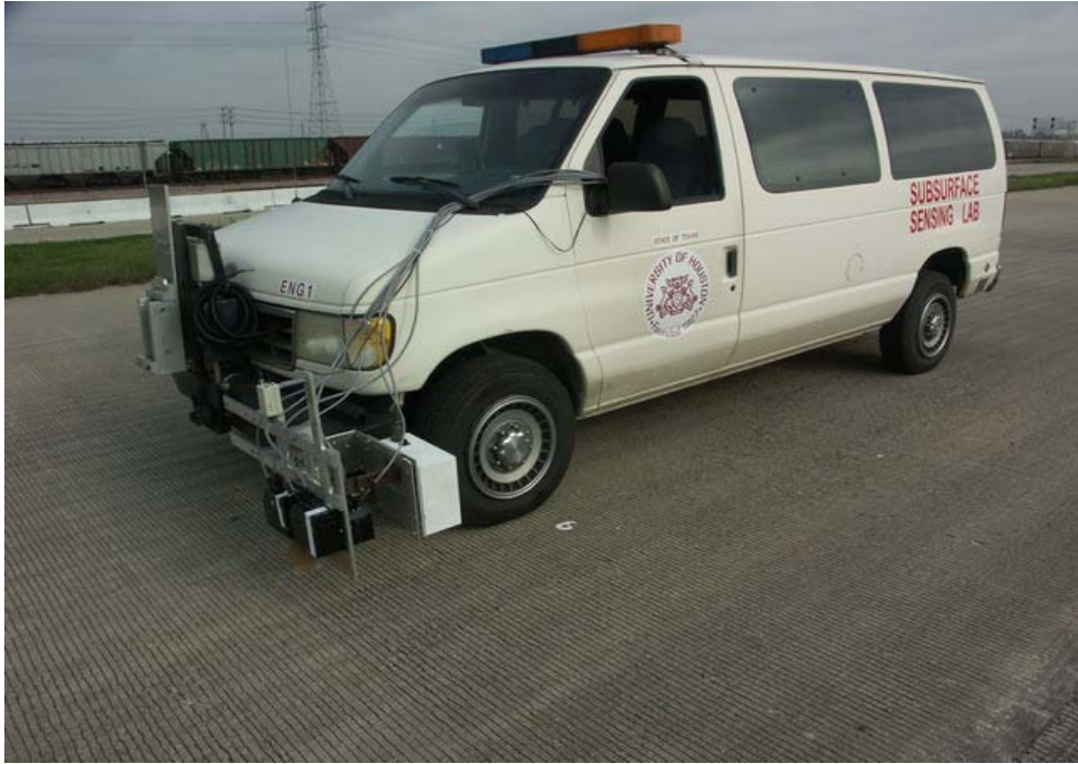
Figure 2-6 Vehicle-mounted laser measuring devices developed by University of Houston
