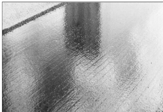
Figure 1-2 Too much aggregate (no binder is visible)
