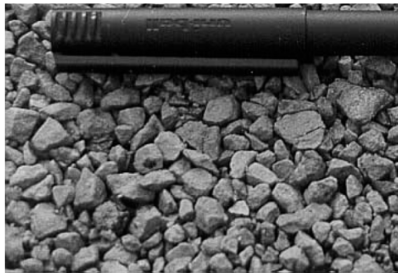
Figure 1-2 Too much aggregate (no binder is visible)
