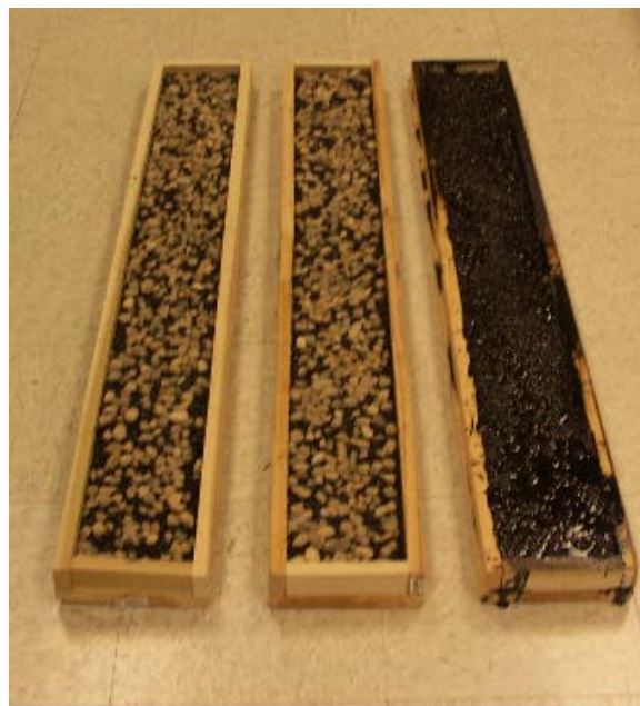
Figure 4-2 Test samples of bare, medium, and flushed asphalt slabs
